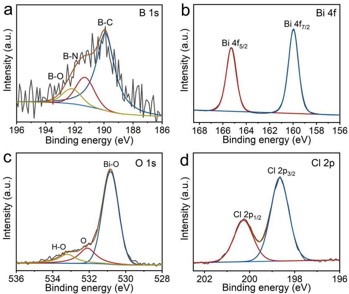
**Fig. S5.** (a) High-resolution XPS spectra of B 1s for BiOCl@N-CNTs, and (b) Bi 4f, (c) O 1s, and (d) Cl 2p for BiOCl@C.
