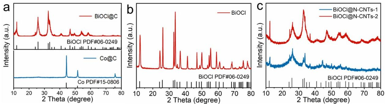
**Fig. S4.** XRD patterns of synthesized (a) Co@C and BiOCl@C, (b) BiOCl, and (c) BiOCl@N-CNTs-1 and BiOCl@N-CNTs-2.
