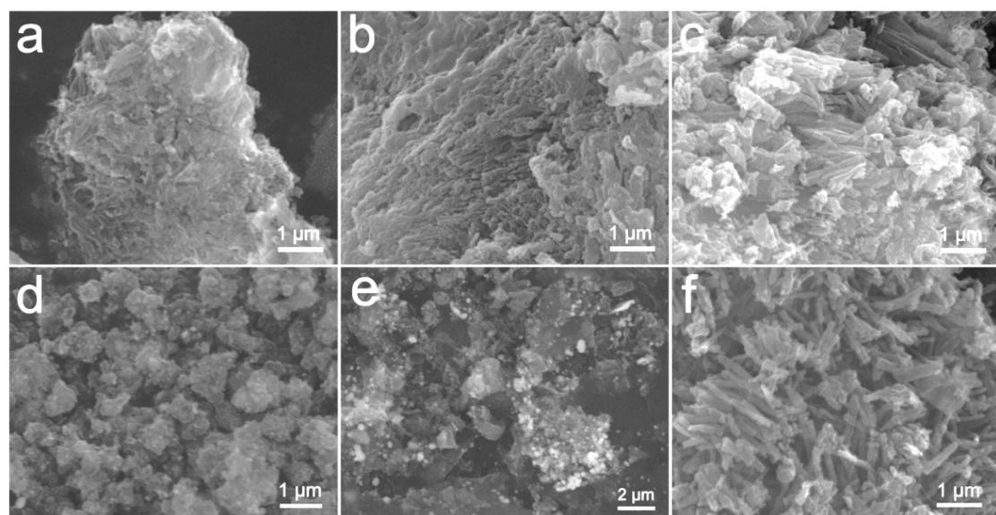
**Fig. S2.** SEM images of (a) Co@N-CNTs-750, (b) Co@N-CNTs-800, (c) Co@N-CNTs-850, (d) Co@NC, (e) Co@BC, and (f) N-CNTs, respectively.
