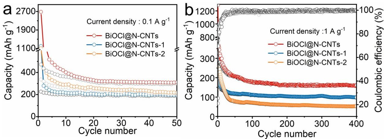
**Fig. S10.** (a) Cycling performance at  $0.1 \text{ A g}^{-1}$ , and (b) Long-term cycling performance at  $1.0 \text{ A g}^{-1}$  of BiOCl@N-CNTs, BiOCl@N-CNTs-1 and BiOCl@N-CNTs-2.
