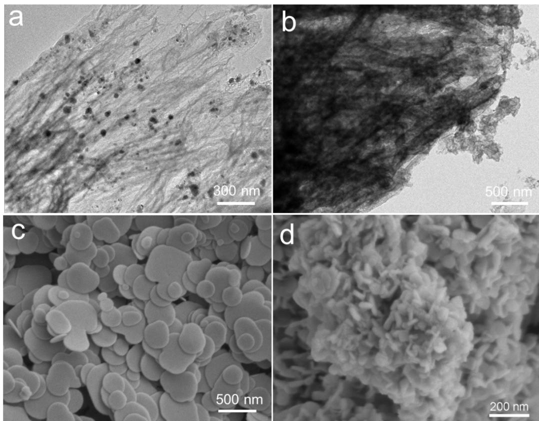
**Fig. S3.** TEM images of (a) BiOCl@N-CNTs-1 and (b) BiOCl@N-CNTs-2. SEM images of (c) BiOCl, and (d) BiOCl@C.
