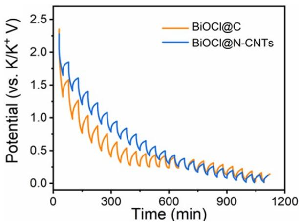
**Fig. S13.** GITT profiles of the BiOCl@C and BiOCl@N-CNTs during the discharge process after 20 cycles.
