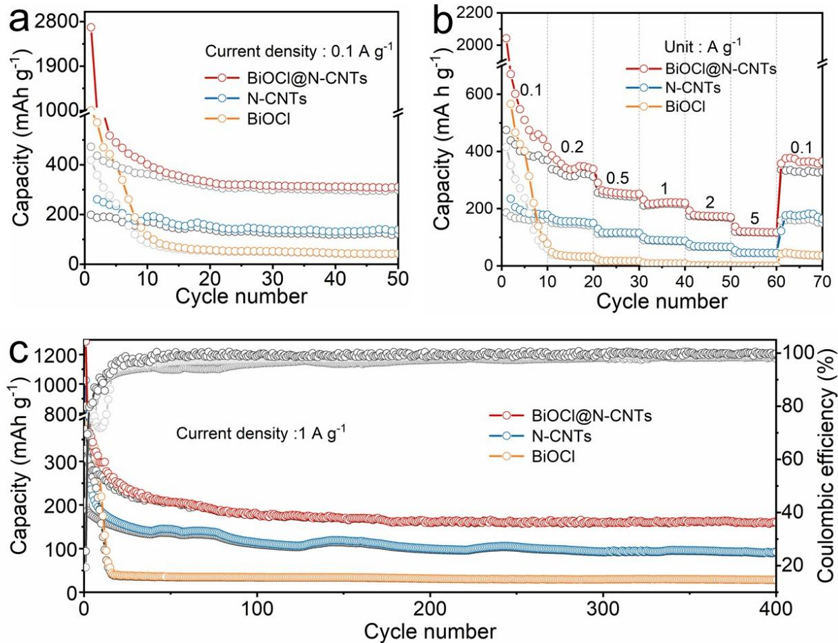
**Fig. S9.** (a) Cycling performance at  $0.1 \text{ A g}^{-1}$ , (b) Rate capability, and (c) Long-term cycling performance at  $1.0 \text{ A g}^{-1}$  of BiOCl@N-CNTs, BiOCl and N-CNTs.
