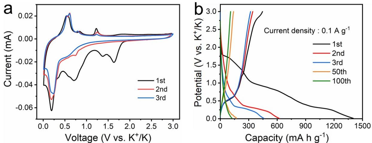
**Fig. S8.** (a) CV curves of the BiOCl@C at a scan rate of 0.1 mV s<sup>-1</sup> within a voltage range of 0.01–3.0 V. (b) Discharge and charge profiles of the BiOCl@C at 0.1 A g<sup>-1</sup>.
