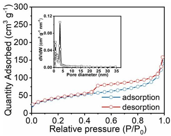
**Fig. S7.** Nitrogen adsorption-desorption isotherm of BiOCl@C (the inset shows the pore size distributions).
