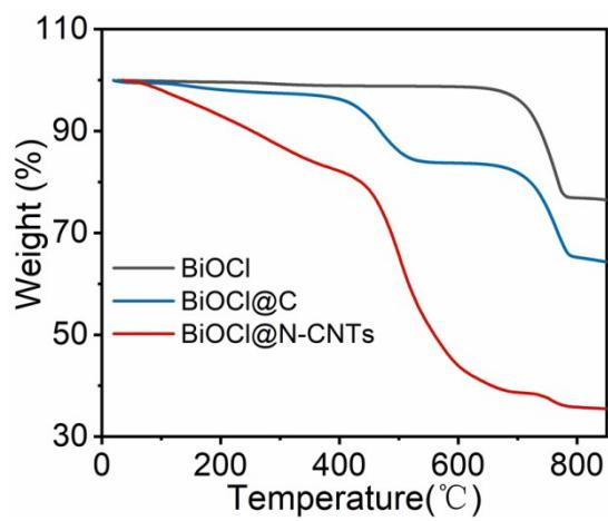
**Fig. S6.** TG curves of BiOCl, BiOCl@C and BiOCl@N-CNTs.
