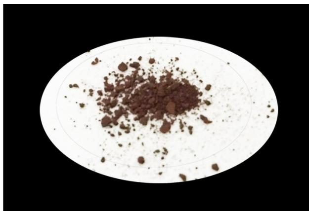
**Figure S4** Image of the initial InP/ZnSe powder. The sample was dark brown in color under daylight.
