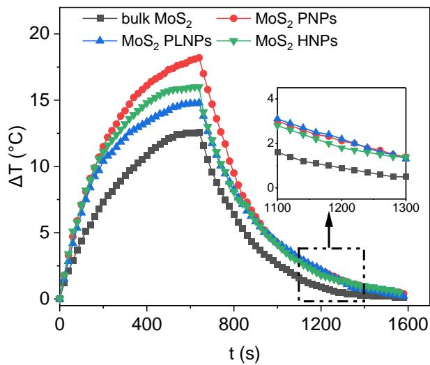
**Fig. S6** Temperature change *vs.* time of  $\text{MoS}_2$  particles with various morphologies when the laser on and off.
