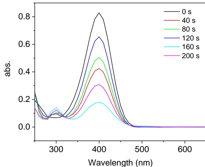
**Fig. S12** UV-vis absorption spectra of the reduction of 4-Nip with  $\text{MoS}_2$ -1.5 PNPs at 0.05 mg/ml and  $3 \text{ W/cm}^2$  within 200 s.
