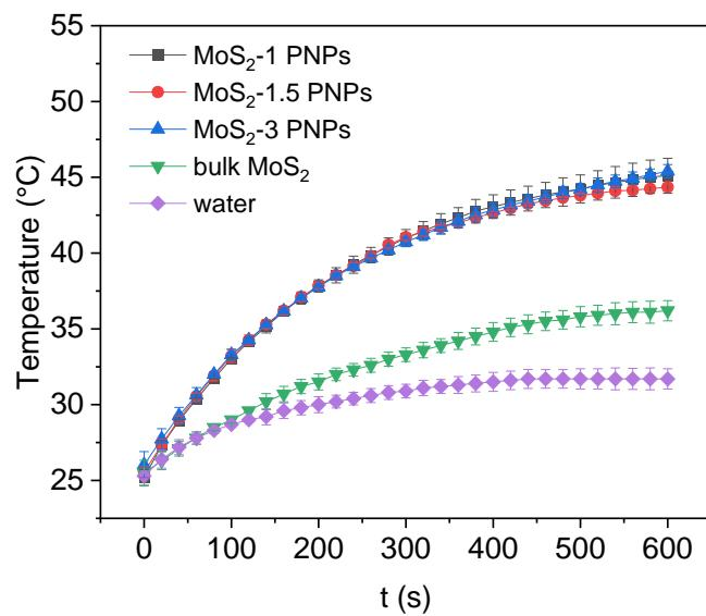
**Fig. S8** Temperature change of water and various MoS<sub>2</sub> PNPs at 0.1 mg/ml under NIR irradiation at 3 W/cm<sup>2</sup>.
