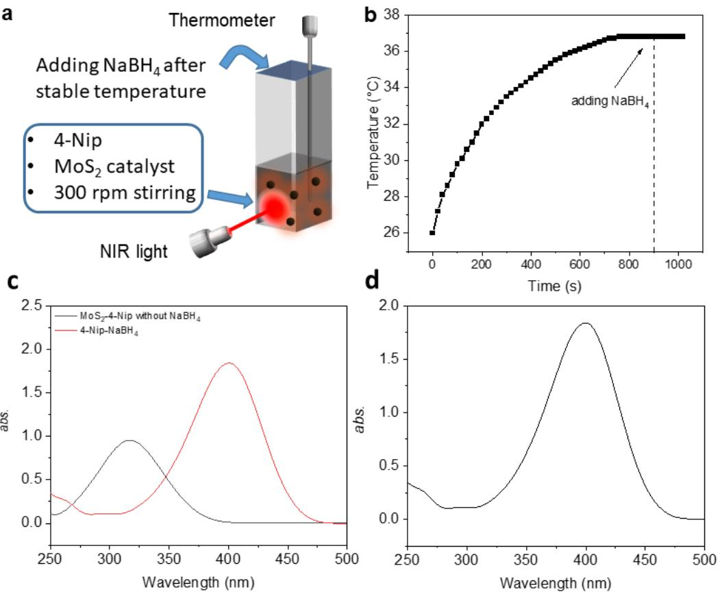
**Fig. S11** (a) Schematic illustration of the catalytic reduction reaction under NIR light irradiation at 0.05 mg/ml and  $3 \text{ W/cm}^2$ . (b) Photoheating curve of  $\text{MoS}_2$ -1.5 PNPs. UV-vis absorption spectra of the reaction solution (c) without  $\text{NaBH}_4$  or  $\text{MoS}_2$ -1.5 PNPs, and (d) when  $\text{NaBH}_4$  was replaced by  $\text{NaOH}$  (0.5 mM) after irradiation for 15 min.
