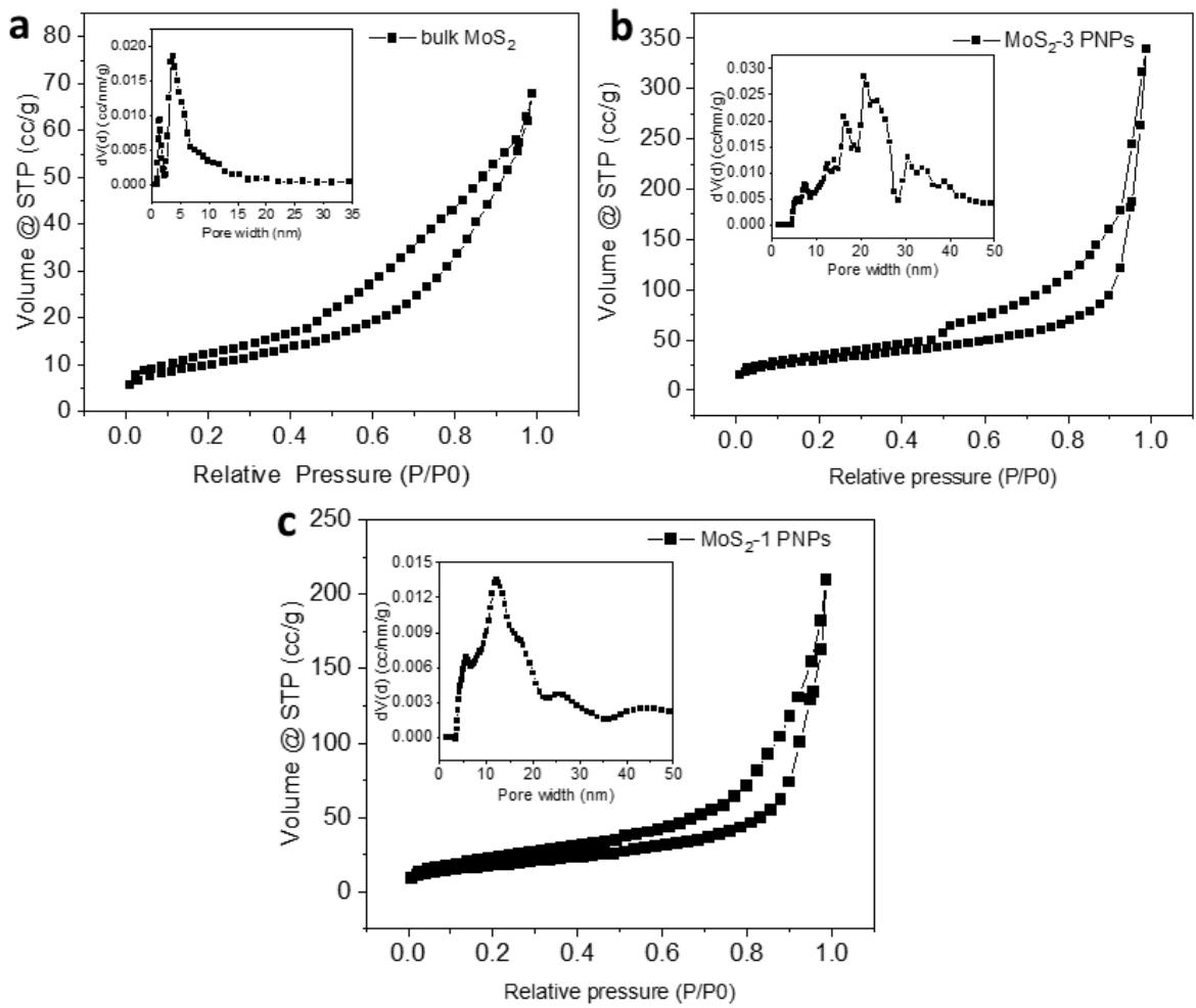
**Fig. S5** Isothermal  $\text{N}_2$  adsorption and desorption of various  $\text{MoS}_2$  particles. The insets are the corresponding curves of pore size distribution.
