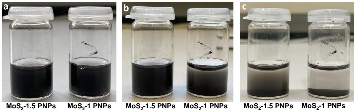
**Fig. S9** Photos of MoS<sub>2</sub> dispersions after storing for (a) 0 h, (b) 1.5 h and (c) 3h.
