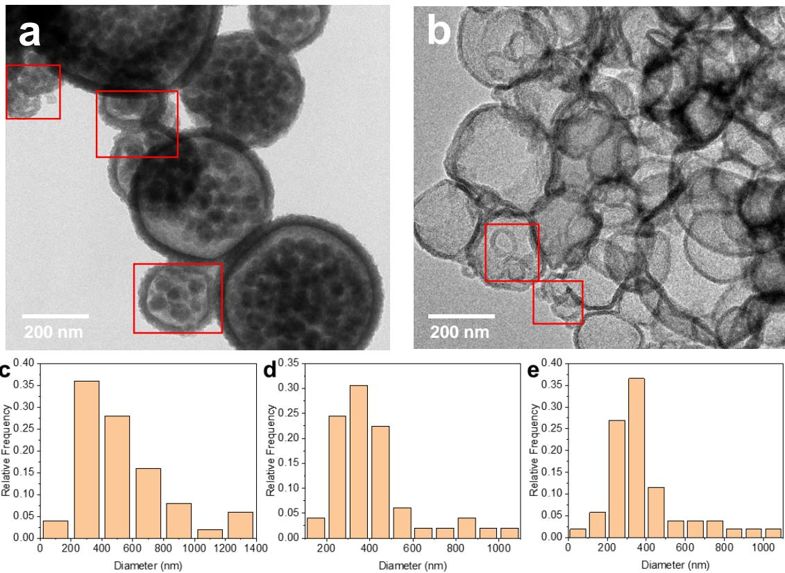
**Fig. S2** TEM images of (a) MoS<sub>2</sub> PLNPs and (b) MoS<sub>2</sub> HNPs. The histograms of particle size distribution of the MoS<sub>2</sub> PNNPs prepared at the precursor concentration of (c) 1, (d) 1.5 and (e) 3 mg/mL.
