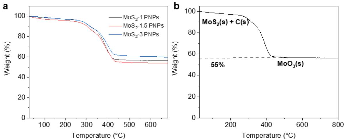
**Fig. S4** TGA curves of (a) various MoS<sub>2</sub> particles and (b) the chemical variation of the MoS<sub>2</sub>-1.5 PLNPs particles during calcination.
