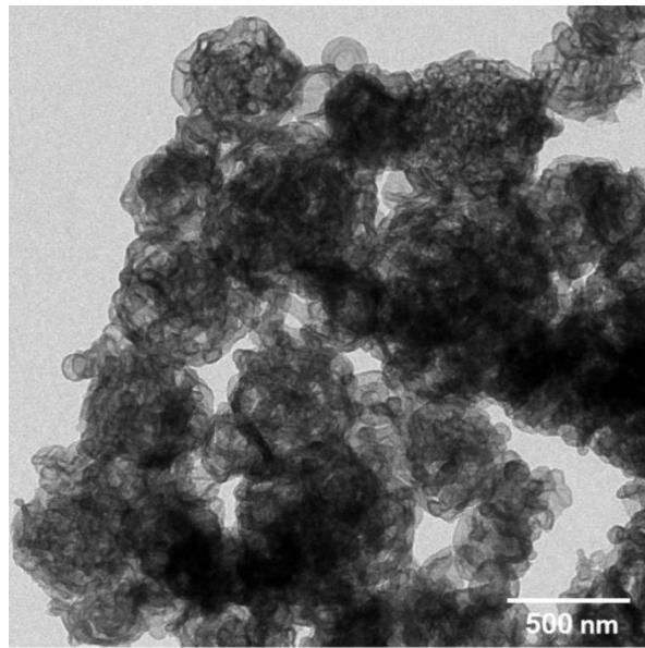
**Fig. S7** TEM image of the MoS<sub>2</sub>-1.5 PNPs after 5 photothermal test cycles.
