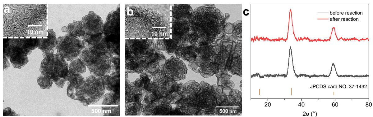
**Fig. S10** TEM image of the MoS<sub>2</sub>-1.5 PNPs (a) before and (b) after 5 catalytic cycles. (c) XRD patterns before and after catalytic reactions.
