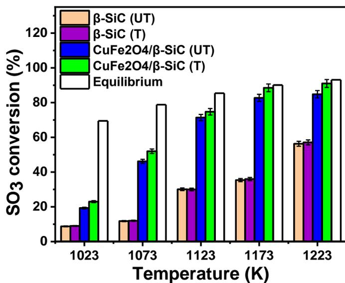
Figure S4 Comparison of SO<sub>3</sub> conversion (%) of β-SiC (UT) and β-SiC (T) with CuFe<sub>2</sub>O<sub>4</sub>/β-SiC (T) and CuFe<sub>2</sub>O<sub>4</sub>/β-SiC (UT) in the temperature range of 1023–1223 K.
