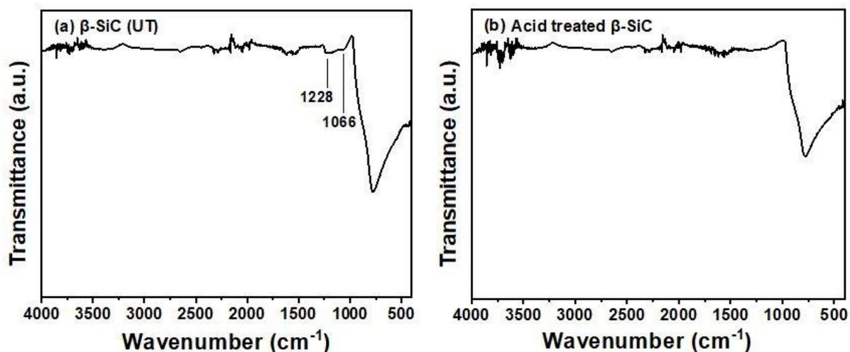
Figure S1 FTIR of (a)  $\beta$ -SiC (UT), and (b) acid treated  $\beta$ -SiC. Acid treatment leads to dissolution of  $\text{Si}_x\text{O}_y\text{C}_z/\text{SiO}_2$  phases and leaving SiC phase which is also evident from the absence of peaks at 1066 to 1164, 1228  $\text{cm}^{-1}$  in the FTIR spectra of acid treated  $\beta$ -SiC.
