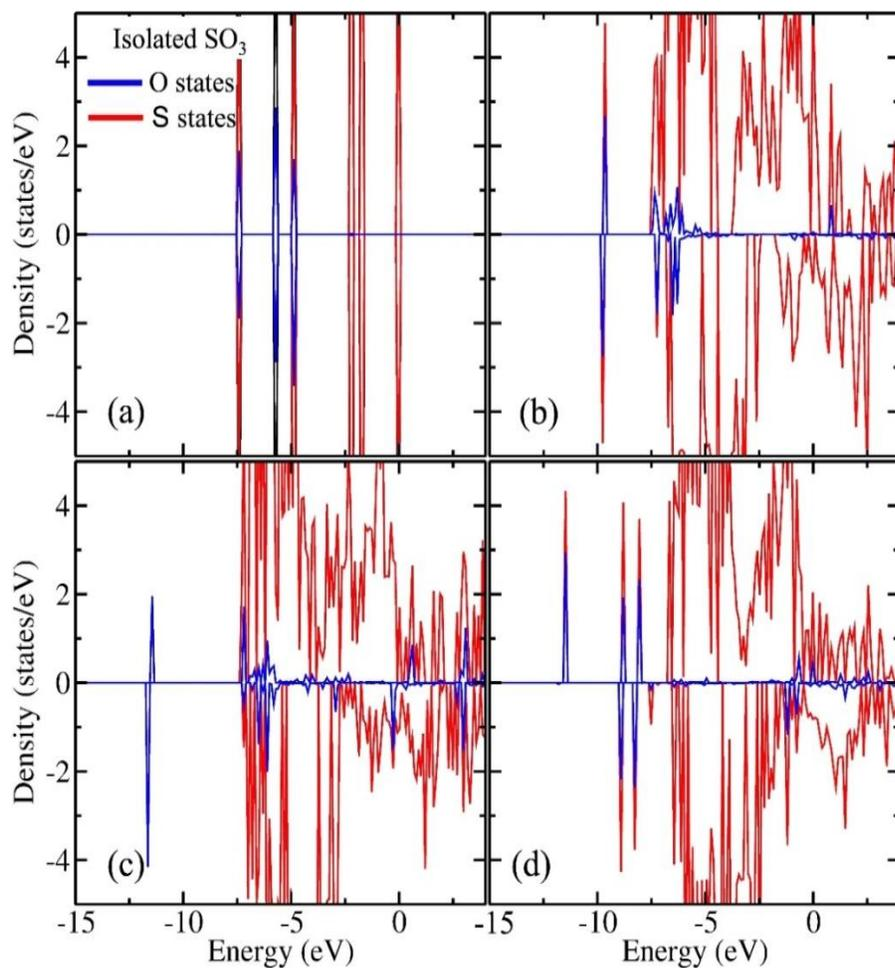
Figure S5 Partial density of states (pDOS) for (a) isolated SO<sub>3</sub>, SO<sub>3</sub> adsorbed over the cluster (b) CuFe<sub>2</sub>O<sub>4</sub>, (c) CuFe<sub>2</sub>O<sub>4</sub> with O-vacancy and (d) Fe<sub>2</sub>O<sub>3</sub> with O-vacancy. Here, blue and red colors correspond to S and O states, respectively.
