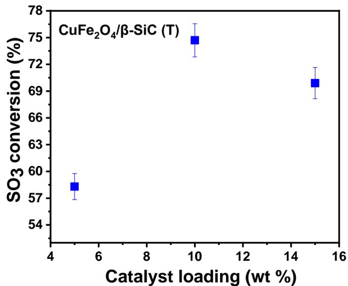
Figure S2 Effect of CuFe<sub>2</sub>O<sub>4</sub> loading over β-SiC (T) support.
