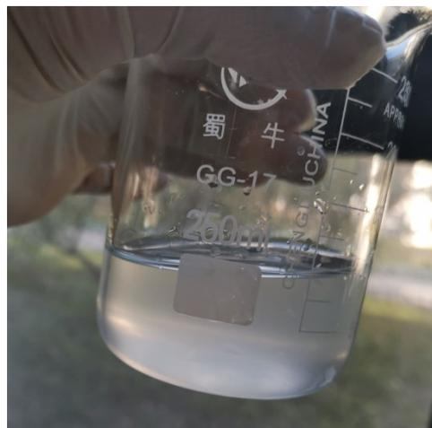
**Fig S2.** The uniform dispersion of SiO<sub>2</sub> nanoparticles within the buffer solution.
