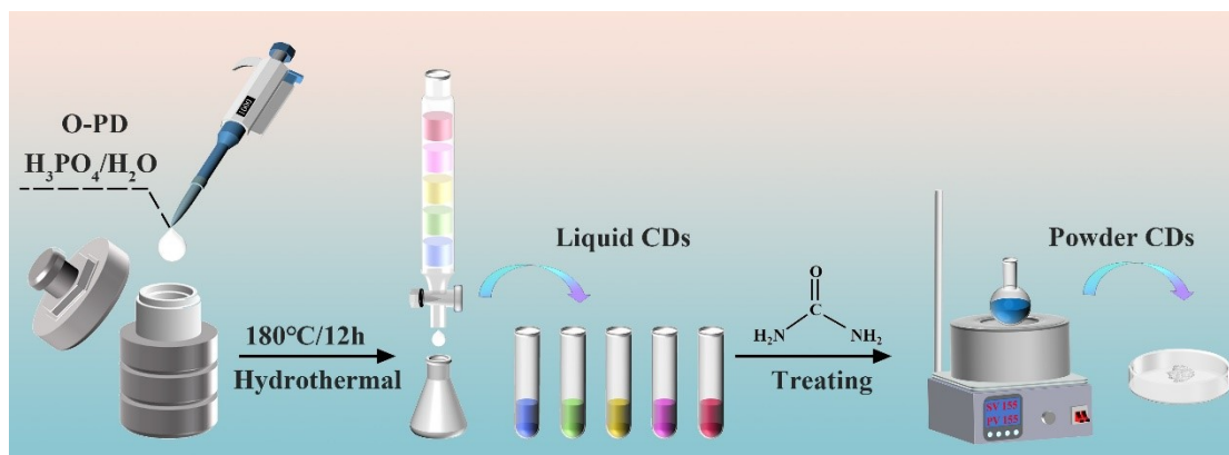
Fig. S1 The schematic diagram of the preparation of liquid CDs and powdered CDs.
