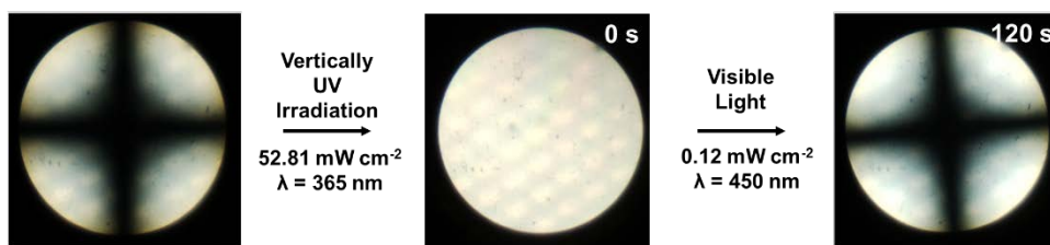
Fig. S12 Conoscopic images of LC command cell according to light source.
