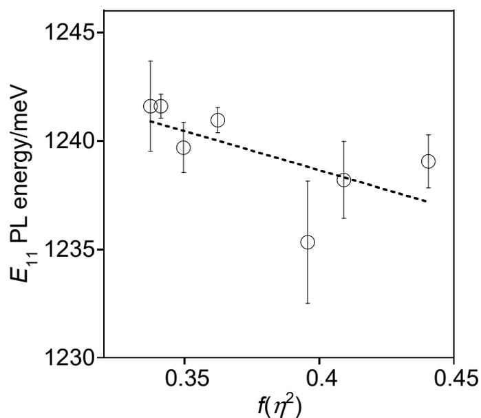
Fig. S4 Plot of the  $E_{11}$  PL energies against  $f(r^2)$ . The dotted line was obtained by the linear approximation method. Error bars are standard deviations of technical triplicates.
