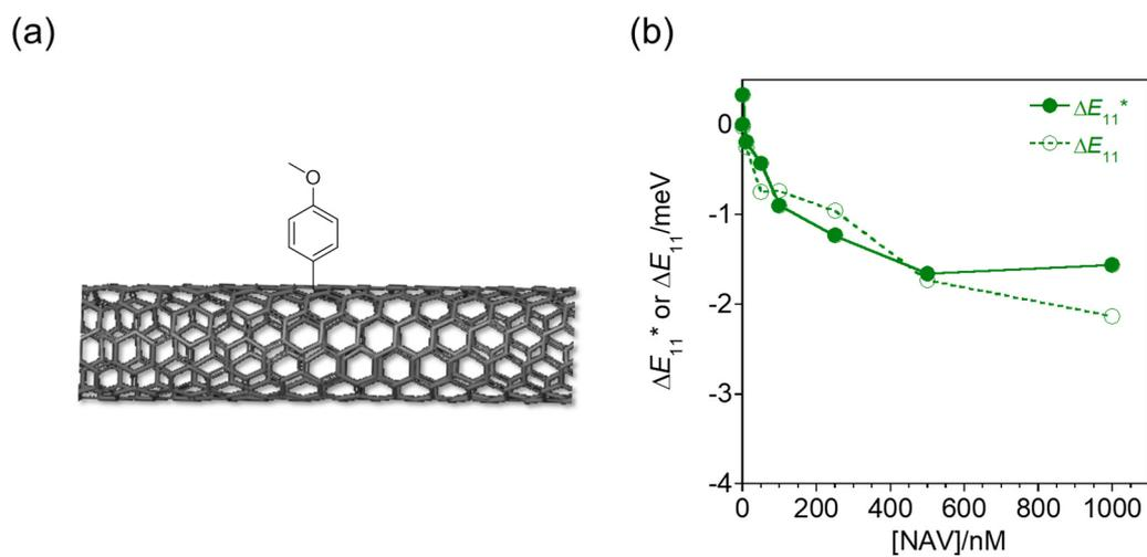
Fig. S8 (a) Schematic image of lf-SWCNTs-OCH<sub>3</sub>. (b) Plots of  $\Delta E_{11}^*$  and  $\Delta E_{11}$  for lf-SWCNT-OCH<sub>3</sub> conjugation with NAV. The average values of technical duplicates are shown.
