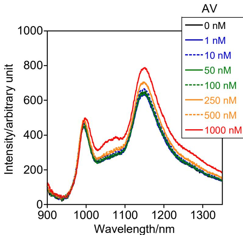
Fig. S13 PL spectra of If-SWCNTs-b after conjugation with AV.  $\lambda_{\text{ex}} = 580 \text{ nm}$ .
