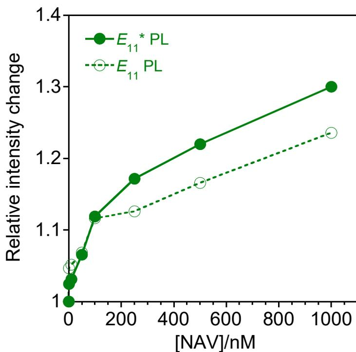
Fig. S6. Plot of the relative intensity changes of  $E_{11}^*$  PL and  $E_{11}$  PL against NAV concentrations.
