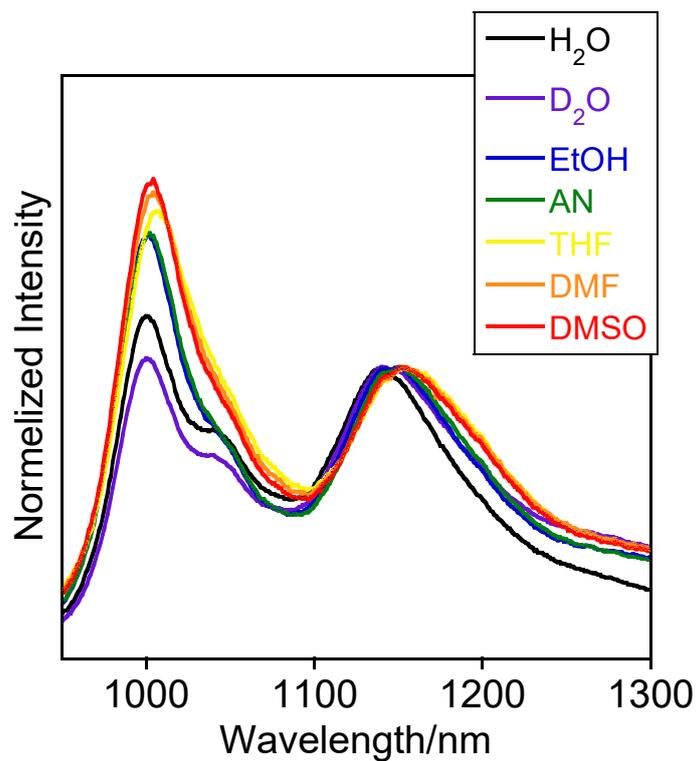
Fig. S3 Normalized PL spectra of If-SWCNTs-b/Na-CMC/PDDA immobilized on quartz substrates, which were immersed in each solvent.  $\lambda_{\text{ex}} = 580$  nm.
