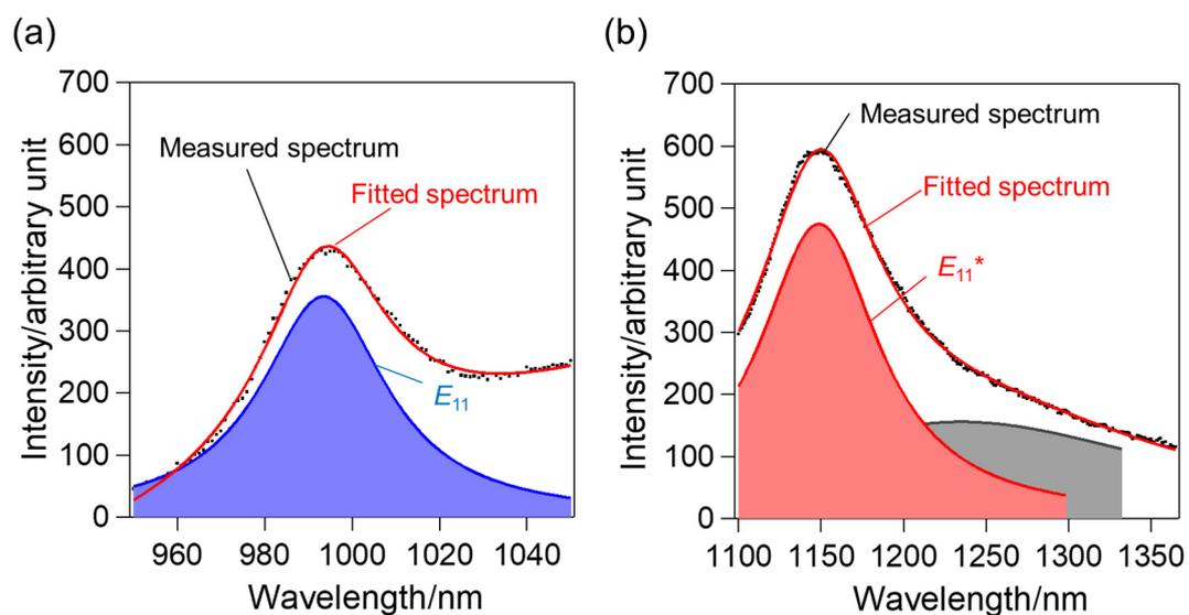
Fig. S18. Deconvoluted PL spectra of If-SWCNTs-b/Na-CMC in  $D_2O$  solutions for (a)  $E_{11}$  PL and (b)  $E_{11}^*$  PL.
