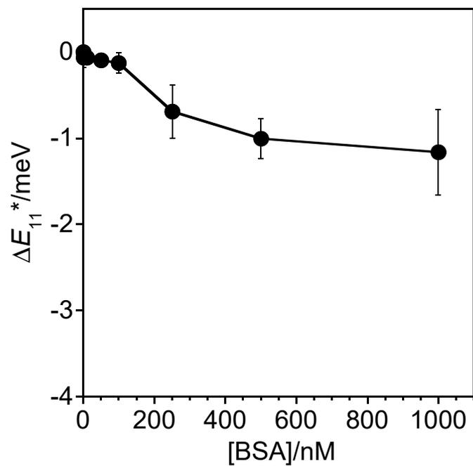
Fig. S9 Plots of the  $\Delta E_{11}^*$  of If-SWCNTs-b as a function of the BSA concentration. Error bars are standard deviations of technical triplicates.
