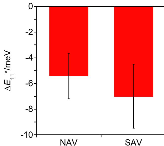
Fig. S16  $\Delta E_{11}^*$  of 1f-SWCNTs-b/Na-CMC on the substrate, after dipping in a NAV solution, where protein concentration is 1000 nM. Error bars are standard deviations of technical triplicates.
