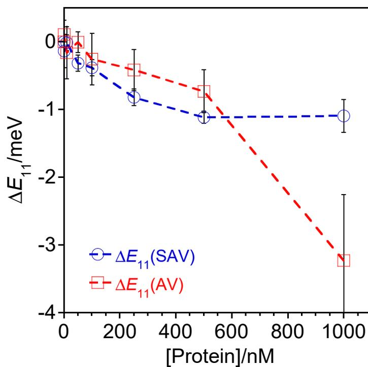
Fig. S14  $\Delta E_{11}$  of If-SWCNTs-b against the AV (red) and SAV (blue) concentrations. Error bars are standard deviations of technical triplicates.
