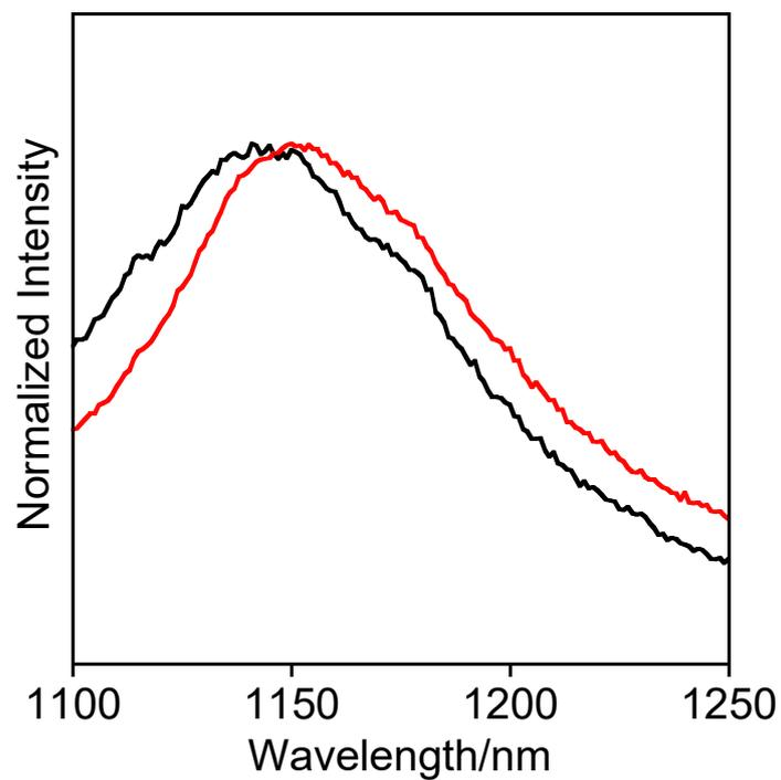
Fig. S15 Normalized PL spectra of 1f-SWCNTs-b/Na-CMC on the APTES-modified substrate before (black) and after (red) immersion in a 1000 nM SAV solution.  $\lambda_{ex} = 580$  nm.
