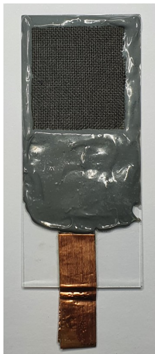
Fig. S2 A working electrode for the electrodeposition of Sn-Cu@Sn dendrites. To get uniform result over the whole area, every side of the carbon cloth was covered with epoxy adhesive. Back side of the electrodes were coated by PTFE to avoid contact with the plating solution.
