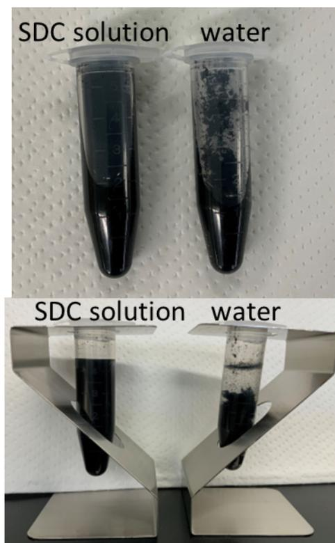
Fig S1. Dispersion of CNT in SDC solution (left) and water (right).
