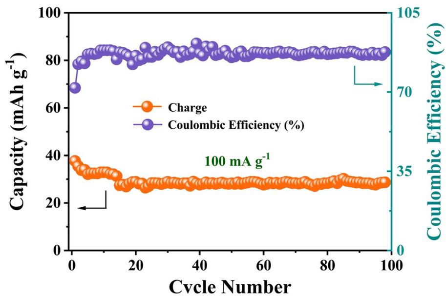
**Fig S21.** Long-term cycling performance of the full cell at 100 mA g<sup>-1</sup> based on the total mass of anode and cathode.
