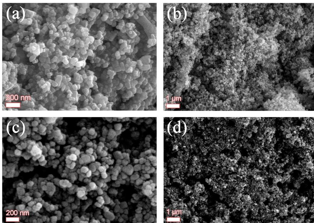
Fig S16. (a-b) SEM image of pristine PNFF-60 electrode. (c-d) SEM image of PNFF-60 electrode after 1500 cycles.
