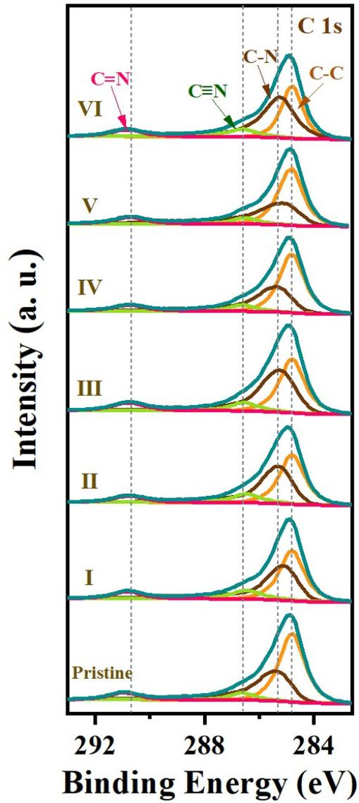
**Fig S17.** Ex-situ XPS spectra for C 1s at pristine and ammoniated/de-ammoniated states.
