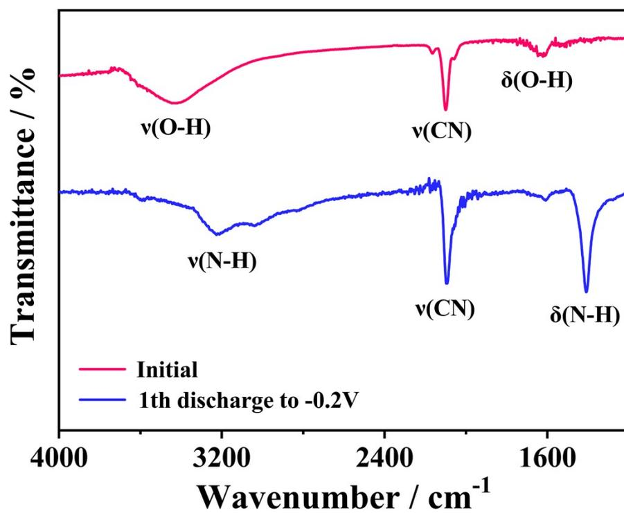
Fig S7. FT-IR spectra of PNFF-60 at different cycle.
