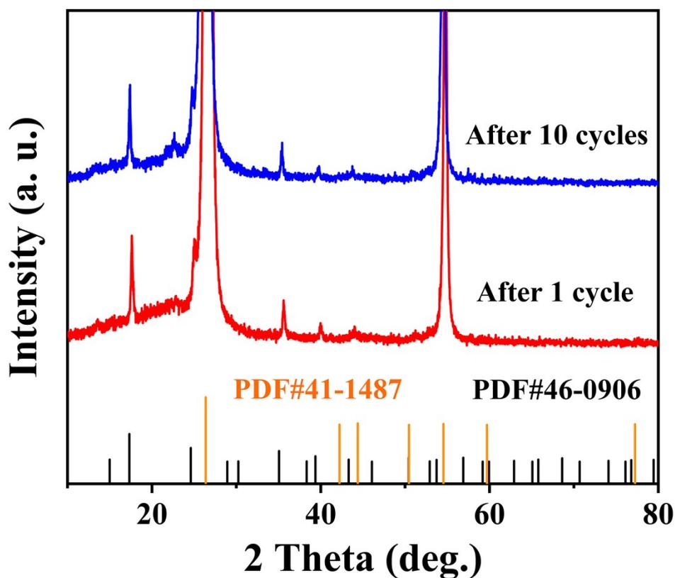
Fig S14. XRD pattern of PNFF-60 after cycles.
