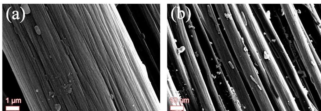
**Fig S12.** SEM image of PANI electrode grown on carbon cloth.
