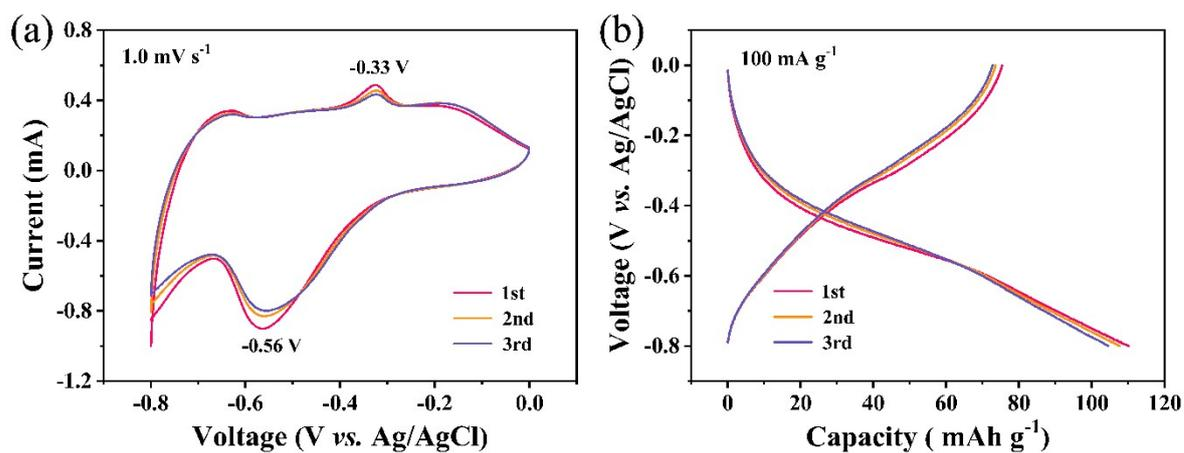
**Fig S19.** Electrochemical characterization of PI@MXene electrode for  $\text{NH}_4^+$  storage a) The first three CV curves at  $1 \text{ mV s}^{-1}$ . b) The first three GCD profiles at  $100 \text{ mA g}^{-1}$ .
