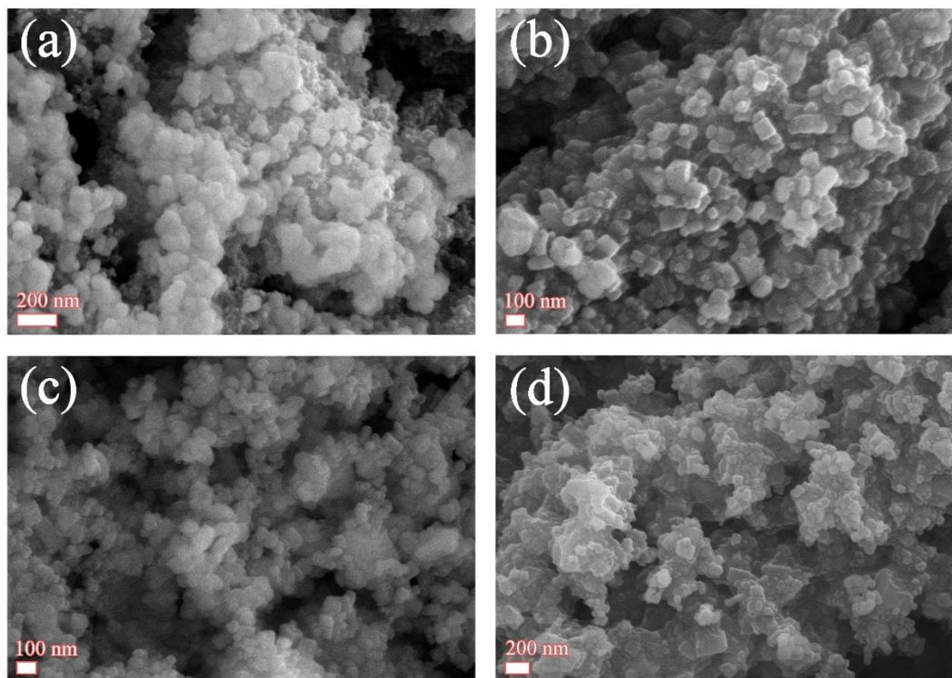
Fig S8. SEM image of a) NFF, b) PNFF-80, c) PNFF-100, d) PNFF-150.
