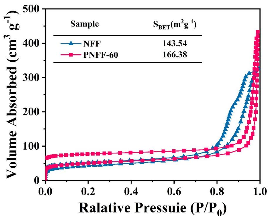
Fig S10. Nitrogen adsorption-desorption isotherm of PNFF-60.
