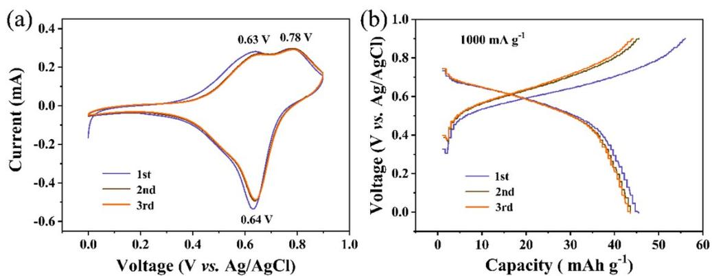
**Fig S11.** Electrochemical characterization of NFF electrode for  $\text{NH}_4^+$  storage a) The first three CV curves at  $1 \text{ mV s}^{-1}$ . b) The first three GCD profiles at  $1000 \text{ mA g}^{-1}$ .
