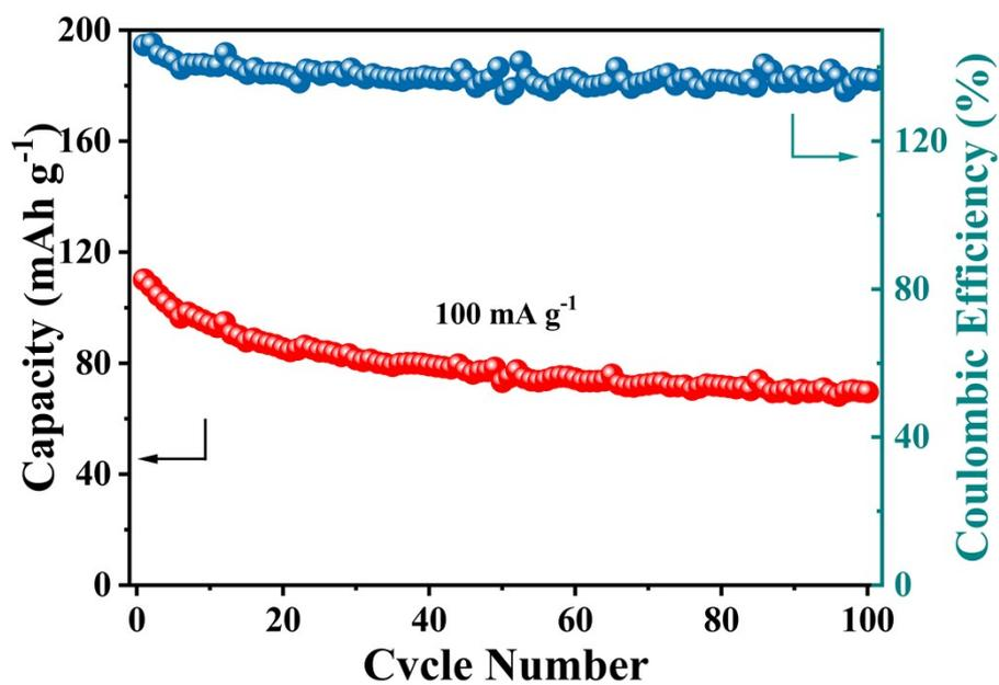
**Fig S20.** Long-term cycling performance of PI@MXene electrode at  $100 \text{ mA g}^{-1}$ .
