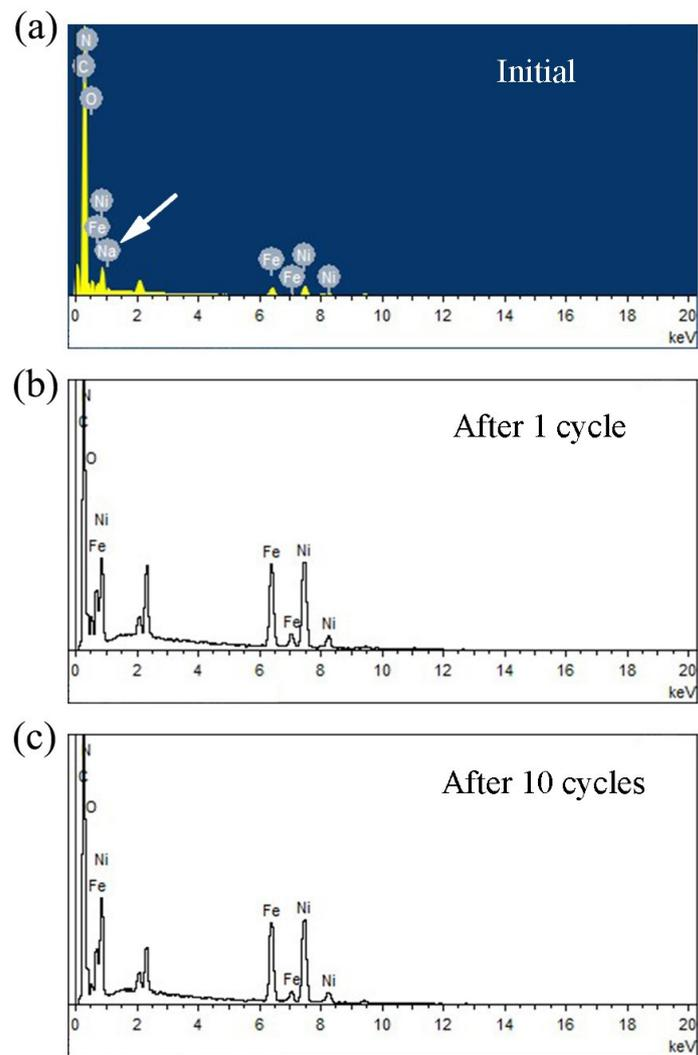
**Fig S6.** Energy dispersive X-ray spectroscopy (EDS) analyses of PNFF-60 at different cycle.
