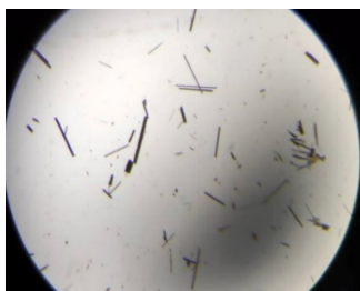
Figure S1. An optical microscopic image of the single crystals of Cd 12 Ag 32 -2 .
