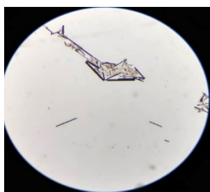
Figure S2. An optical microscopic image of the single crystals of Cd 12 Ag 32 -1 .
