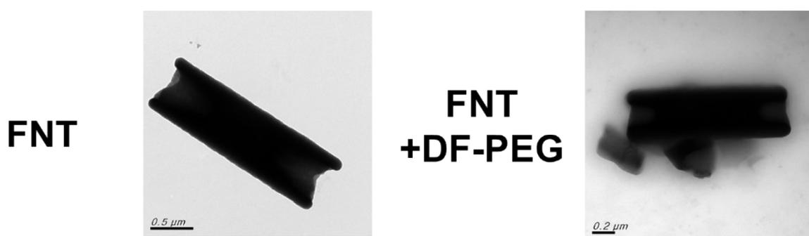
**Figure S8.** Interactions between fullerene nanomaterials and the crosslinker. FNT powder was added to a 2% DF-PEG solution and reacted for 30 min, and then the supernatant was removed by centrifugation. After washing the precipitate with DI water, the precipitate was dropped on a copper grid and dried. TEM images show that DF-PEG was attached around FNT, which was possibly attributed to the chemical bonding between amino groups on FNT and aldehyde groups on DF-PEG.
