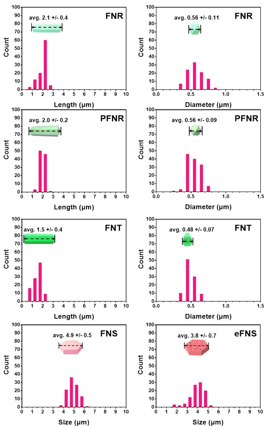
**Figure S2.** The size distribution of hydrophobic or hydrophilic self-assembled fullerenes obtained from the LLIP, Pluronic P123 coating, and EDA selective etching method.
