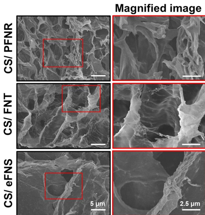
**Figure S7.** SEM images of freeze-dried composite hydrogels with the same concentration (150 µg/mL) of fullerenes.
