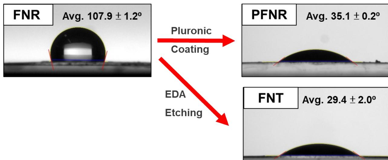
**Figure S1.** Contact angle measurement of FNR before and after hydrophilic surface modification by Pluronic P123 coating or EDA chemical etching.
