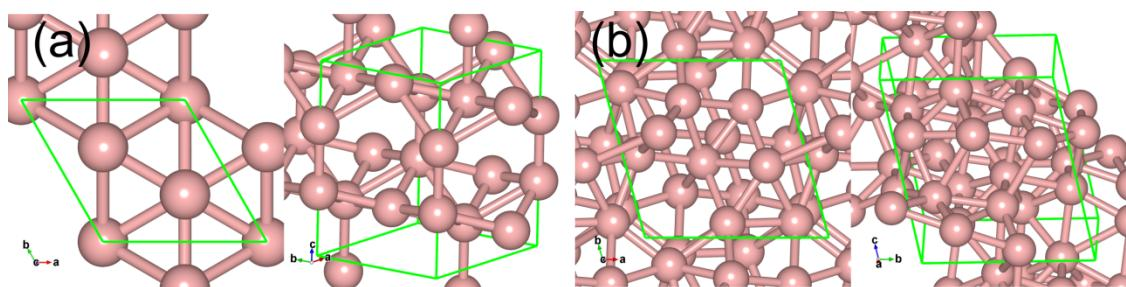
Figure S6. Top and side views of high-pressure phases of (a)  $\delta_6\text{-B}_6$  and (b)  $\alpha\text{-B}_{16}$  at 200 GPa.
