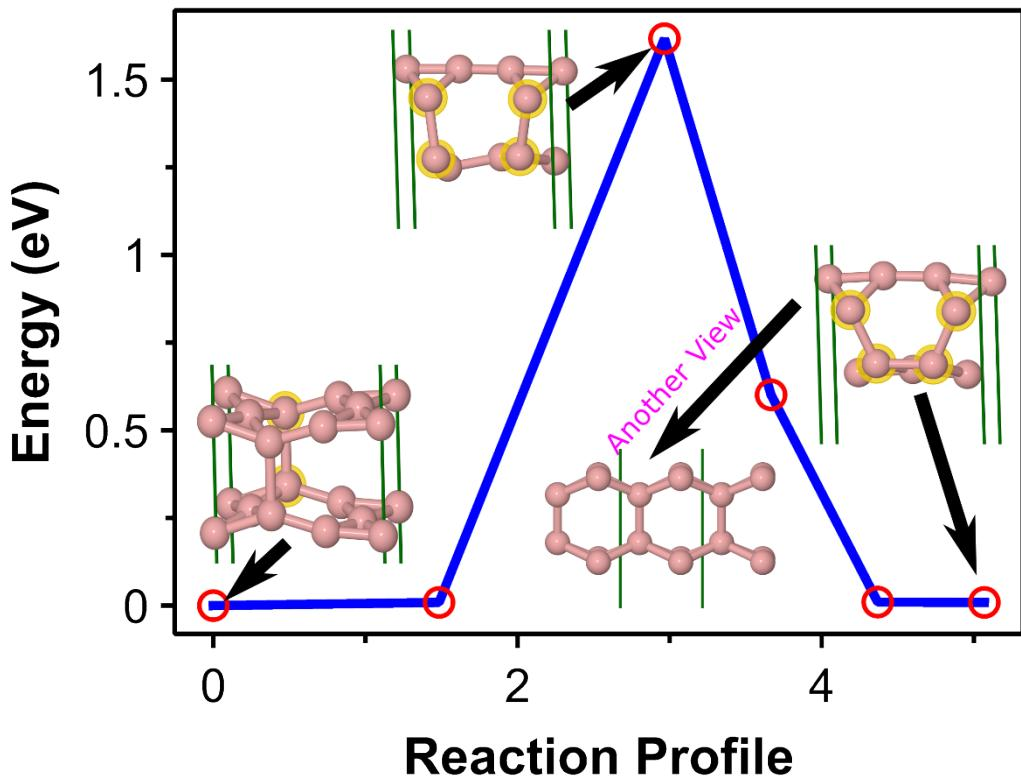
Figure S3. Phase transition from the free-standing bilayer  $\beta_{12}$  borophene to the  $\beta_{12}\text{-B}_5$  bilayer unit. Key connections are marked in halos to illustrate transition details.
