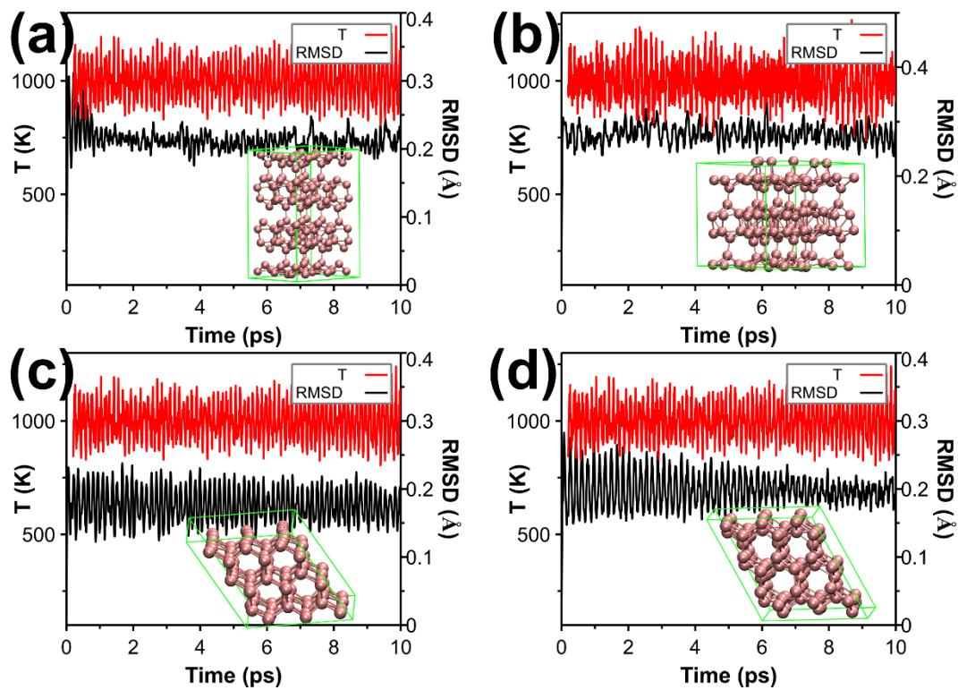
Figure S5. The evolution of the temperatures and root mean square deviations (RMSD) in the BOMD simulations at 1000 K (10 ps) for proposed allotropes (a)  $\delta_6\text{-B}_6$ , (b)  $\alpha\text{-B}_{16}$ , (c)  $\beta_{12}\text{-B}_5$  and (d)  $\delta_3\text{-B}_4$ . The RMSD is calculated using VMD package<sup>[2]</sup>. The snapshots for their last frames are shown as insets.
