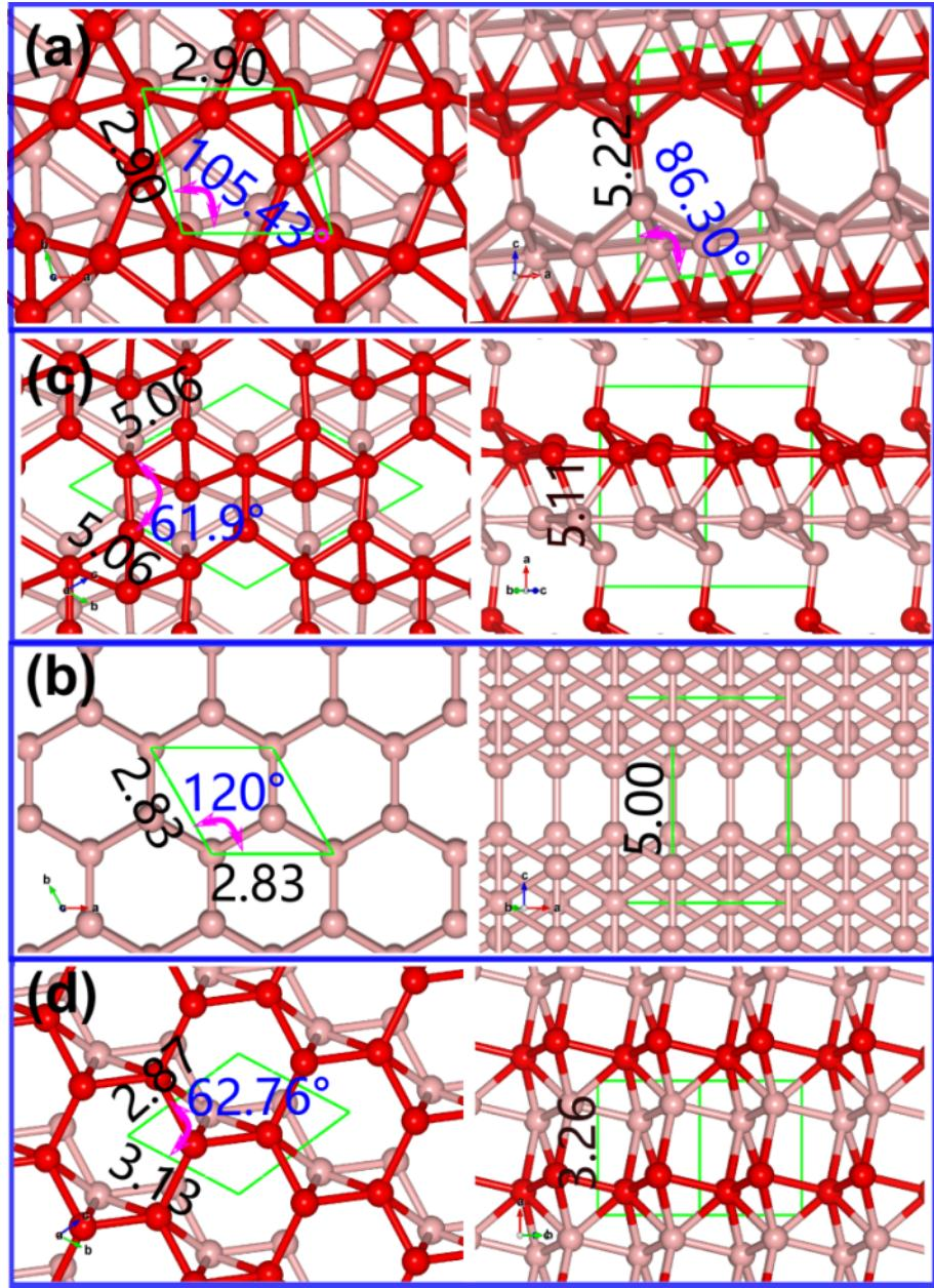
Figure S1. Top and side views of primitive cells converted by AFLOW package<sup>[1]</sup> for proposed allotropes (a)  $\delta_6\text{-B}_6$ , (b)  $\alpha\text{-B}_{16}$ , (c)  $\beta_{12}\text{-B}_5$  and (d)  $\delta_3\text{-B}_4$ .
