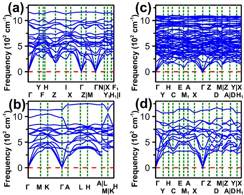
Figure S4. Phonon spectra of (a)  $\delta_6\text{-B}_6$ , (b)  $\alpha\text{-B}_{16}$ , (c)  $\beta_{12}\text{-B}_5$  and (d)  $\delta_3\text{-B}_4$  allotropes by Phonopy program with  $3 \times 3 \times 3$  supercells.
