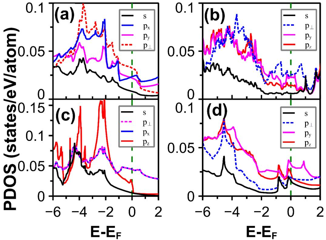
Figure S7. Projected density of states (PDOS) for proposed allotropes (a)  $\delta_6\text{-B}_6$ , (b)  $\alpha\text{-B}_{16}$ , (c)  $\beta_{12}\text{-B}_5$  and (d)  $\delta_3\text{-B}_4$  at PBE level.  $p_{\perp}$  stands for  $p$  states basically perpendicular to the basal plane of precursor borophenes.
