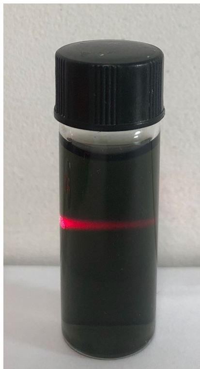
Fig. S1 Image of the dispersion in aqueous solution of \text{Ti}_3\text{C}_2 nanosheets with the Tyndall effect.
