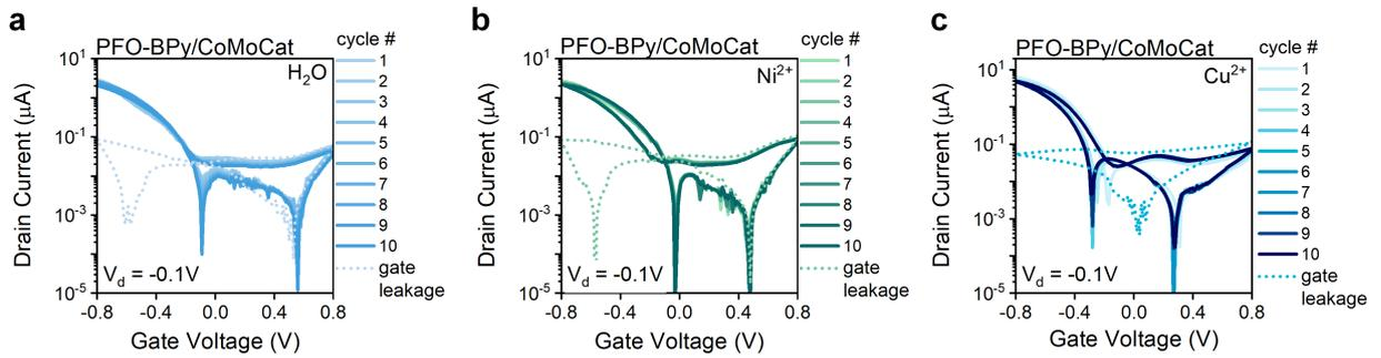
**Figure S2.** Conditioning of PFO-BPy/CoMoCat SWNT network-based, water-gated transistors (ten consecutive cycles of transfer characteristics, sweep rate  $\sim 50$  mV/sec, total measurement time  $\sim 13$  min) with (a) de-ionized water, (b)  $15 \mu\text{M Ni}^{2+}$  aqueous solution, (c)  $15 \mu\text{M Cu}^{2+}$  aqueous solution as electrolyte.
