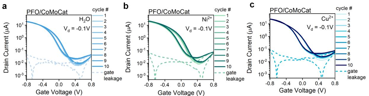
**Figure S3.** Conditioning of a reference transistor based on a PFO/CoMoCat SWNT network (ten consecutive cycles of transfer characteristics, sweep rate  $\sim 50$  mV/sec, total measurement time  $\sim 13$  min) with (a) de-ionized water, (b)  $15 \mu\text{M Ni}^{2+}$  aqueous solution, (c)  $15 \mu\text{M Cu}^{2+}$  aqueous solution as electrolyte.
