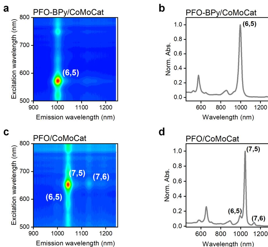
**Figure S1.** PLE maps and absorbance spectra of PFO-BPy/CoMoCat (a,b) and PFO/CoMoCat (c,d) dispersions in toluene. The absorption peaks at 575 nm and 650 nm correspond to the  $E_{22}$  transitions of the (6,5) and (7,5) SWNTs, respectively.
