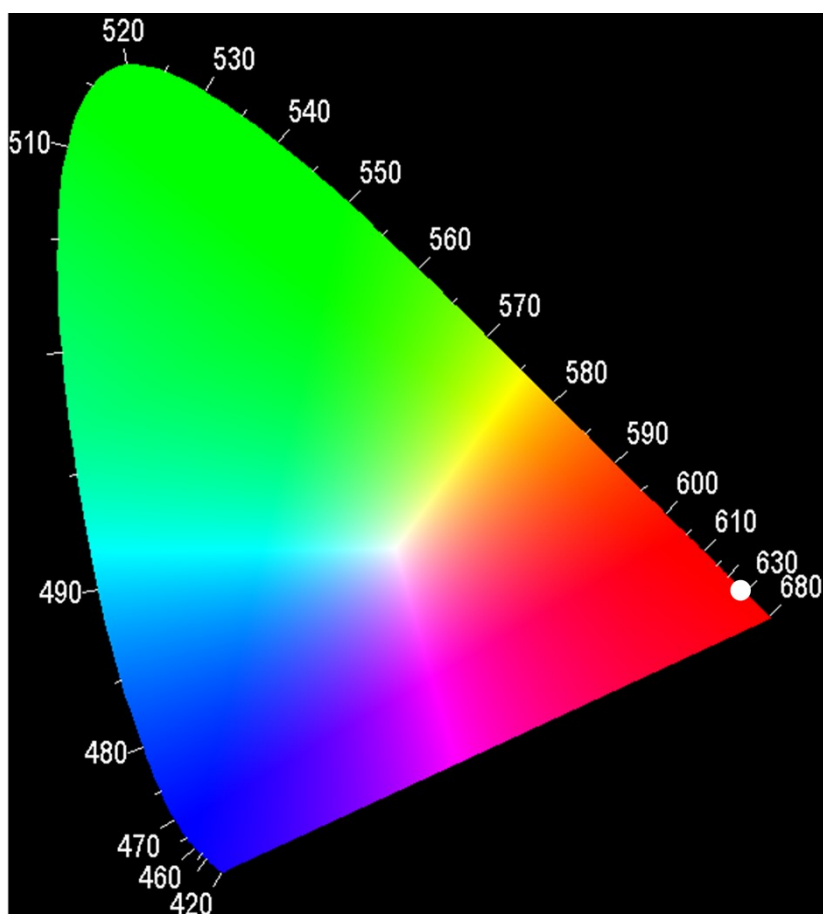
Figure S7: CIE diagram for \{\text{Gd}_8\text{Ho}_2\text{Yb}_{10}\} MCA. ( P = 16 \text{ W cm}^{-2} ).
