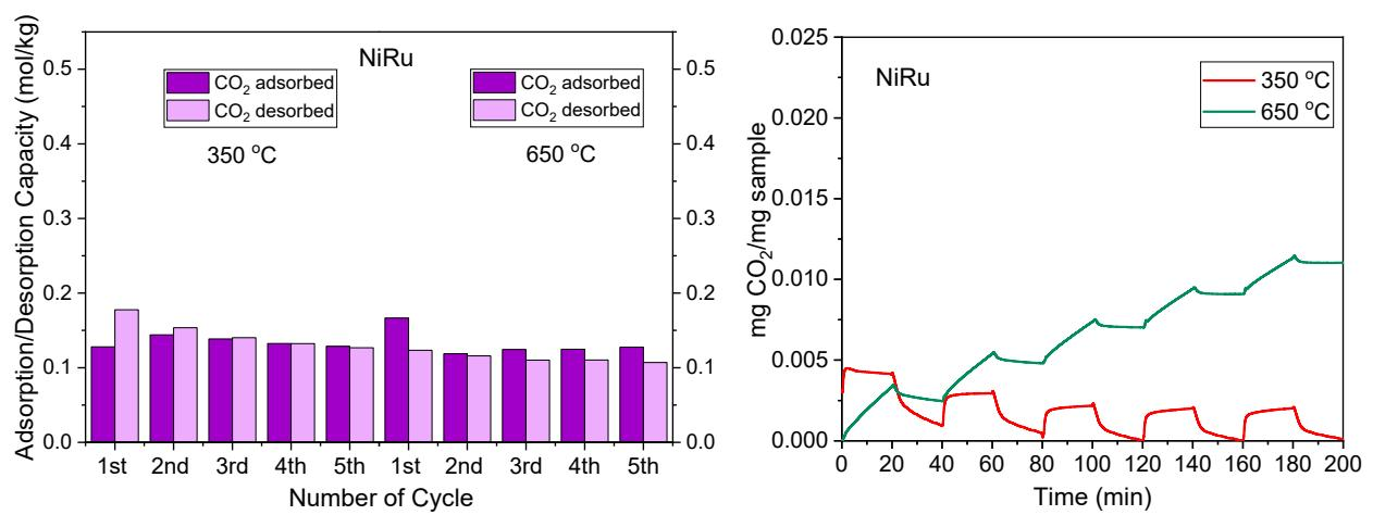
**Figure S3** TGA adsorption-desorption results at different temperatures for NiRu
