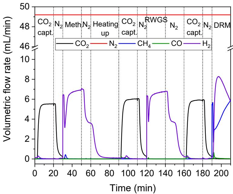
**Figure S5** CO<sub>2</sub> capture and CO<sub>2</sub> methanation, followed by the RWGS and DRM for NiRuk
