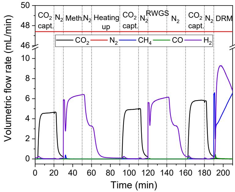
**Figure S4** CO<sub>2</sub> capture and CO<sub>2</sub> methanation, followed by the RWGS and DRM for NiRuNa
