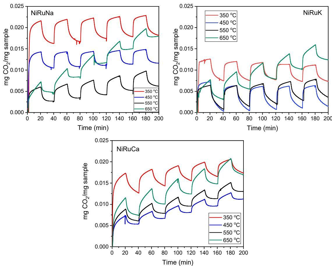
**Figure S1** TGA adsorption-desorption results at different temperatures for NiRuNa, NiRuK and NiRuCa
