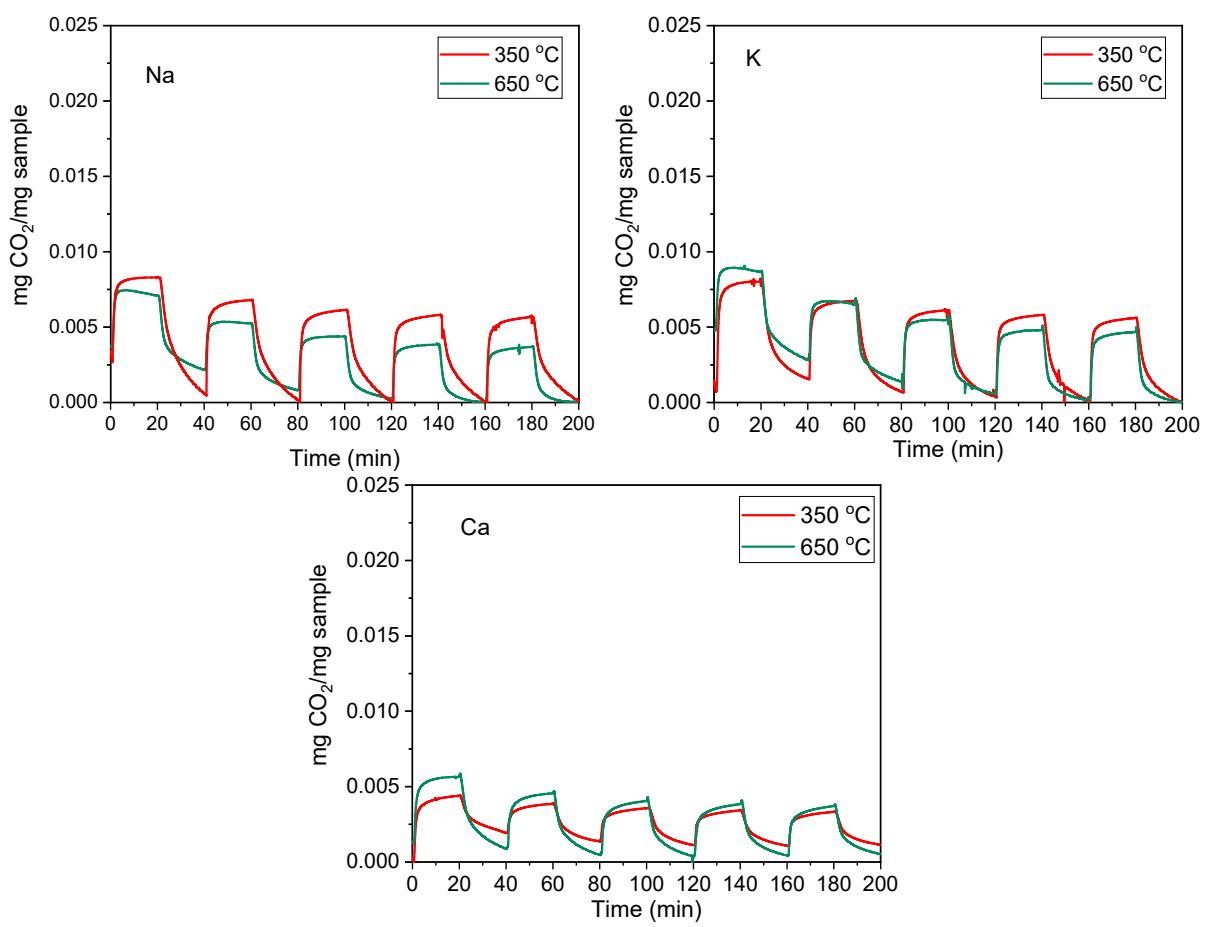
**Figure S2** TGA adsorption-desorption results at different temperatures for Na, K and Ca
