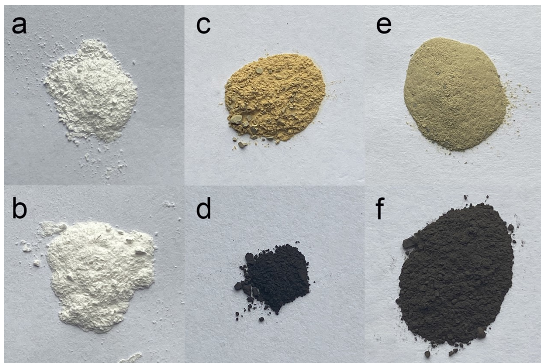
Figure S6. Graphs of bulk samples of (a) MOF-808, (b) MOF-808-Pza, (c) Pd@MOF-808-Pza, (d) Pd-nano@MOF-808-Pza, (e) Pd@MOF-808, and (f) Pd-nano@MOF-808, respectively.
