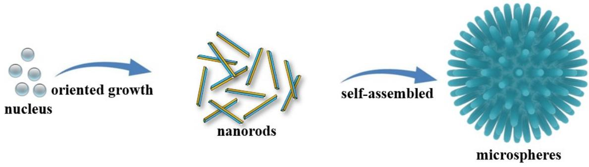
**Fig. S3.** The possible formation process of Nb<sub>2</sub>O<sub>5</sub>-MS.
