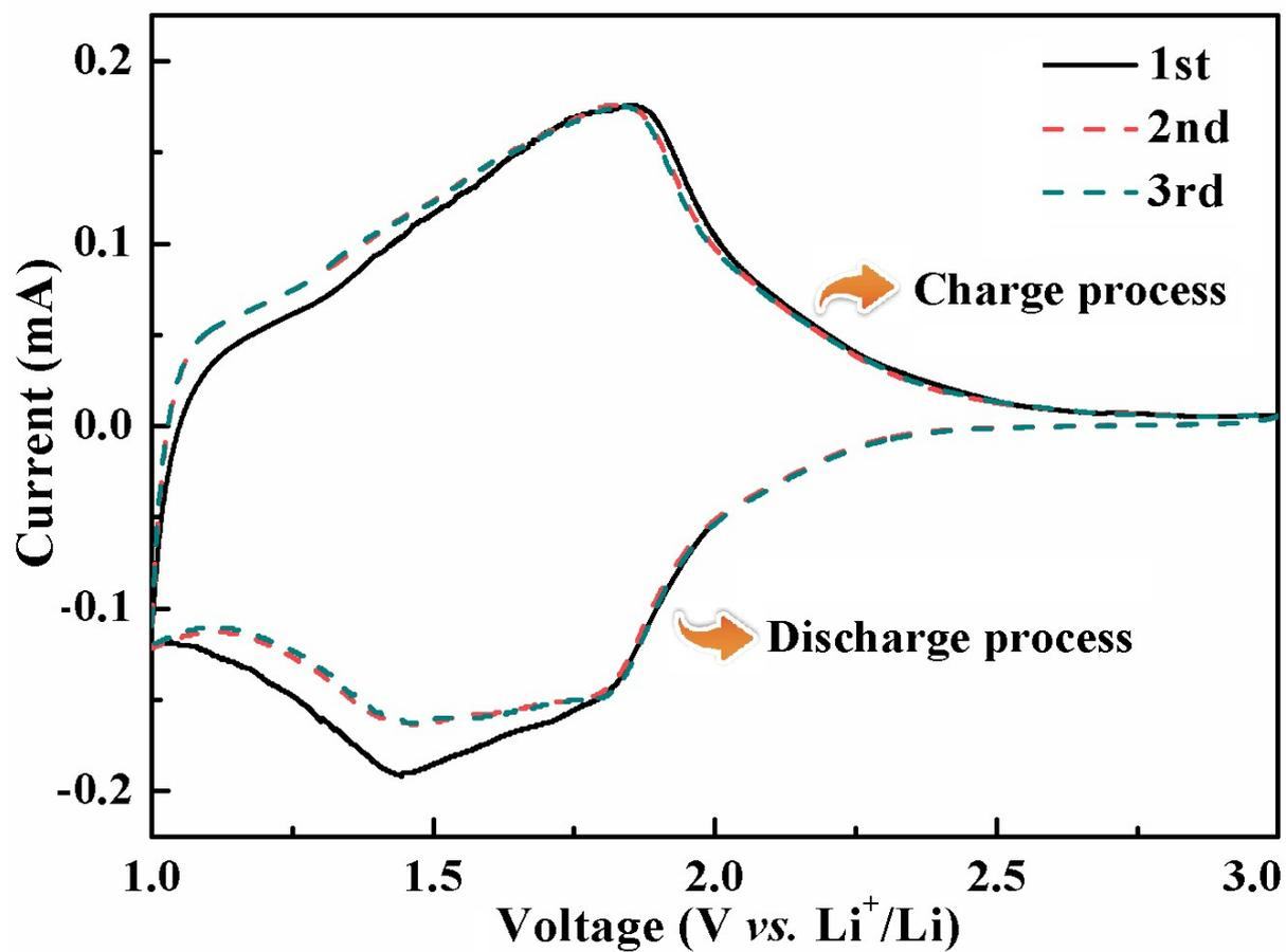
**Fig. S4.** The initial three CV curves of N-Nb<sub>2</sub>O<sub>5</sub> in a voltage range of 1.0-3.0 V (vs. Li/Li<sup>+</sup>) at a scan rate of 0.1 mV s<sup>-1</sup>.
