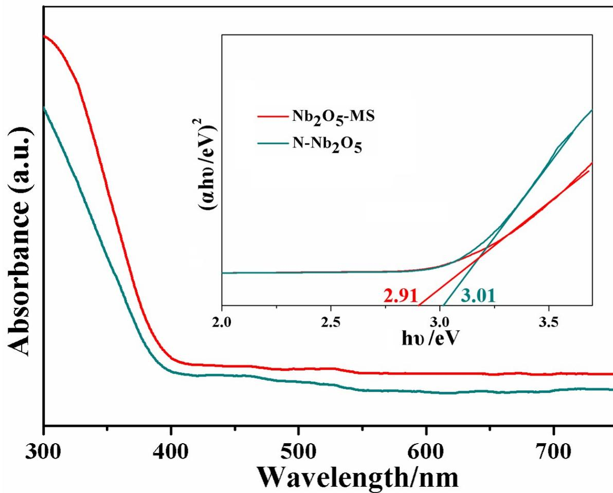
Fig. S8. UV-Vis diffuse reflectance spectra and the corresponding Tauc's curves of  $\text{N-Nb}_2\text{O}_5$  and  $\text{Nb}_2\text{O}_5\text{-MS}$ .
