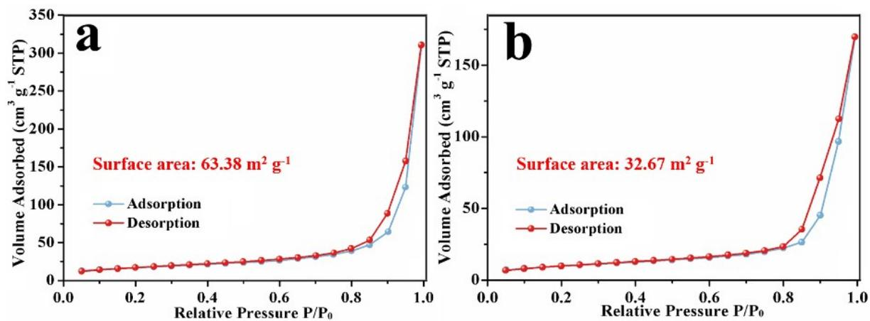
**Fig. S2.** Nitrogen adsorption-desorption isotherms of (a) N-Nb<sub>2</sub>O<sub>5</sub> and (b) Nb<sub>2</sub>O<sub>5</sub>-MS.
