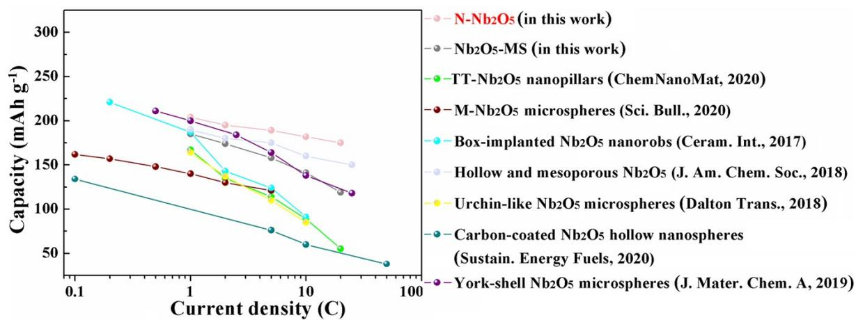
**Fig. S5.** The comparison of the rate capabilities between the obtained N-Nb<sub>2</sub>O<sub>5</sub>, Nb<sub>2</sub>O<sub>5</sub>-MS, and other previously reported Nb<sub>2</sub>O<sub>5</sub>-based anodes.
