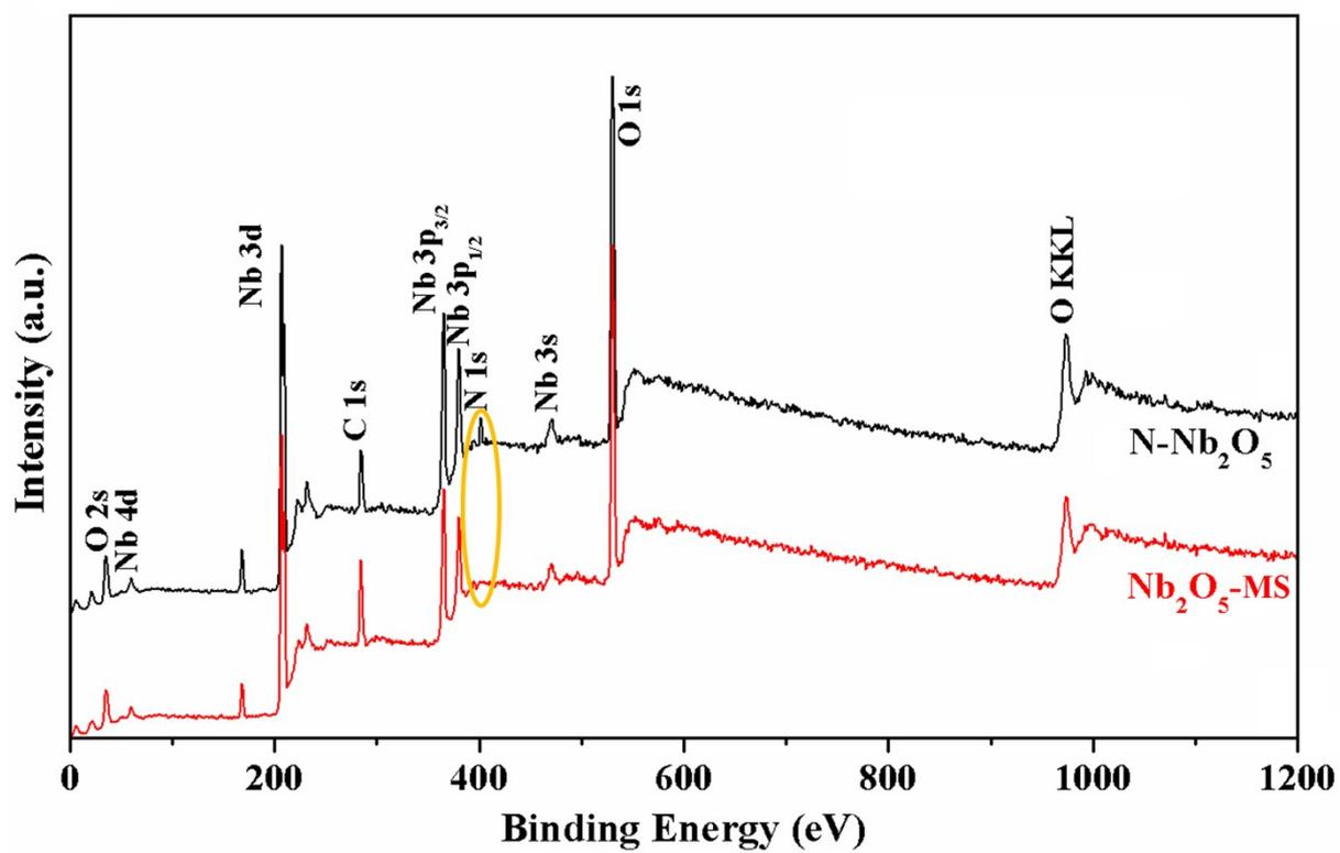
Fig. S1. XPS spectra of N-Nb<sub>2</sub>O<sub>5</sub> and Nb<sub>2</sub>O<sub>5</sub>-MS.
