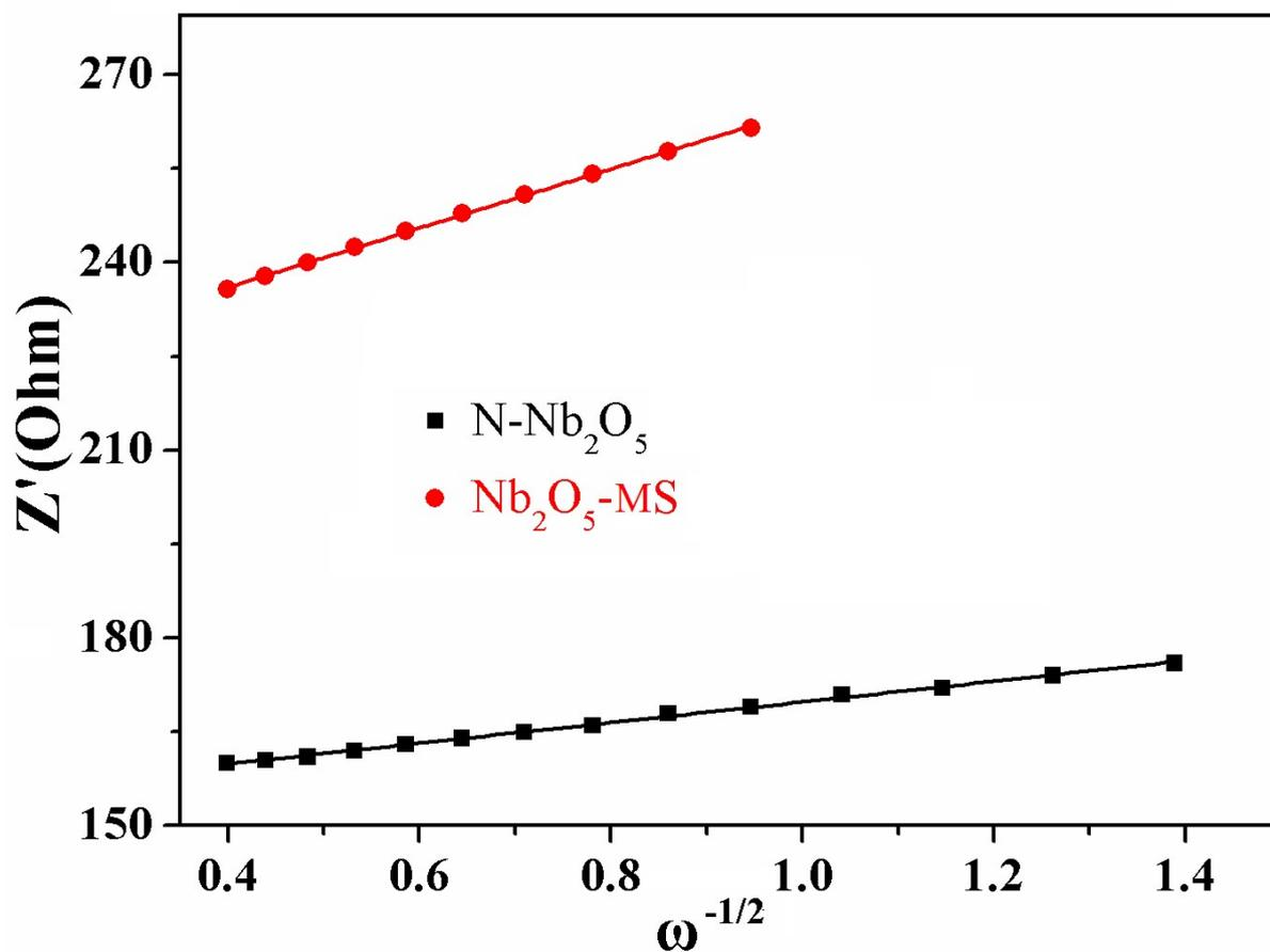
**Fig. S6.** Relationship between imaginary resistance ( $Z'$ ) and inverse square root of angular speed ( $\omega^{-0.5}$ ) at low frequency region.
