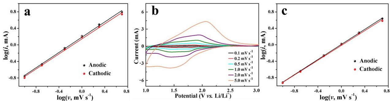
**Fig. S7.** (a) Plots of  $\log(i)$  vs.  $\log(v)$  used to calculate  $b$ -values of N-Nb<sub>2</sub>O<sub>5</sub>; (b) cyclic voltammograms of Nb<sub>2</sub>O<sub>5</sub>-MS at different scanning rates with potential window of 1.0-3.0 V vs. Li/Li<sup>+</sup>; (c) plots of  $\log(i)$  vs.  $\log(v)$  used to calculate  $b$ -values of Nb<sub>2</sub>O<sub>5</sub>-MS.
