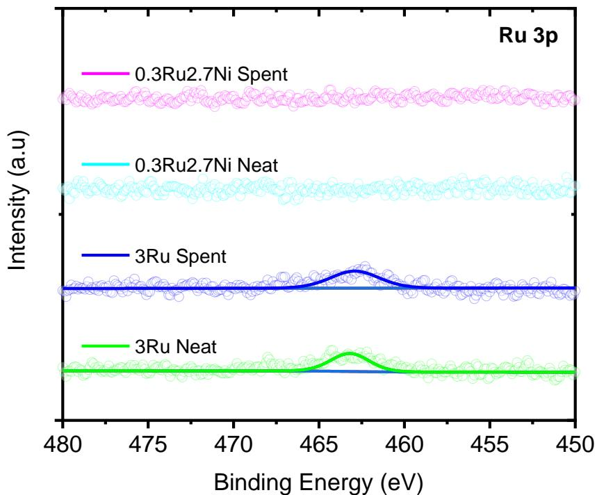
**Figure S10.** High-resolution XPS spectra for the Ru 3p region of Mg-CUK-1 before and loading with Ni and Ru.
