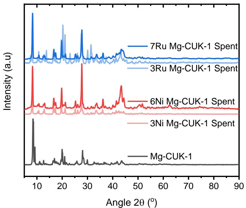
**Figure S3.** X-ray diffraction patterns of spent Ni- and Ru-loaded Mg-CUK-1 following steady state CO<sub>2</sub> hydrogenation performance tests.
