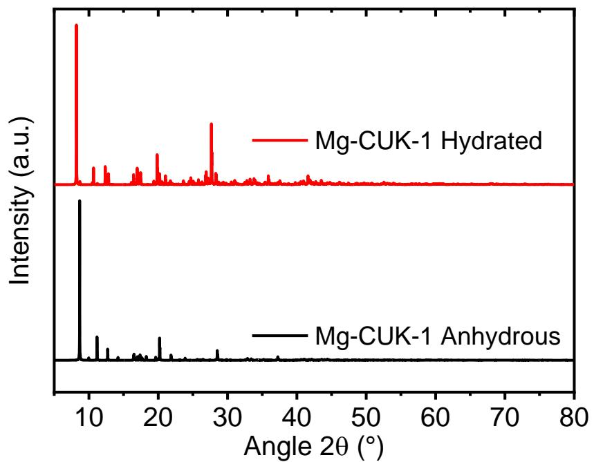
**Figure S1.** Simulated powder XRD patterns for Mg-CUK-1 under anhydrous and hydrated conditions.
