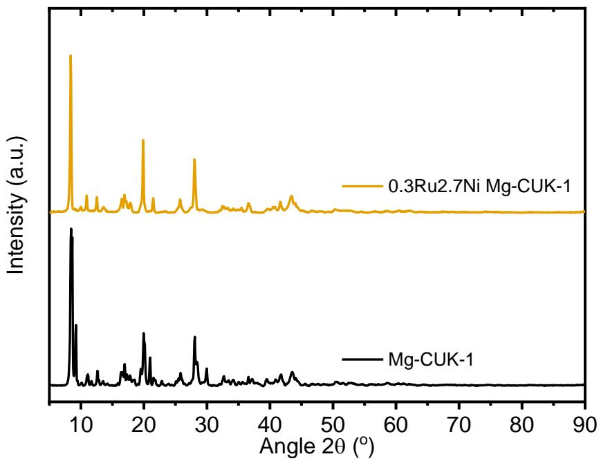
**Figure S5.** X-ray diffraction patterns of 0.3Ru2.7Ni-loaded Mg-CUK-1. Neat Mg-CUK-1 is provided for comparison.
