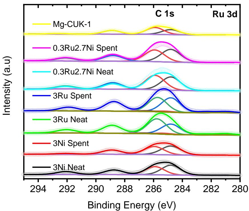
**Figure S9.** High-resolution XPS spectra for the C 1s and Ru 3d region of Mg-CUK-1 before and loading with Ni and Ru.
