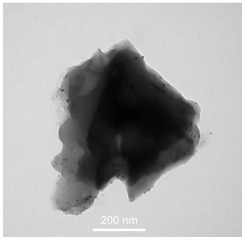
**Figure S14.** Transmission electron micrograph of 0.3Ru2.7Ni Mg-CUK-1.
