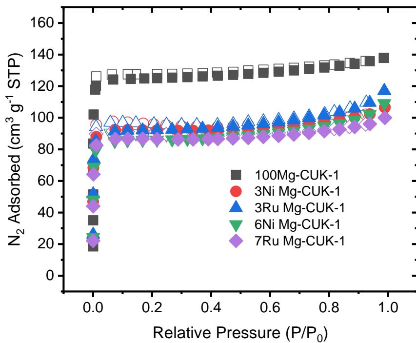
**Figure S2.** N<sub>2</sub> adsorption isotherms of Mg-CUK-1 before and after loading with Ni and Ru.
