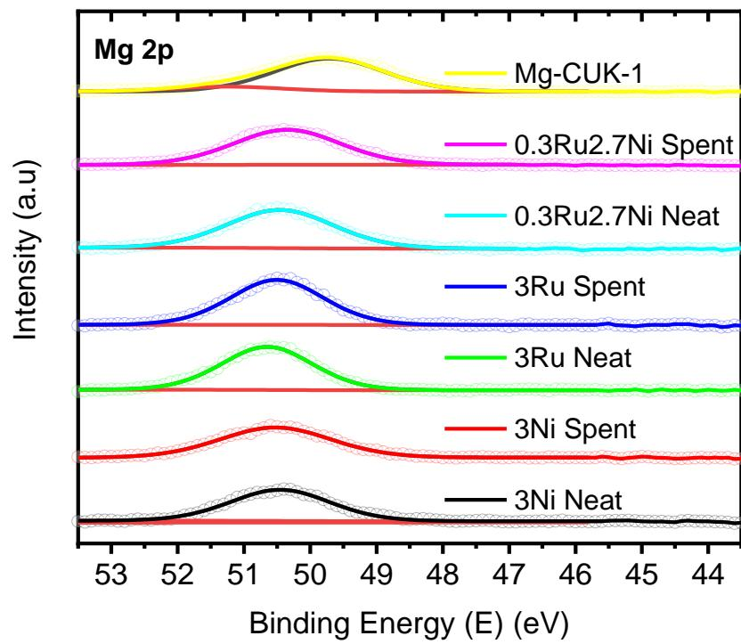
**Figure S11.** High-resolution XPS spectra for the Mg 2p region of Mg-CUK-1 before and loading with Ni and Ru.
