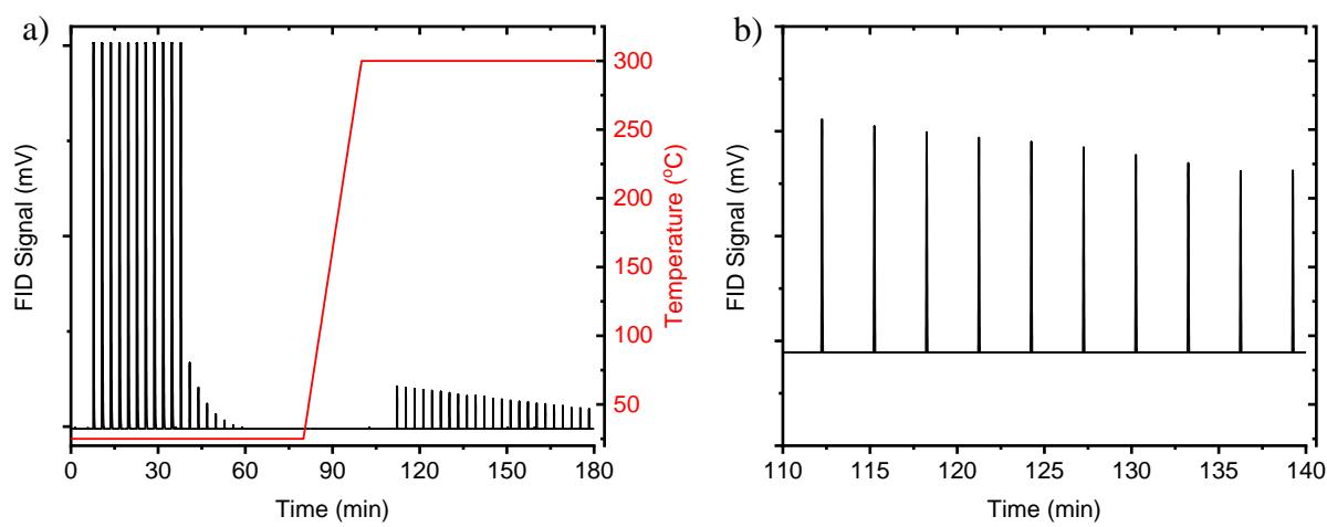
**Figure S4.** Representative gas chromatograph flame ionization detector (GC-FID) signal for the CO<sub>2</sub> capture and conversion experimental runs. a) Complete experimental time on stream data and b) first 10 peaks associated with CH<sub>4</sub> generation.
