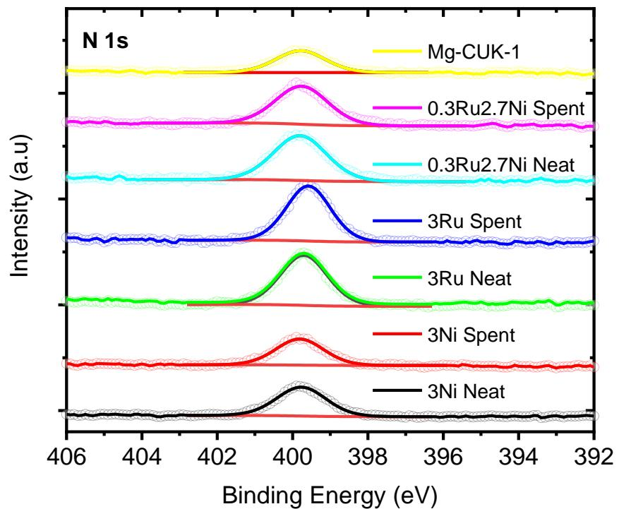
**Figure S13.** High-resolution XPS spectra for the N 1s region of Mg-CUK-1 before and loading with Ni and Ru.
