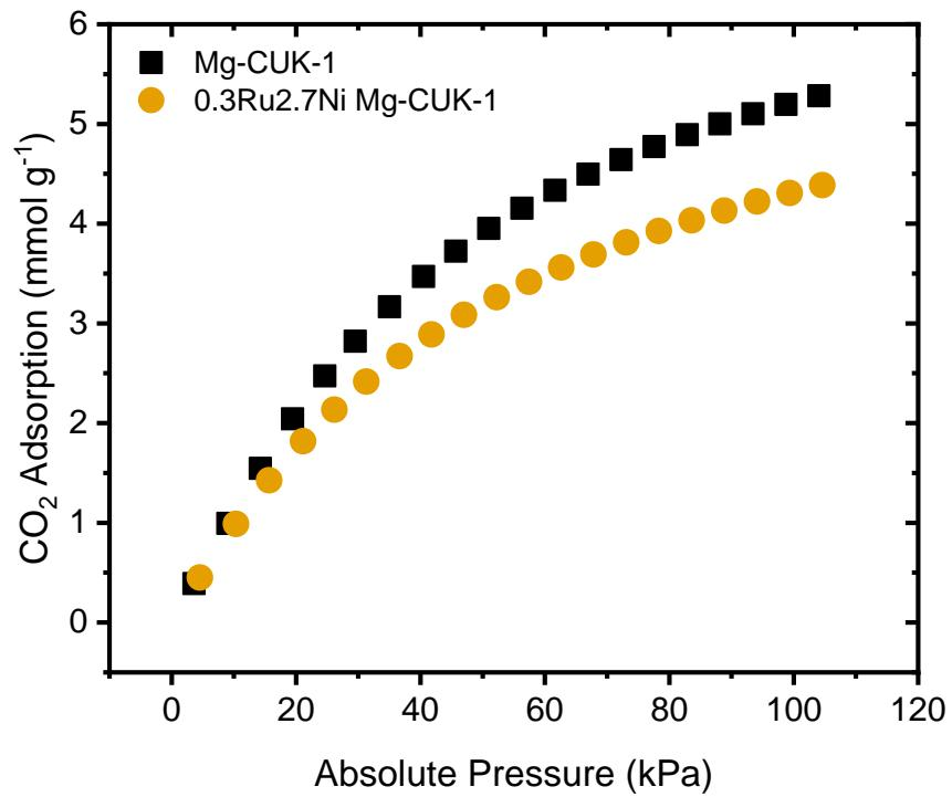
**Figure S6.** CO<sub>2</sub> adsorption isotherm of 0.3Ru2.7Ni Mg-CUK-1. Neat Mg-CUK-1 is provided for comparison
