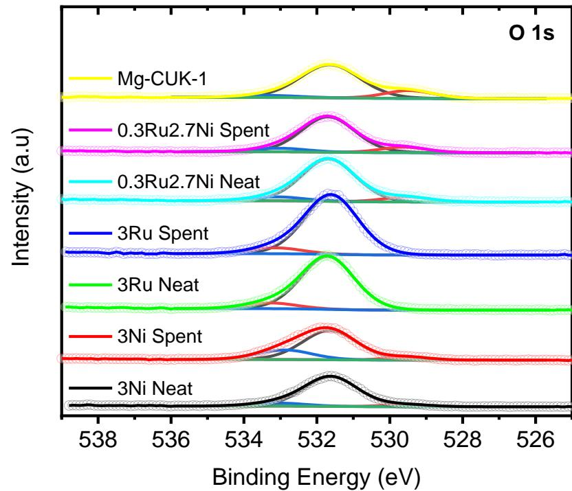
**Figure S12.** High-resolution XPS spectra for the O 1s region of Mg-CUK-1 before and loading with Ni and Ru.
