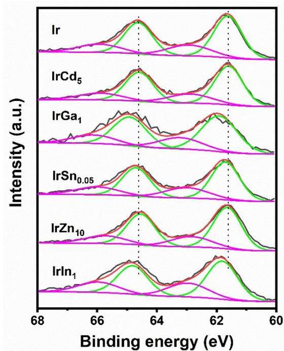
Fig. S14. (a) XPS spectra of Ir 4f in Ir and Ir-M alloy catalysts.
