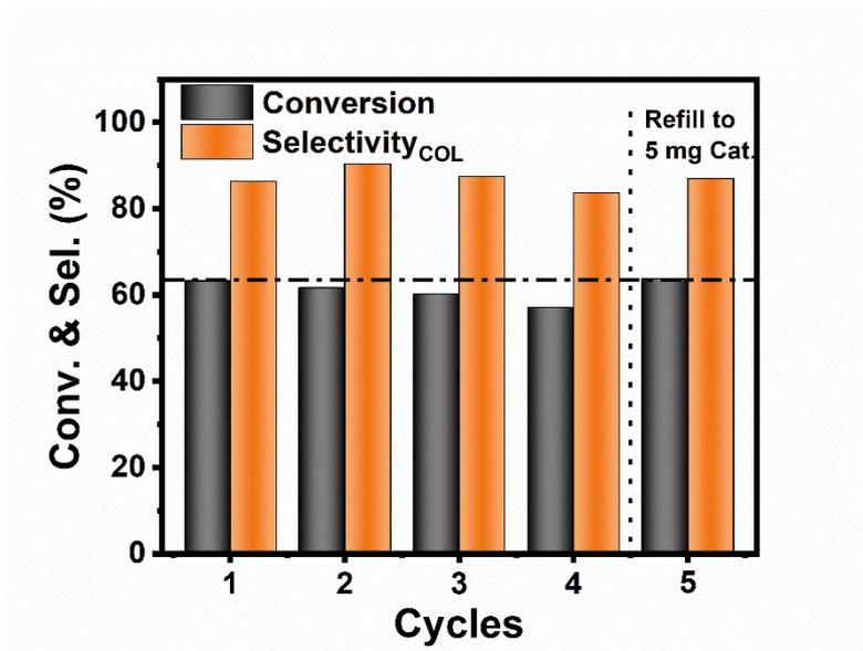
Fig. S16 Recycle test of IrCd<sub>5</sub>. Reaction condition: 5 mg IrCd<sub>5</sub>, 50  $\mu$ L CAL, 1 mL isopropanol, 1 mL DIW, RT, 1 MPa H<sub>2</sub>, 6 h. After 4 cycles reaction, the amount of catalyst was refilled to 5 mg, and then carried out the fifth cycle test. Fortunately, the catalytic performance recovered to a level comparable to that of the first cycle, demonstrating the impressive stability of IrCd<sub>5</sub> catalyst.
