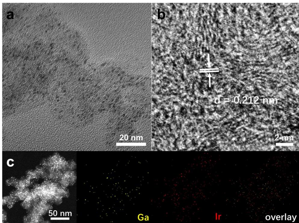
Fig. S10 (a) TEM (b) HRTEM image (c) HAADF-STEM-EDS element mappings of IrGa<sub>1</sub>.
