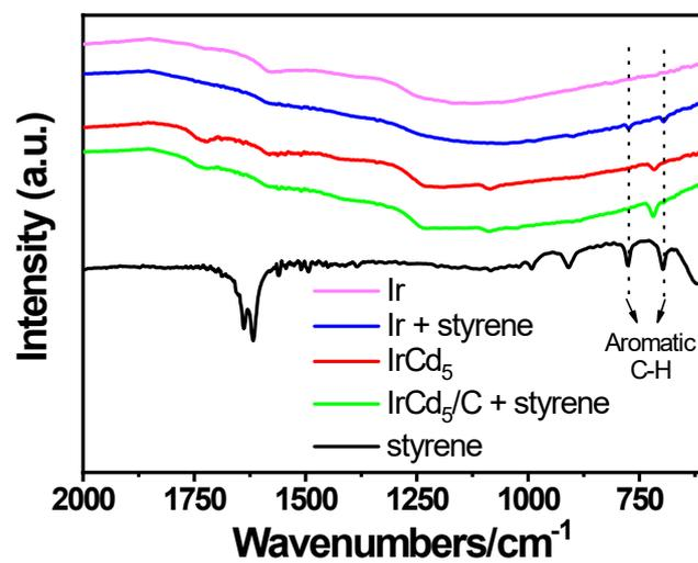
Fig. S15 IR spectra of the catalysts treated with styrene. The doublet 770 and 690 cm<sup>-1</sup> associate with the Aromatic C-H, and the signal at 720 cm<sup>-1</sup> assigns to C-Cl bond.
