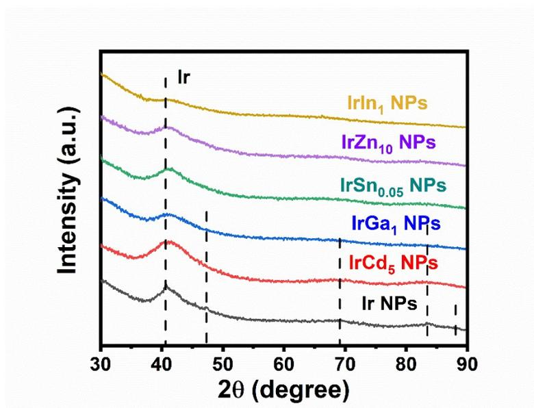
Fig. S4 XRD patterns of Ir-M nanoparticles
