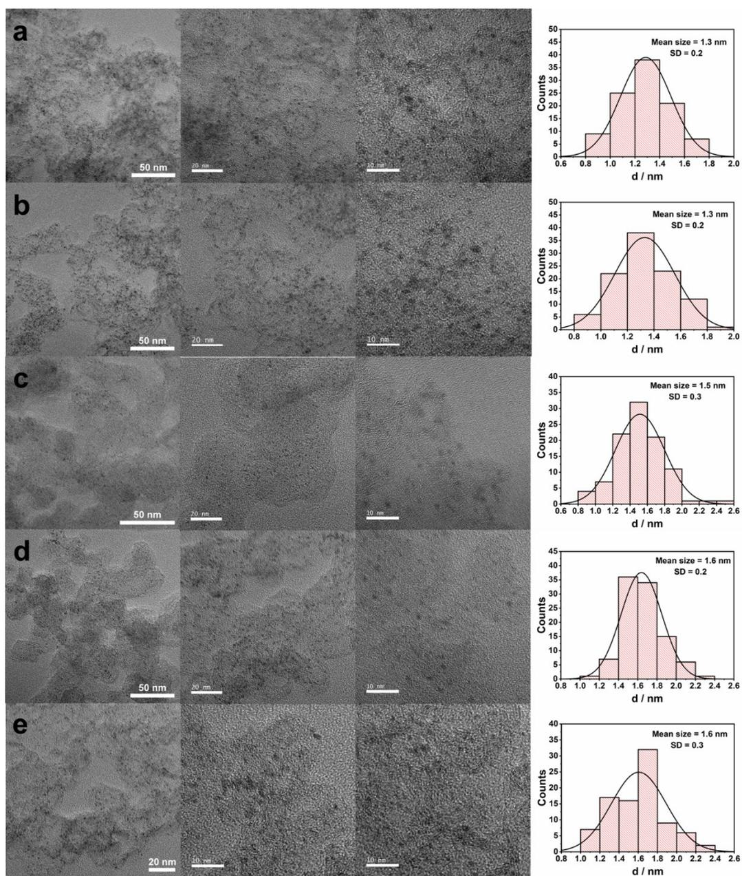
Fig. S5 TEM images and corresponding nanoparticle size distribution of (a) IrCd<sub>0.5</sub> (b) IrCd<sub>1</sub> (c) IrCd<sub>2</sub> (d) IrCd<sub>5</sub> and (e) IrCd<sub>10</sub>.
