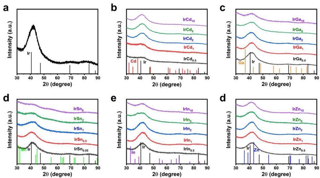
Fig. S3 XRD patterns of carbon black supported (a) Ir, (b) IrCd<sub>x</sub>, (c) IrGa<sub>x</sub>, (d) IrSn<sub>x</sub>, (e) IrIn<sub>x</sub>, (f) IrZn<sub>x</sub>.
