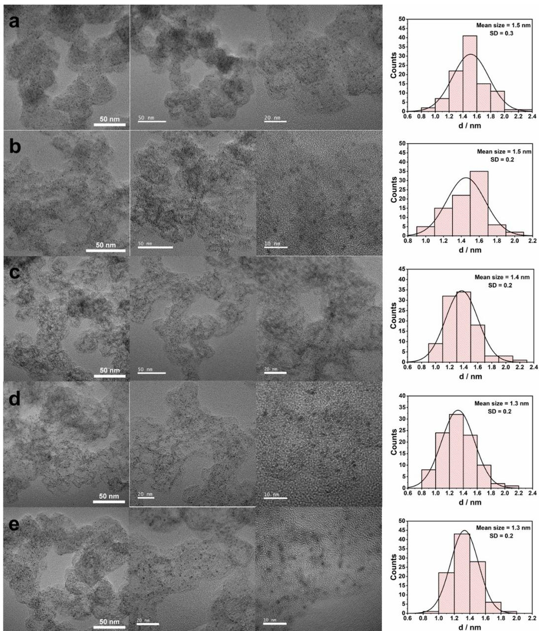
Fig. S9 TEM image and corresponding nanoparticle size distribution of (a) IrIn<sub>0.5</sub> (b) IrIn<sub>1</sub> (c) IrIn<sub>2</sub> (d) IrIn<sub>5</sub> and (e) IrIn<sub>10</sub>.
