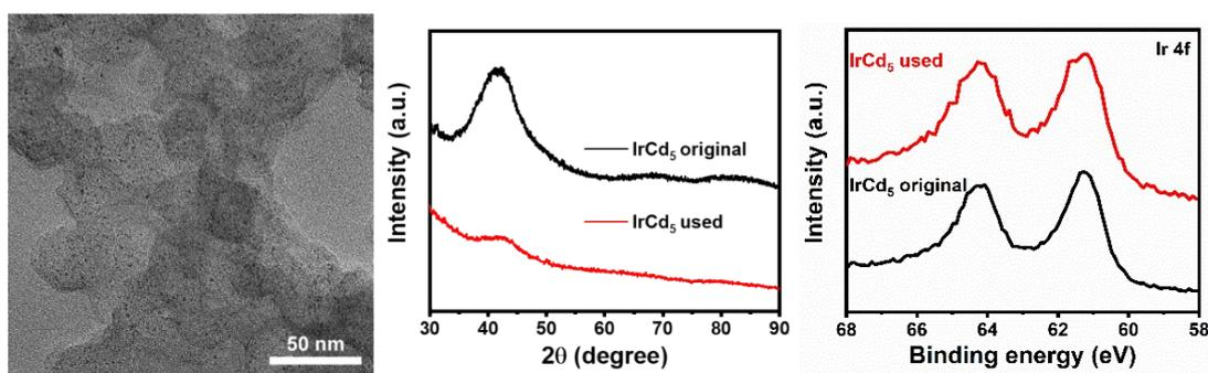
Fig. S17 TEM image, XRD and XPS pattern of used IrCd<sub>5</sub>.
