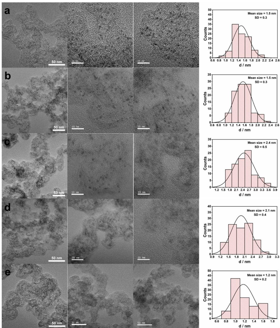
Fig. S7 TEM image and corresponding nanoparticle size distribution of (a) IrSn<sub>0.05</sub>, (b) IrSn<sub>0.5</sub>, (c) IrSn<sub>1</sub> and (d) IrSn<sub>2</sub> and (e) IrSn<sub>5</sub>.
