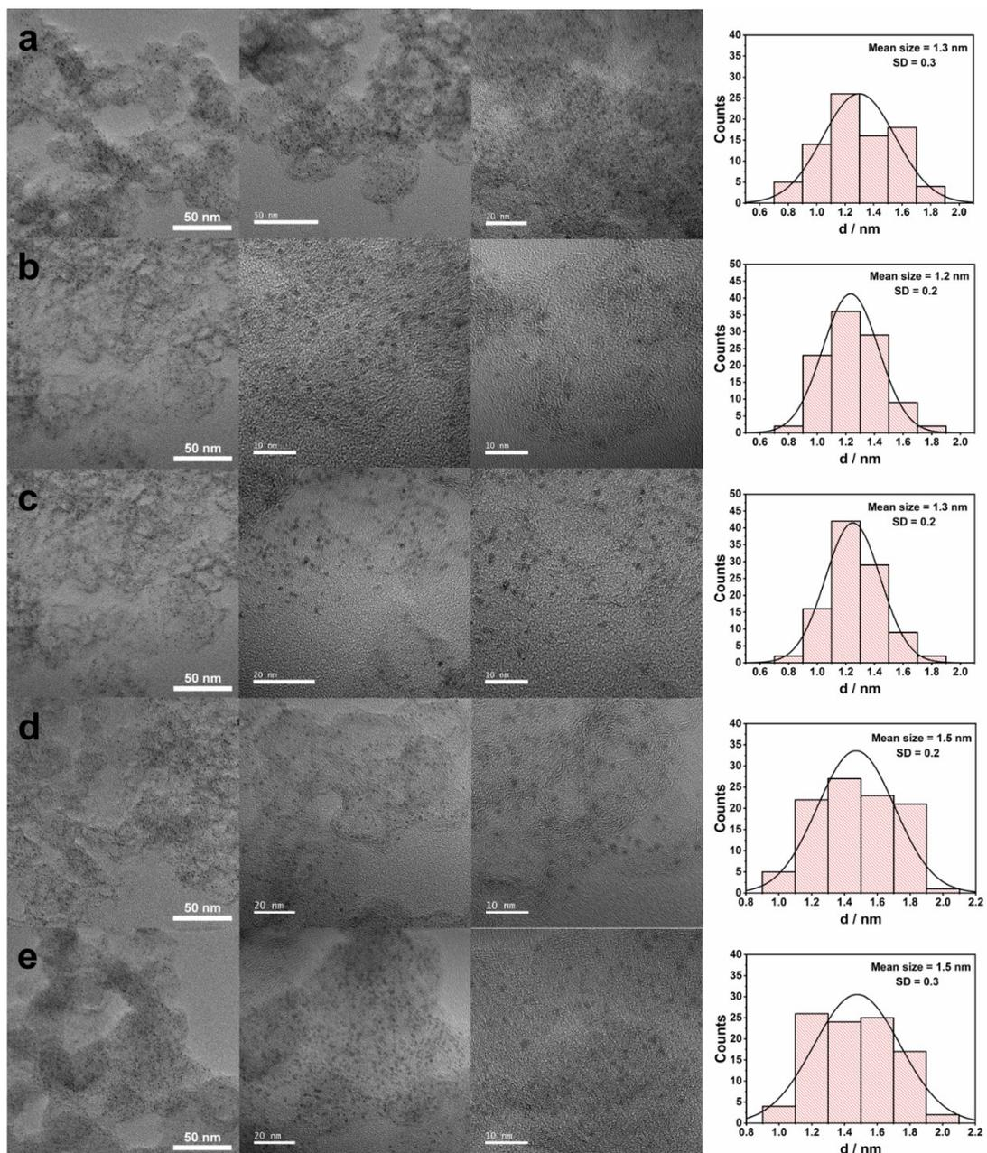
Fig. S8 TEM image and corresponding nanoparticle size distribution of (a) IrZn<sub>0.5</sub> (b) IrZn<sub>1</sub> (c) IrZn<sub>2</sub> (d) IrZn<sub>5</sub> and (e) IrZn<sub>10</sub>.
