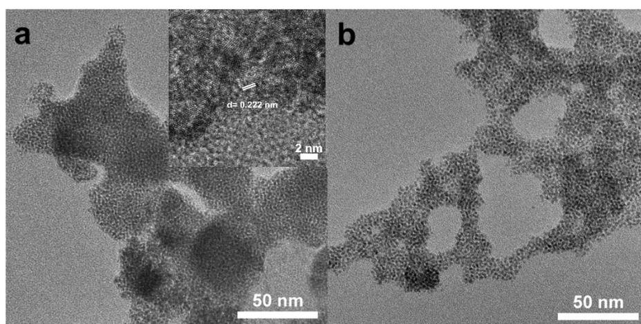
Fig. S2 (a) TEM and HRTEM images of metallic Ir and (b) TEM image of IrCd<sub>5</sub> synthesized without carbon black.
