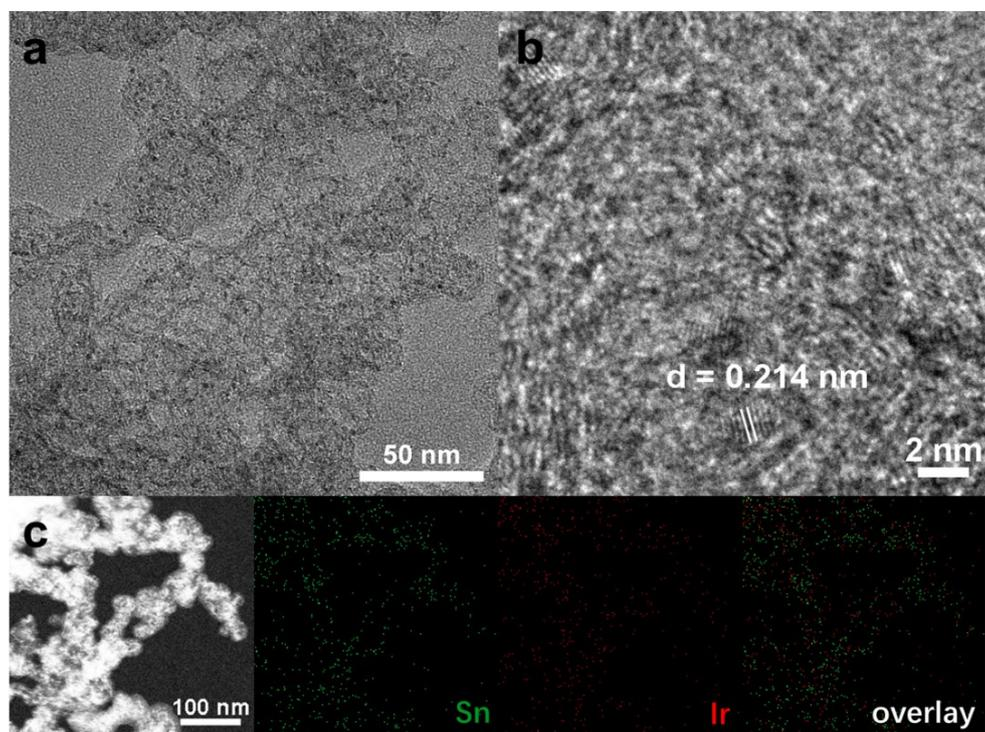
Fig. S11 (a) TEM (b) HRTEM image (c) HAADF-STEM-EDS element mappings of IrSn<sub>0.05</sub>.
