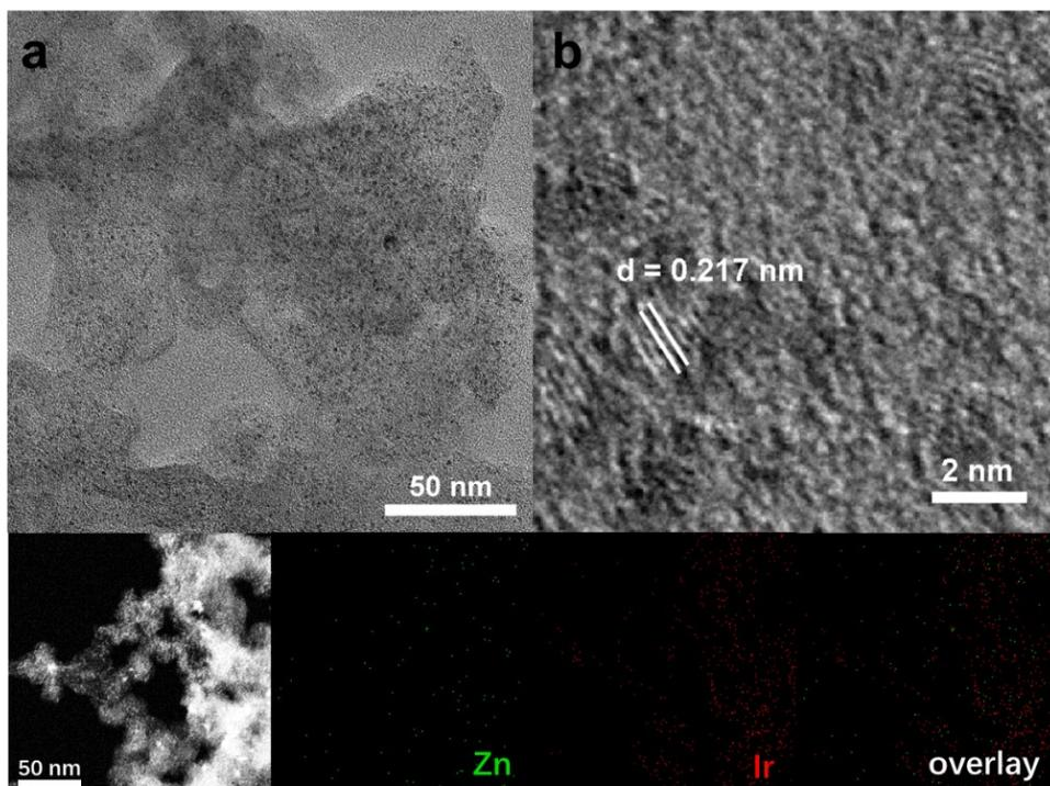
Fig. S12 (a) TEM (b) HRTEM image (c) HAADF-STEM-EDS element mappings of of IrZn<sub>10</sub>.
