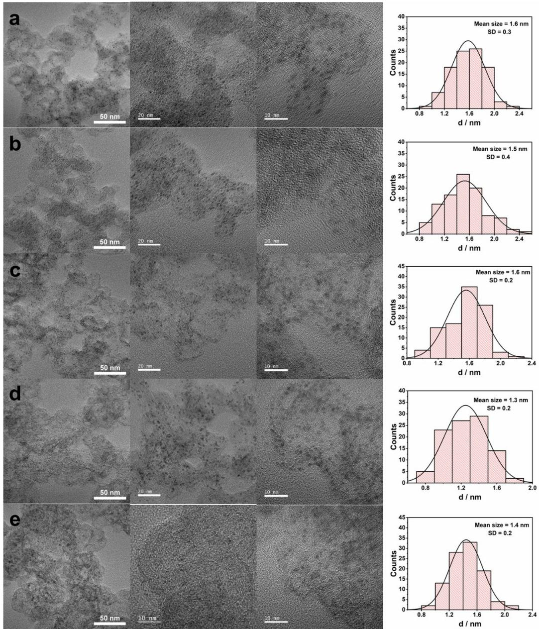
Fig. S6 TEM images and corresponding nanoparticle size distribution of (a) IrGa<sub>0.5</sub> (b) IrGa<sub>1</sub> (c) IrGa<sub>2</sub> (d) IrGa<sub>5</sub> and (e) IrGa<sub>10</sub>.
