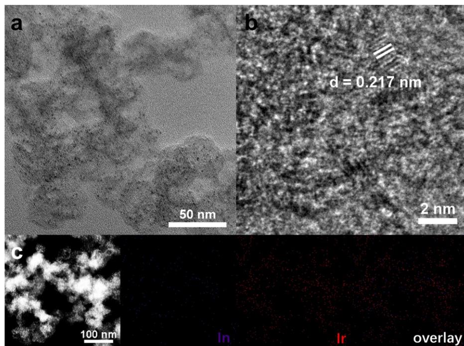
Fig. S13 (a) TEM (b) HRTEM image (c) HAADF-STEM-EDS element mappings of IrIn<sub>1</sub>.
