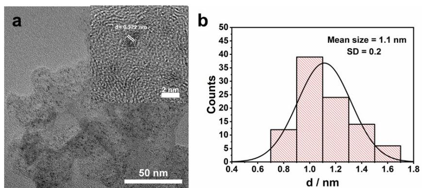
Fig. S1 (a) TEM and HRTEM image of Ir supported on CB and (b) corresponding nanoparticle size distribution of Ir.
