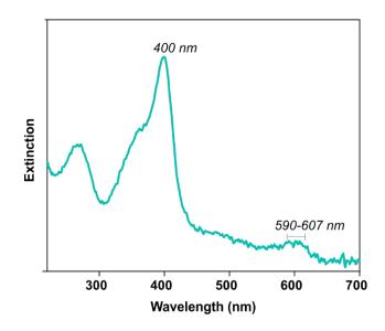
**Fig. S11** UV-vis absorption spectra of 10  $\mu$ M hemin solution (water-ethanol mixture). The UV-vis absorption spectra shows a main band at 400 nm and a broad band at around 590-607 nm that corresponds to the Soret band (B-band) and Q-band respectively which arises due to  $\pi$ -  $\pi$ \* transitions of the porphyrin ring modulated by the ferric ion.
