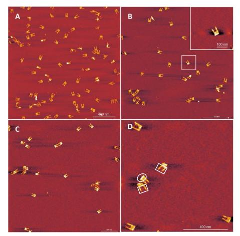
**Fig. S2** (**A-C**) AFM images of DNA origami nanofork samples with hemin bound to the bridge. (**D**) White rectangular boxes highlights the double stranded running bridge sequence in the forks and white circle highlights the extra rows of DNA double helices imparting support to the base of the nanofork.
