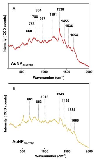
**Fig. S12** SERS spectra recorded from (A) (GTT)<sub>8</sub>-SH and (B) (TTT)<sub>8</sub>-SH coated Au NPs deposited on Si-wafer with 633 nm laser excitation source. (10 s, acc 20,  $50\times$ , 250 µW)
