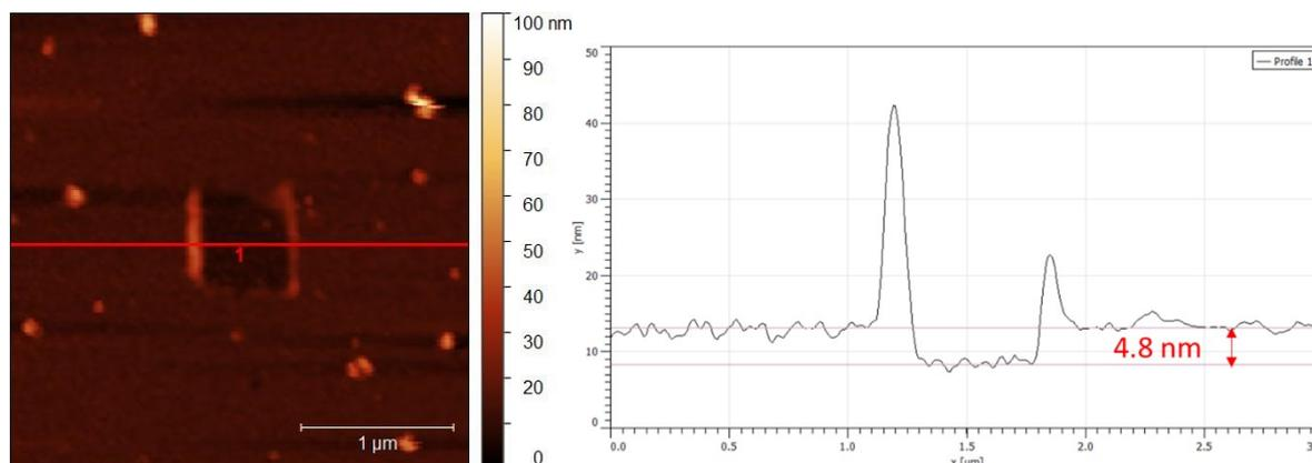
**Fig. S1** Determination of the polyscopoletin nanofilm thickness by local removal of the polymer from the gold surface in a rectangular area (left) to reveal the cross-section (right).
