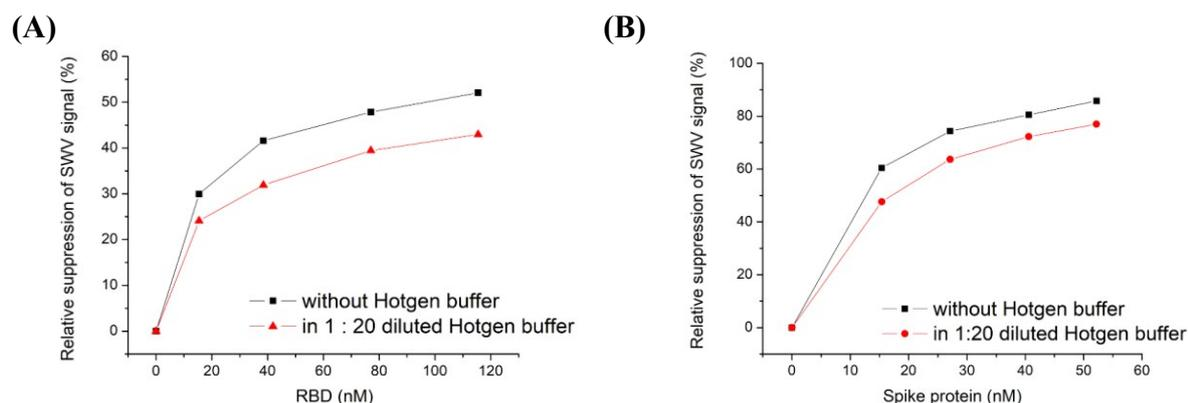
**Fig. S5** Comparison of binding of RBD (A) and spike protein (B) to the MIP measured in 5 mM  $\text{K}_3[\text{Fe}(\text{CN})_6]/\text{K}_4[\text{Fe}(\text{CN})_6]$  in PBS or 1:20 diluted Hotgen buffer.
