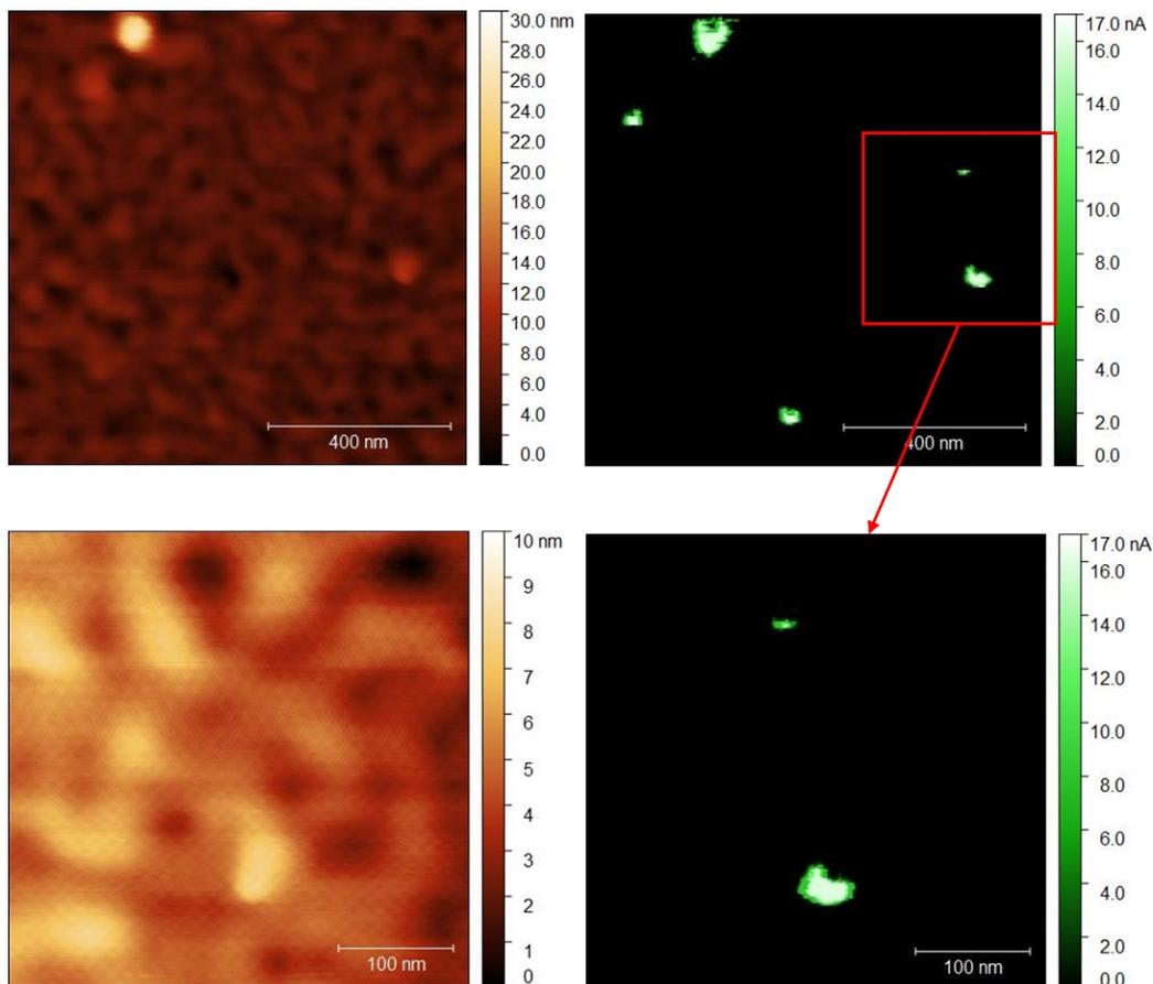
**Fig. S3** High resolution topographic and current maps of G-Peptide (5  $\mu\text{M}$ ) imprinted polyscopeletin nanofilms after template removal recorded by c-AFM.
