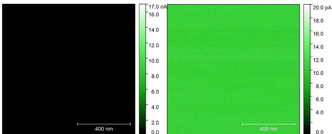
**Fig. S2** Current maps of the polyscopoletin film (NIP) by c-AFM in low (left) and high (right) current sensitivity mode that shows the excellent electrical insulating property of the film.
