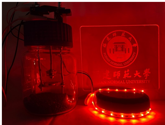
Fig. S18. Two batteries in series power the LED lights in a carbon dioxide atmosphere.
