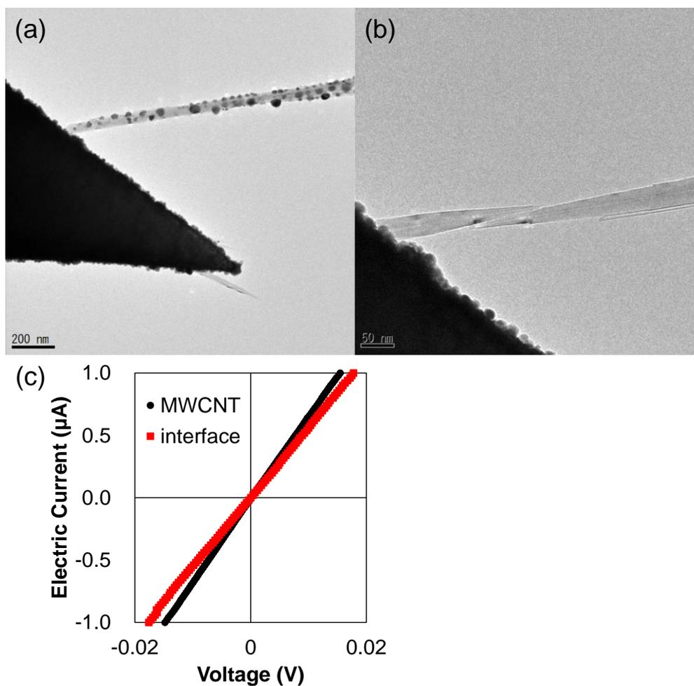
Fig. S4. Electrical resistance before and after cutting the multiwalled carbon nanotube (MWCNT). (a, b) Transmission electron microscopy images of (a) single MWCNT and (b) two MWCNTs connected by an interface. (c) Current–voltage relationships for the MWCNT without and with an interface, corresponding to the images shown in (a) and (b), respectively.
