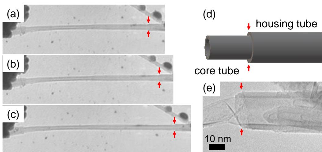
Fig. S3. TEM images and schematic of a telescoped MWCNT. (a, b, c) TEM images of the core tube extraction from the housing tube. (d) Schematic of the telescoped MWCNT. (e) TEM image of the housing tube after core tube extraction. Red arrows indicate the edge of the housing tube.
