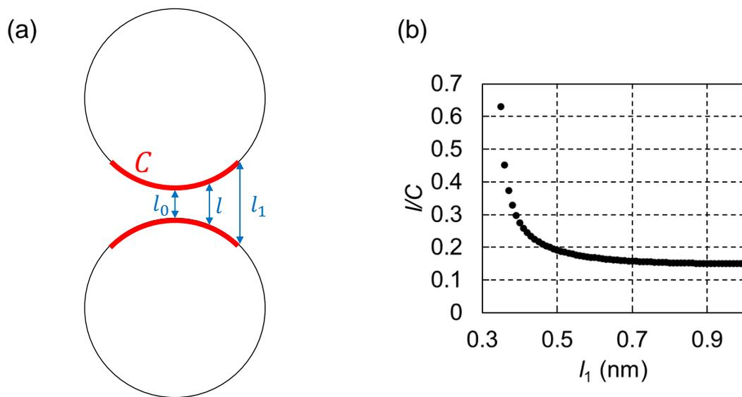
Fig. S1. Estimation of size factor of interfacial electrical resistance. (a) Schematic of the cross-sections of two adjacent multiwalled carbon nanotubes. (b) Size factor  $l/C$  as a function of  $l_1$ .
