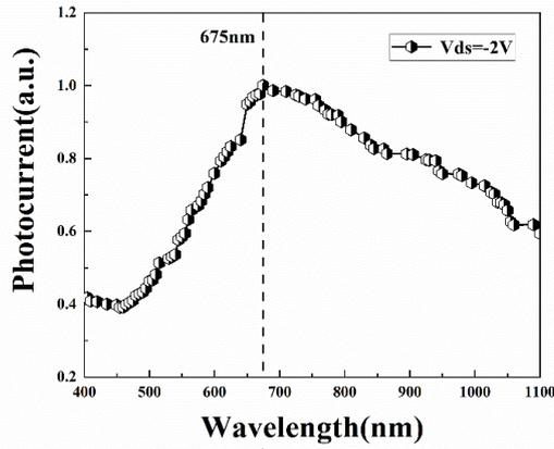
**Figure S13.** Wavelength-dependent relative responsivity of the device II at  $V_{ds} = -2$  V.
