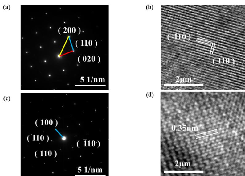
**Figure S8.** (a) selected area electron diffraction (SAED) pattern and (b)HRTEM image of the SnS nanosheet. (c) selected area electron diffraction (SAED) pattern and (d)HRTEM image of the InSe nanosheet.
