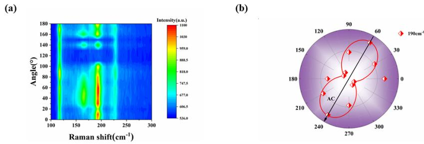
**Figure S20.** (a) Angle-resolved polarized Raman mapping of the device I as a function of polarization angle. b) Polar plots of Raman intensity with the Raman mode at  $190 \text{ cm}^{-1}$ , the pink line is the fitting curve.
