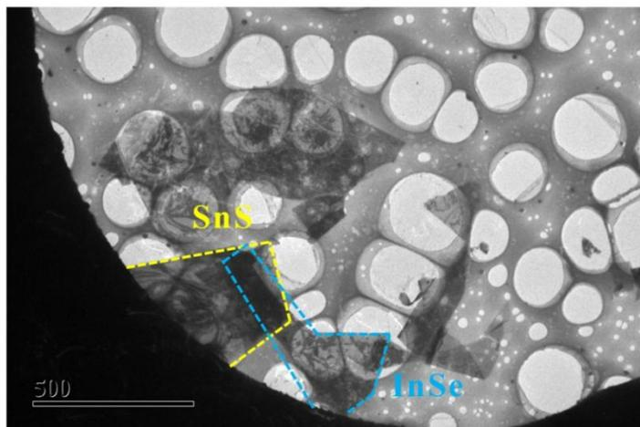
**Figure S9.** Low-resolution TEM image of the SnS / InSe heterojunction.
