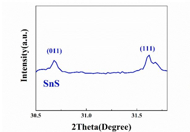
**Figure S7.** XRD patterns of SnS samples on SiO<sub>2</sub>/Si substrates.
