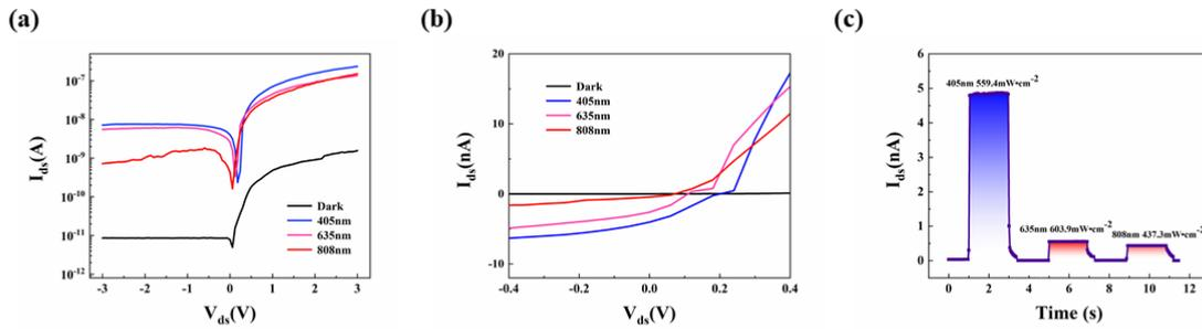
**Figure S12.** Logarithmic  $I_{ds}$ - $V_{ds}$  curves of the device I under the wavelengths of 405 nm, 635 nm and 808 nm under darkness conditions. (b) The enlarged  $I_{ds}$ - $V_{ds}$  curves of the device I under different wavelengths, showing the variation of the short circuit current ( $I_{sc}$ ) and the open circuit voltage ( $V_{oc}$ ). (c) Time-dependent photoresponse behavior of the the device I under different wavelengths at  $V_{ds} = 0$  V.
