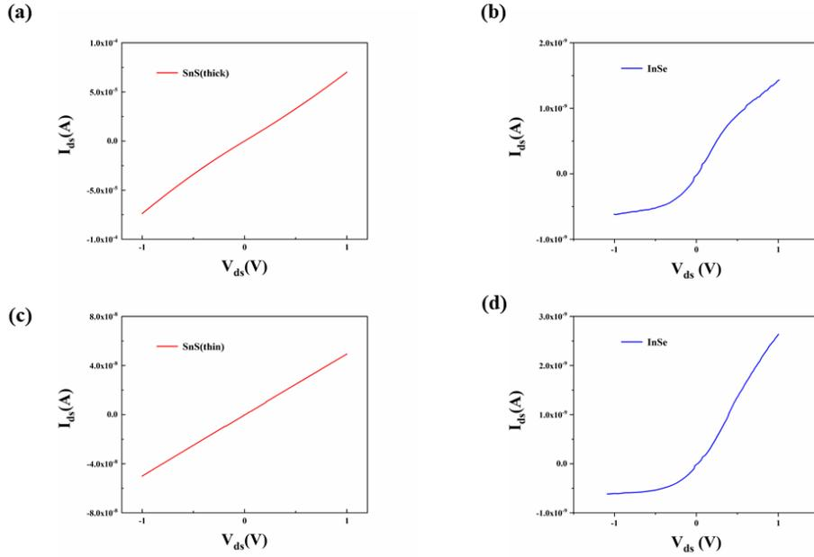
**Figure S11.** The electrical characteristics of individual FET. (a, b) the I-V curve of SnS(thick) and InSe of the device I under in dark conditions under ambient atmosphere, respectively. (c, d) the I-V curve of SnS(thin) and InSe of the device II under in dark conditions under ambient atmosphere, respectively.
