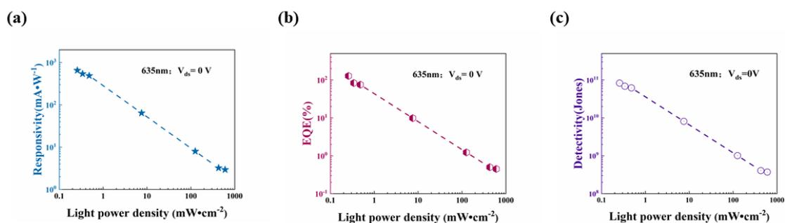
**Figure S18.** (a, b and c) Responsivity, EQE and detectivity of the device I as a function of light power density without bias.
