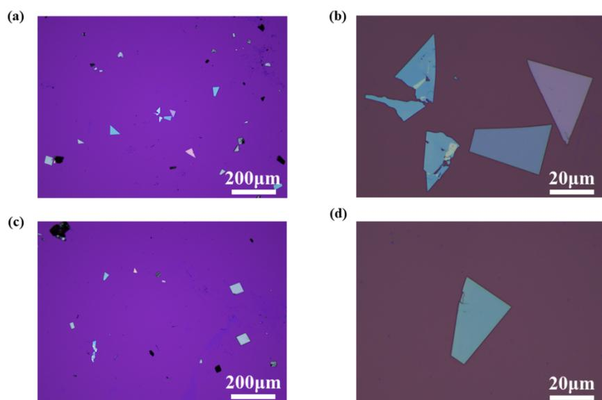
**Figure S1.** OM images of the SnS nanosheets prepared by LPPVD method. (a,c) OM images at the magnification of 10x.(b,d) OM images at the magnification of 100x.
