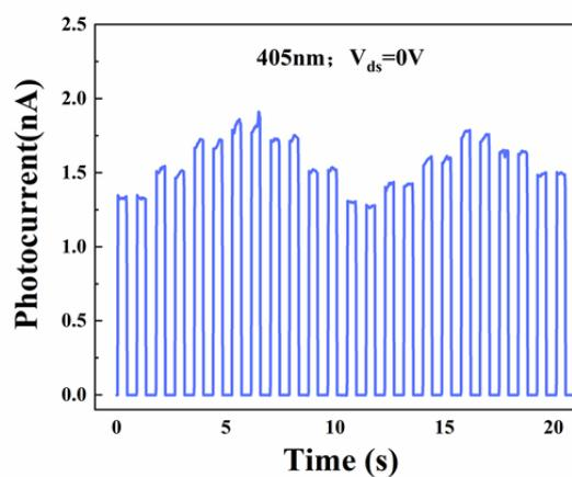
**Figure S19.** The time resolved photocurrent of the device II under polarized light with varying
