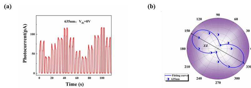
**Figure S21.** (a) The time resolved photocurrent of the device I under polarized light with varying polarization angle from  $30^\circ$  to  $360^\circ$  under 635 nm light power of 15.8 mW. (b) Polarizationsensitive photocurrent as a function of the polarization angle in the polar coordinates under linear-polarization laser of 635 nm at  $V_{ds} = 0 \text{ V}$ .
