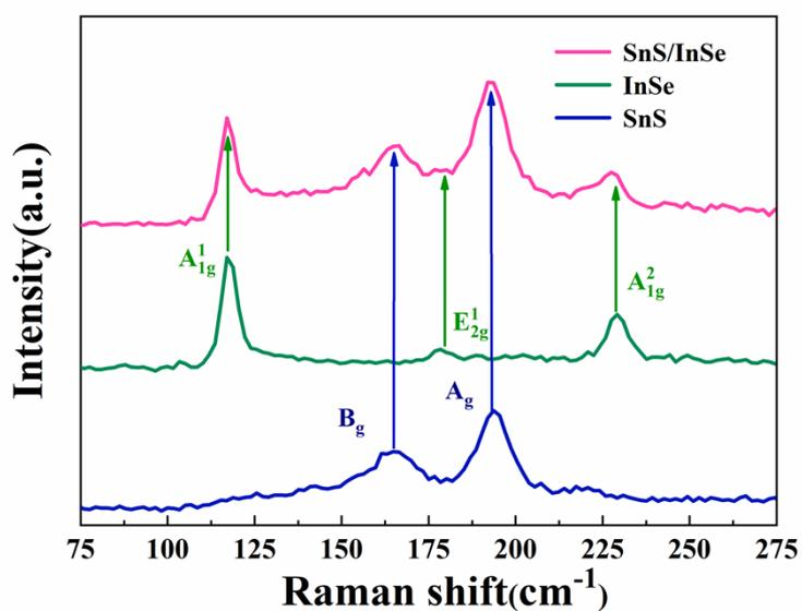
**Figure S2.** Raman Scattering spectra of individual SnS, InSe and their heterojunction for Device I.
