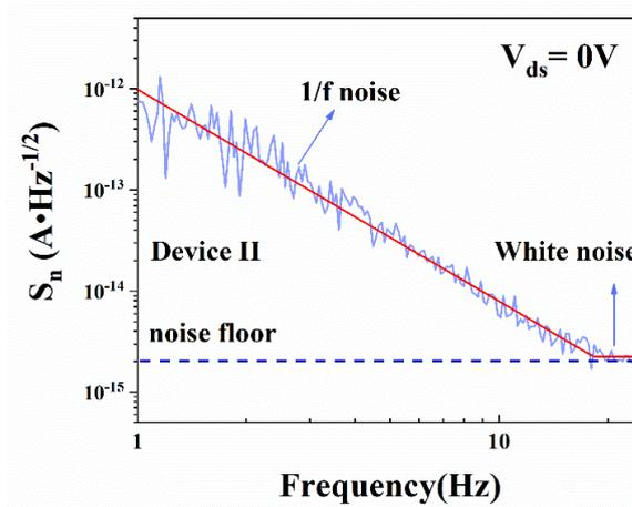
**Figure S15.** Noise spectral density ( $S_n$ ) as a function of frequency at  $V_{ds}=0$ V.
