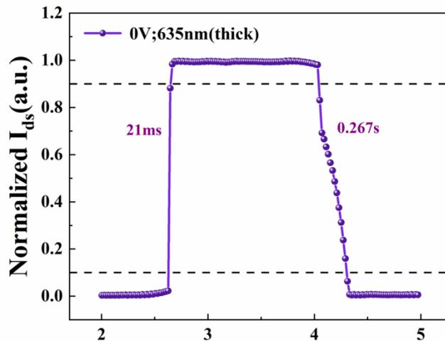
**Figure S16.** One cycle of the photoresponse of the device I to a wavelength of 635 nm at zero bias voltage for estimating both the rise and fall time.
