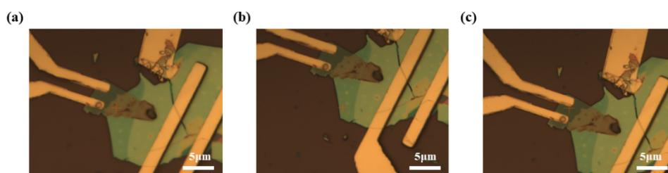
**Figure S5.** OM images for the device II in Photoluminescence measurement (Figure 1d). (a) OM image of the chosen InSe.(b) OM image of the chosen SnS/InSe heterojunction. (c) OM image of the chosen SnS. The red cross represents the measured spot.
