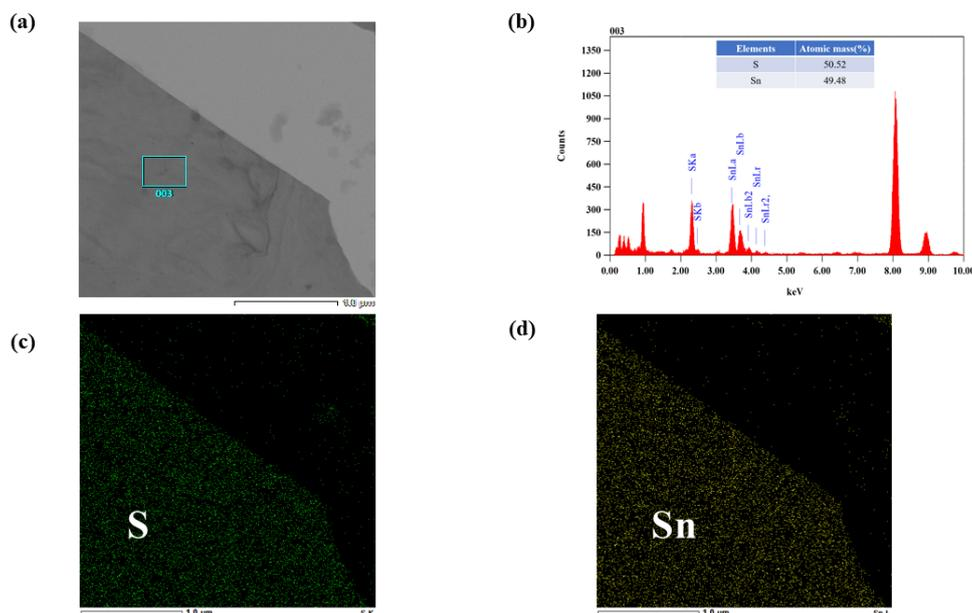
**Figure S6.** (a) HRTEM image and (b) The corresponding EDS spectrum and the extracted EDS data of SnS nanosheets in the blue square. (c,d) HRTEM EDS mapping of the elements S and Sn for the SnS nanosheet.
