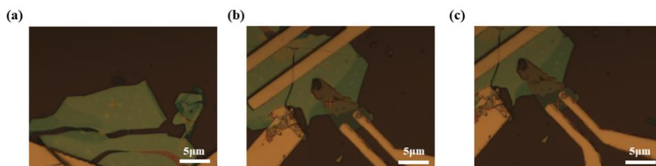
**Figure S3.** OM images for the device II in Raman spectra measurement (Figure 1c). (a) OM image of the chosen InSe.(b) OM image of the chosen SnS/InSe heterojunction. (c) OM image of the chosen SnS. The red cross represents the measured spot.
