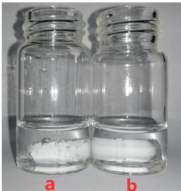
**Fig. S8** The decomposition of  $\text{NH}_4\text{HCO}_3$ . (a) At 45 °C. (b) At room temperature.
