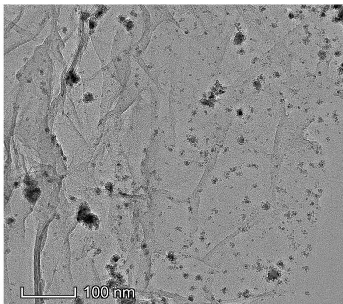
**Fig. S2** TEM image of Pd-CeO<sub>2-x</sub>/FGS after 500 cycles CV scans.
