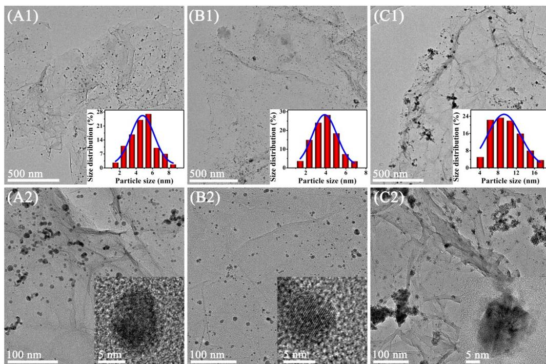
**Fig. S1** TEM images of Pd/GS (A1, A2), Pd/FGS (B1, B2) and Pd-CeO<sub>2-x</sub>/GS (C1, C2). The insets are HRTEM images and the corresponding particle size statistical charts.
