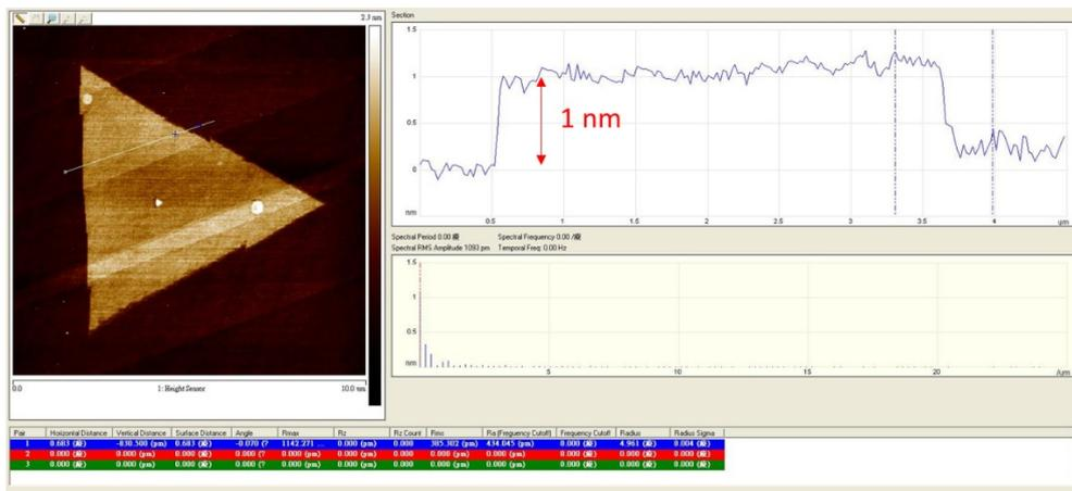
**Figure S5.** AFM image of Cr:WS<sub>2</sub>. The height of the Cr:WS<sub>2</sub> is about 1 nm and the surface is uniform without extra layer grown on the surface after the ORC reaction.
