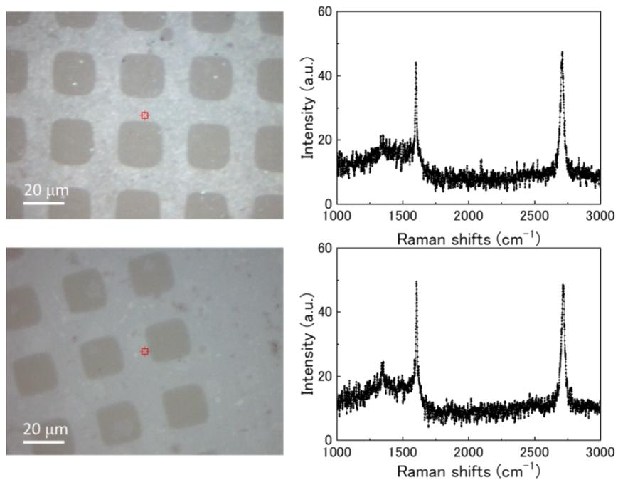
**Figure S3.** Optical images and corresponding Raman spectra of the single layer graphene mask after the ORC reaction.
