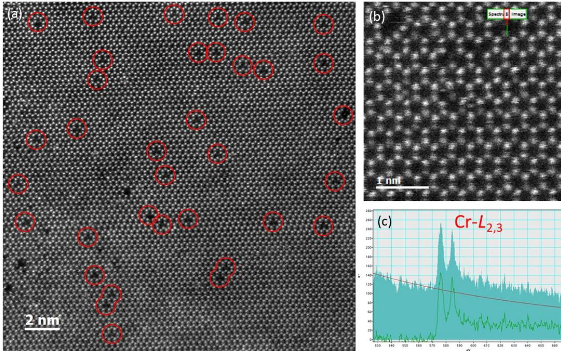
**Figure S1.** (a) STEM-ADF image of Cr:WSe<sub>2-x</sub> with Se flow to repair the Se vacancies through ORC reaction. The Cr substitutional dopants are highlighted by red circles. (b) Magnified STEM-ADF image of Cr:WSe<sub>2</sub>. The atom-by-atom EELS line scan is performed along the green line. (c) EELS profile of Cr L<sub>2</sub>, L<sub>3</sub> edges extracted from the EELS line scan.
