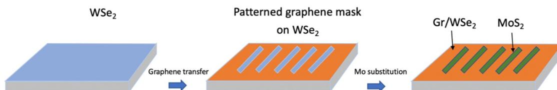
**Figure S7.** To make lateral heterostructures, graphene is used as the mask and transferred onto a monolayer WSe<sub>2</sub> film. The exposed WSe<sub>2</sub> areas allow for ORC reaction. After the ORC reaction with the supply of Mo and S precursors, the exposed WSe<sub>2</sub> stripes can be nearly converted into MoS<sub>2</sub>.
