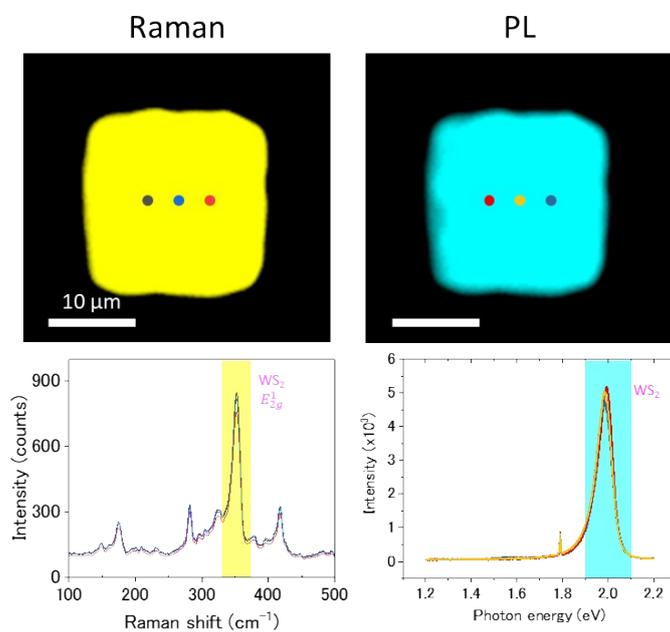
**Figure S4.** Raman and PL mapping of the unmasked region where the  $\text{WSe}_2$  was transformed into  $\text{Cr:WS}_2$  completely after the ORC reaction. The Raman and PL mappings were plotted regarded to the integrated  $\text{WS}_2 E_{2g}^1$  peak ( $325\sim 275 \text{ cm}^{-1}$ ) and the
