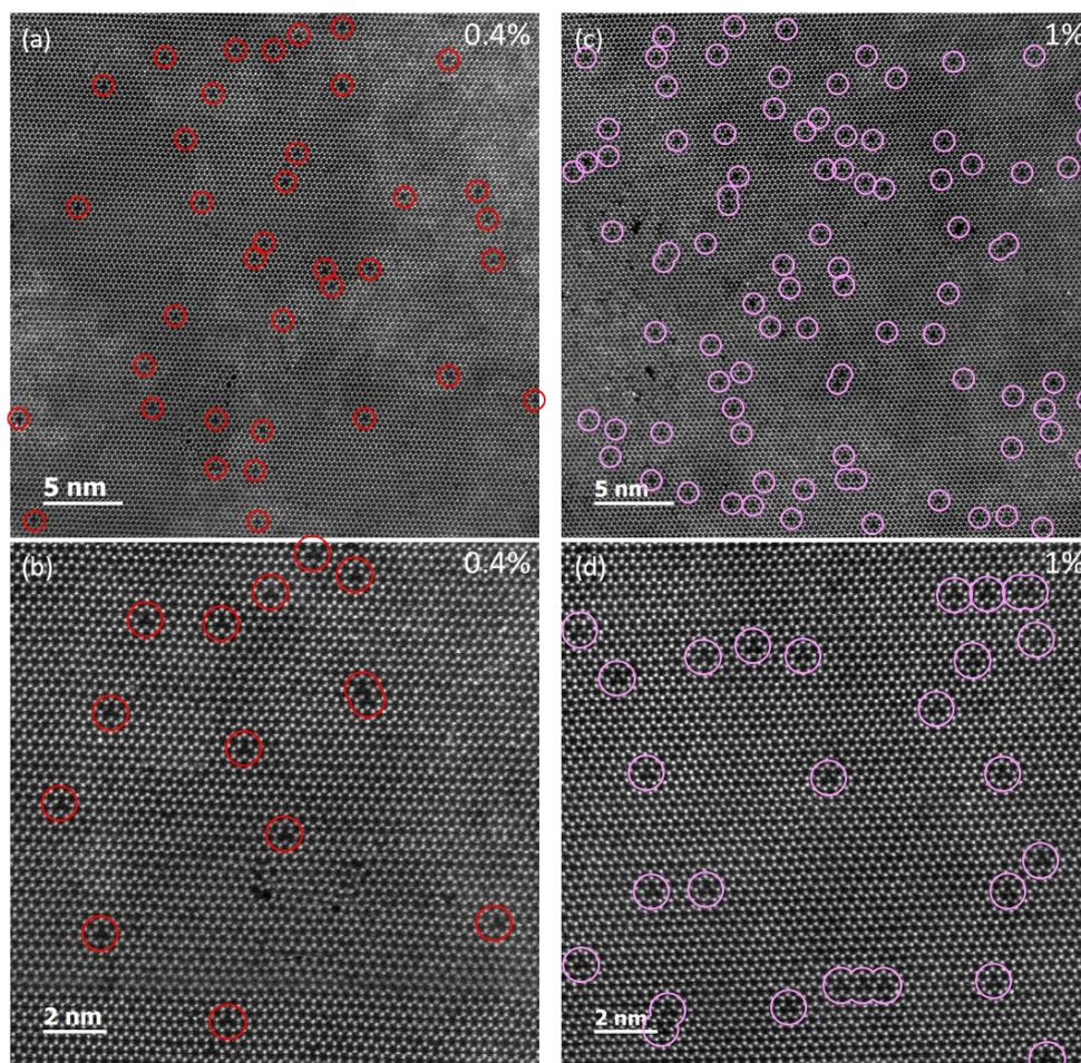
**Figure S6.** (a,b) STEM images of 0.4% Cr-doped WSe<sub>2</sub> at different magnifications. (c,d)
