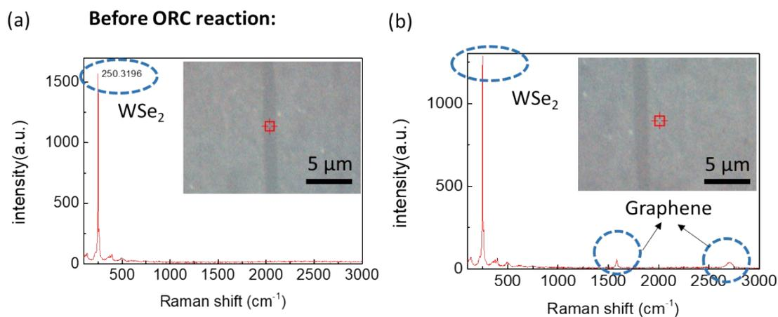
**Figure S8.** Raman spectra before the ORC reactions with the supply of Mo and S precursors. (a) Raman spectrum acquired on the area of exposed WSe<sub>2</sub>. (b) Raman spectra acquired on the area of Gr/WSe<sub>2</sub>. The figure insets in (a) and (b) show the optical microscopy image of the patterned Gr mask on WSe<sub>2</sub>.
