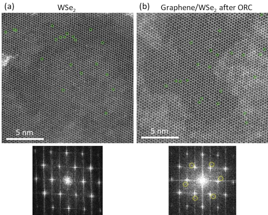
**Figure S2.** (a) STEM and corresponding FFT image of pristine WSe<sub>2</sub>. Se vacancies are marked with green circles. (b) STEM and corresponding FFT image of WSe<sub>2</sub> covered with graphene after the ORC process. The yellow circles in the FFT image are contributed from the graphene lattice covered on WSe<sub>2</sub>.
