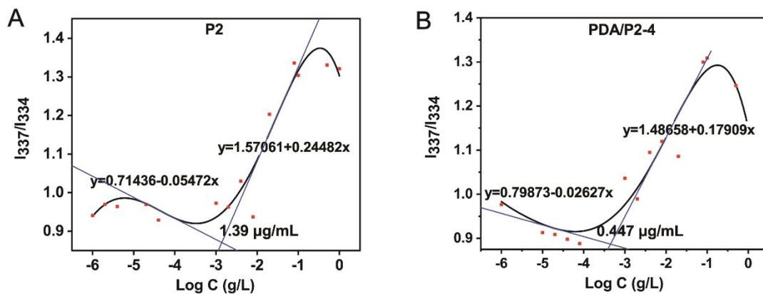
**Figure S6.** CMC values of P2 and PDA/P2-4 polymers.
