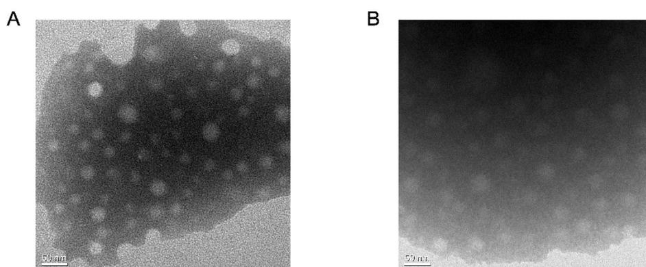
**Figure S5.** The TEM images of P2 (A) and PDA/P2-4 (B), the particle size of P2:  $24.30 \pm 2.78$  nm, the particle size of PDA/P2-4:  $29.53 \pm 2.37$  nm,  $n = 30$ . (Stained with 3% phosphotungstic acid solution for 30 s)
