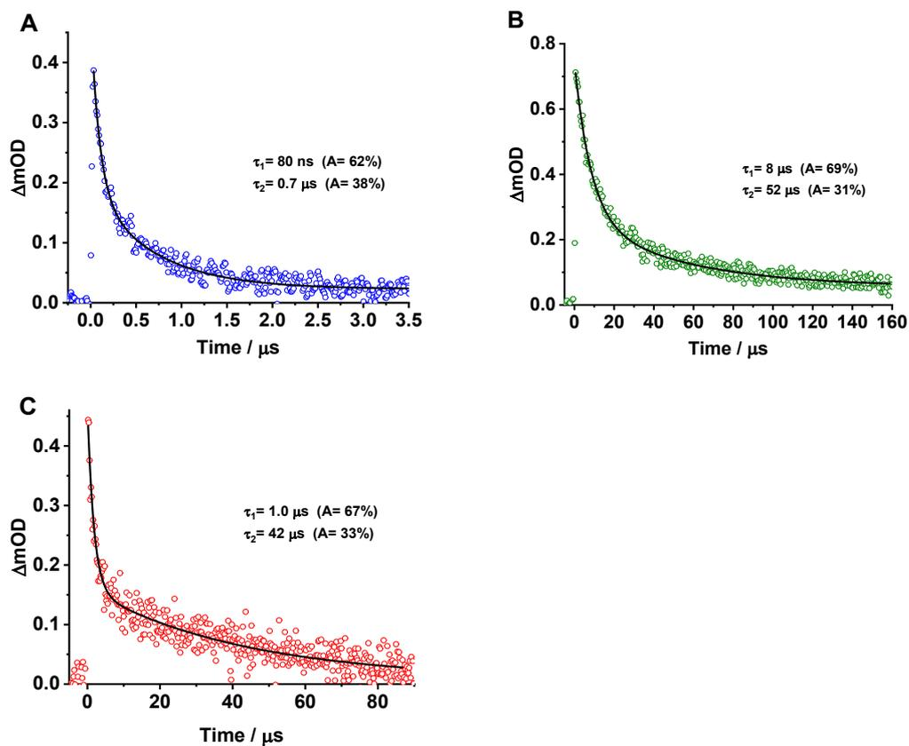
**Figure S7.** Laser flash photolysis decays at 470 nm for A) CuS (EDA) NCs, B) CuS/CdS (EDA) HNCs and C) CuS/CdS (EDT) HNCs following excitation at 1100 nm. The solid line represents the best bi-exponential fit. Note the difference in the timescales.
