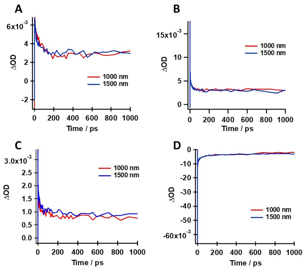
**Figure S6.** Comparison of the transient decays at: A) 440 nm; B) 560 nm; C) 640 nm and D) 900 nm probe wavelengths of thin films of CuS (EDA) NCs at long time window following excitation at 1000 and 1500 nm. The excitation power was 2 mW and the IRF is 80 fs.
