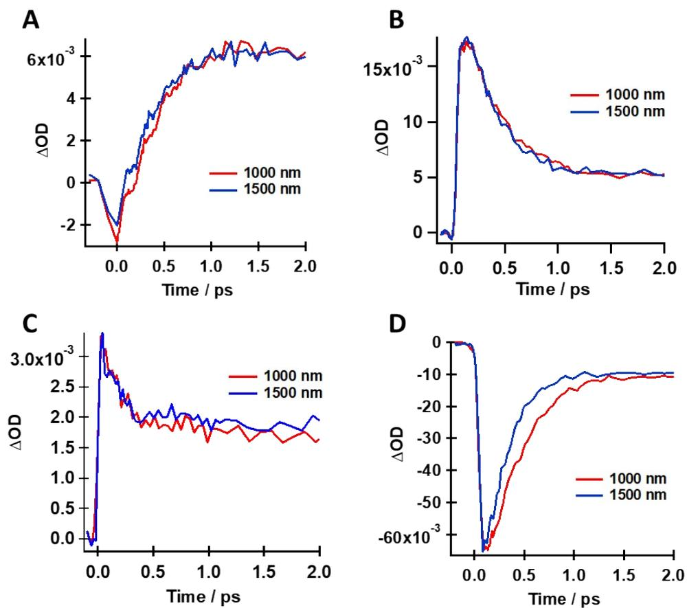
**Figure S5.** Comparison of the transient decays at: A) 440 nm; B) 560 nm; C) 640 nm and D) 900 nm probe wavelengths of thin films of CuS (EDA) NCs at short time window following excitation at 1000 and 1500 nm. The excitation power was 2 mW and the IRF is 80 fs.
