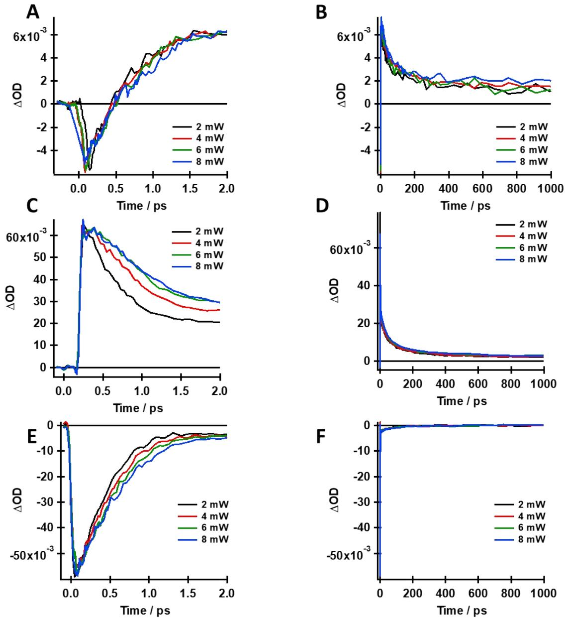
**Figure S13.** Comparison of the transient decays at A) and B) 440 nm; C) and D) 560 nm; and E) and F) 900 nm probe wavelengths at short and long time windows of thin films of CuS/CdS (EDA) HNCs following excitation at 1500 nm using different excitation power. The IRF is 80 fs.
