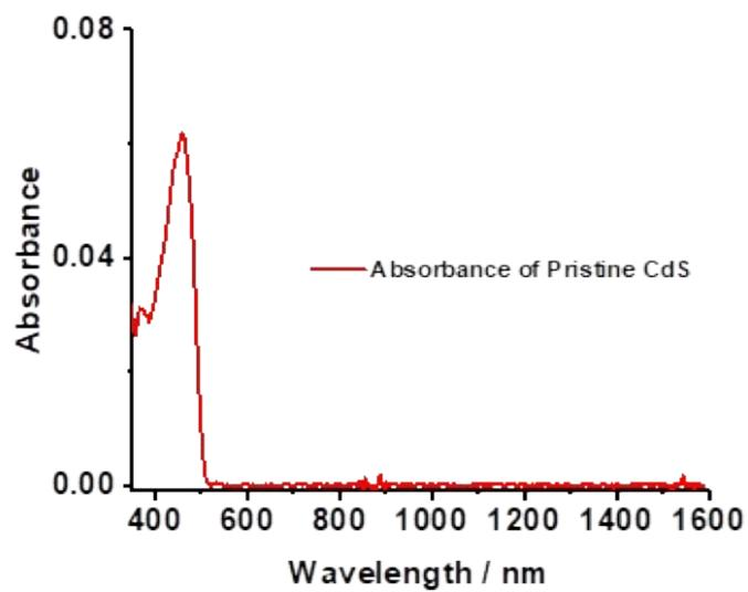
**Figure S11.** Absorption spectrum of pristine CdS. For more clarity, we have corrected the light dispersion of this sample by subtracting the baseline.
