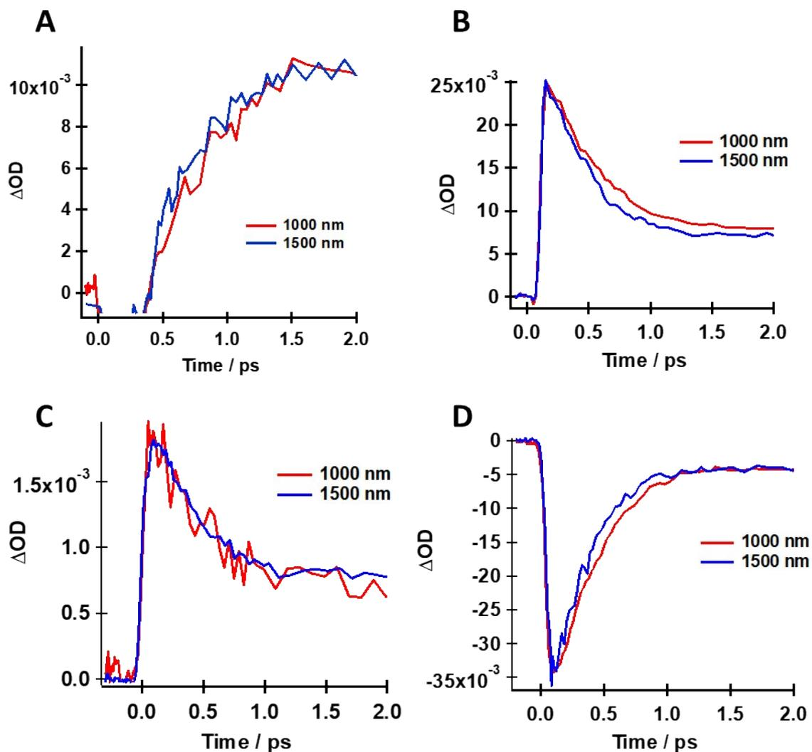
**Figure S9.** Comparison of the transient decays at: A) 440 nm; B) 560 nm; C) 640 nm and D) 900 nm probe wavelengths of thin films of CuS/CdS (EDA) HNCs at short time window following excitation at 1000 and 1500 nm. The excitation power was 2 mW and the IRF is 80 fs.
