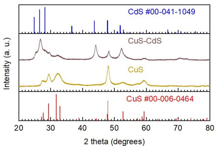
**Figure S3.** Powder X-ray diffraction (PXRD) patterns of CuS NCs and CdS/CuS HNCs, compared with the reference obtained for *cv*-CuS (JCPDS no 00-006-0464), and *w*-CdS (JCPDS no. 00-041-1049).
