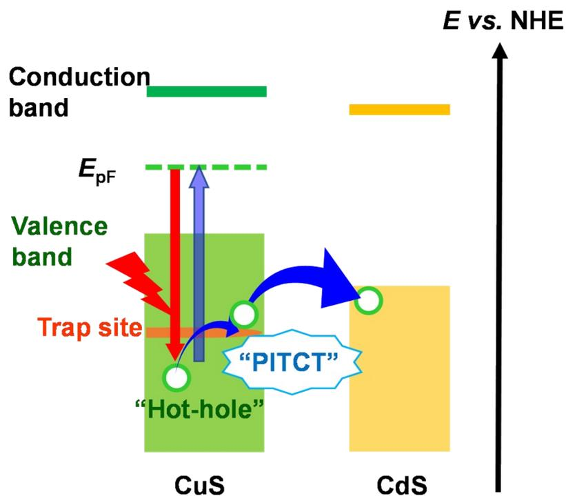
**Scheme S1.** Schematic presentation of the plasmon induced transit hole transfer (PITCT) mechanism. The hot hole transfer proceeds through a two-step process of hole trapping followed by transfer of the trapped holes to the acceptor phase.
