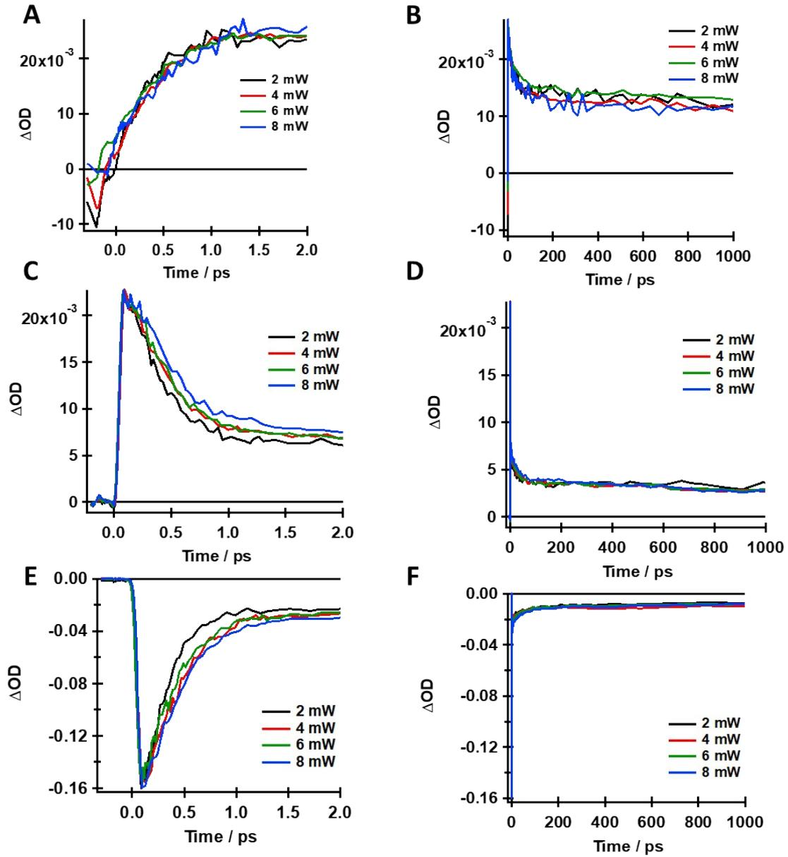
**figure S12.** Comparison of the transient decays at A) and B) 440 nm; C) and D) 560 nm; and E) and F) 900 nm probe wavelengths at short and long time windows of thin films of CuS (EDA) NCs following excitation at 1500 nm using different excitation power. The IRF is 80 fs.
