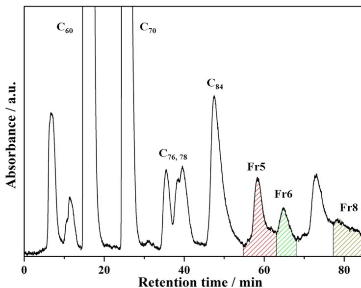
**Fig. S1** Isolation scheme of the fullerene extract on a Buckyprep column. Conditions: 20 mL injection volume; 10 mL/min toluene flow; 330 nm detecting wavelength.
