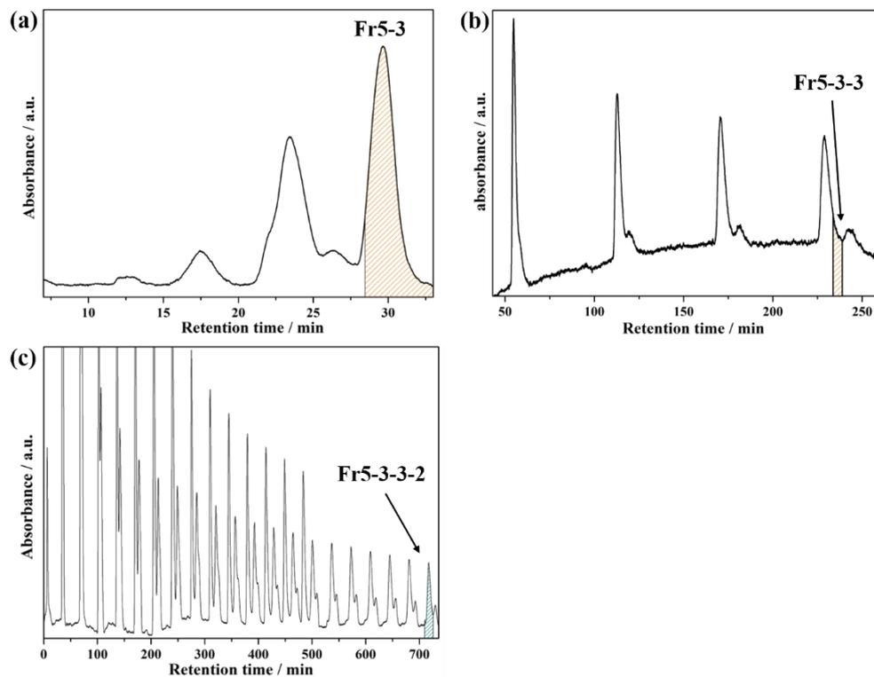
**Fig. S4** Isolation schemes of  $\text{Lu}_3\text{N}@D_{3h}(5)\text{-C}_{78}$ . (a) HPLC chromatogram of Fr5 on a Buckyrep-M column. Conditions: 20 mL injection volume; 10 mL/min toluene flow. (b) Recycling HPLC chromatogram of Fr5-3 on a Buckyrep column. Conditions: 20 mL injection volume; 10 mL/min toluene flow. (c) Recycling HPLC chromatogram of Fr5-3-3 on a Buckyrep column. Conditions: 5 mL injection volume; 4 mL/min toluene flow. (All of the detection wavelengths are 330 nm.)
