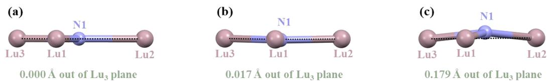
**Fig. S8** Drawings showing the planarity of Lu<sub>3</sub>N cluster in (a)  $C_s(17490)$ -C<sub>76</sub> and (b)  $C_2(22010)$ -C<sub>78</sub>, and the deviation of the Lu<sub>3</sub>N unit from planarity in (c)  $D_{3h}(5)$ -C<sub>78</sub>.
