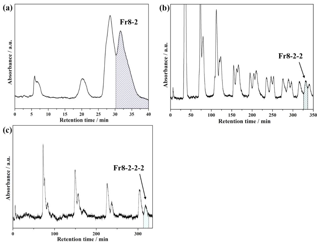
**Fig. S3** Isolation schemes of  $\text{Lu}_3\text{N}@C_2(22010)\text{-C}_{78}$ . (a) HPLC chromatogram of Fr8 on a Buckyrep-M column. Conditions: 20 mL injection volume; 10 mL/min toluene flow. (b) Recycling HPLC chromatogram of Fr8-2 on a Buckyrep-M column. Conditions: 15 mL injection volume; 10 mL/min toluene flow. (c) Recycling HPLC chromatogram of Fr8-2-2 on a Buckyrep column. Conditions: 115 mL injection volume; 10 mL/min toluene flow. (All of the detection wavelengths are 330 nm.)
