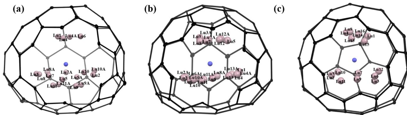
**Fig. S5** Positions of the disordered lutetium sites in (a)  $\text{Lu}_3\text{N}@C_s(17490)\text{-C}_{76}$ , (b)  $\text{Lu}_3\text{N}@C_2(22010)\text{-C}_{78}$ , and (c)  $\text{Lu}_3\text{N}@D_{3h}(5)\text{-C}_{78}$  relative to the cage orientation. The Lu sites labeled with “A” are generated by crystallographic operation and a part of the cages are omitted for clarity.
