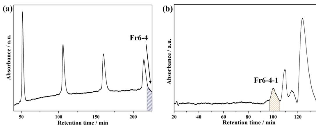
**Fig. S2** Isolation schemes of  $\text{Lu}_3\text{N}@C_s(17490)\text{-C}_{76}$ . (a) Recycling HPLC chromatogram of Fr6 on a Buckyprep column. Conditions: 15 mL injection volume; 10 mL/min toluene flow. (b) HPLC chromatogram of Fr6-4 on a 5PBB column. Conditions: 10 mL injection volume; 10 mL/min toluene flow. (All of the detection wavelengths are 330 nm.)
