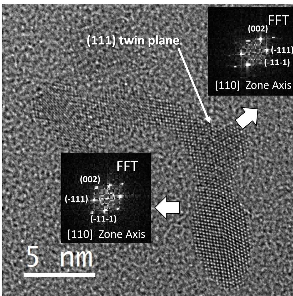
Figure S4. HRTEM image showing the presence of a  $\{111\}$  twin plane on a nano-object obtained after 8 h of reaction.
