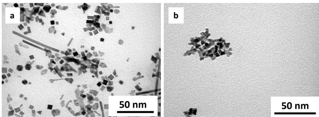
**Figure S14.** Influence of the reaction temperature. (a) 16 h at 40 °C. (b) 4 days at 10 °C.
