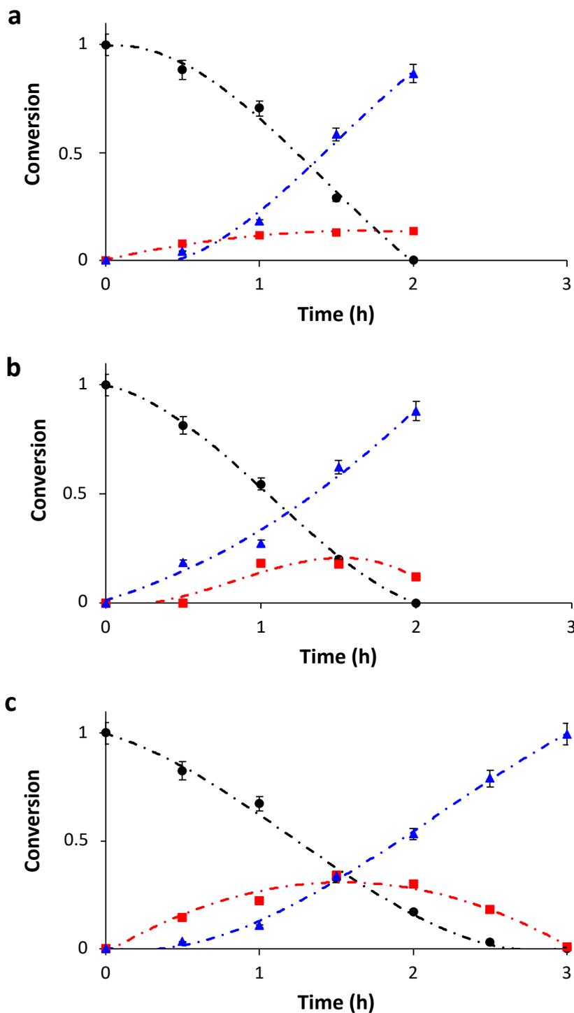
**Figure S18.** Results of PhA hydrogenation on Pt/C catalysts modified or not with ODA. (a) Pt/C catalyst without additional ODA. (b) Pt-ODA1/C catalyst containing 20%w/w ODA related to Pt. (c) Pt-ODA2/C catalyst containing 20%w/w ODA related to Pt/C, (black circles PhA, red squares ST, and blue triangles EB).
