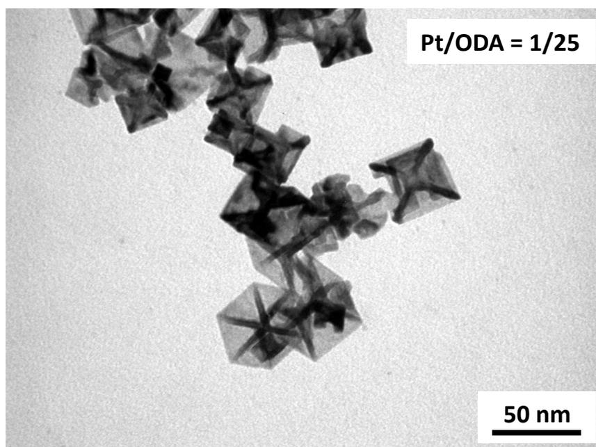
**Figure S1.** Concave nanocubes obtained by reduction of  $\text{PtCl}_2$  in the presence of ODA at 20 °C under 3 bar  $\text{H}_2$  (7 days reaction).
