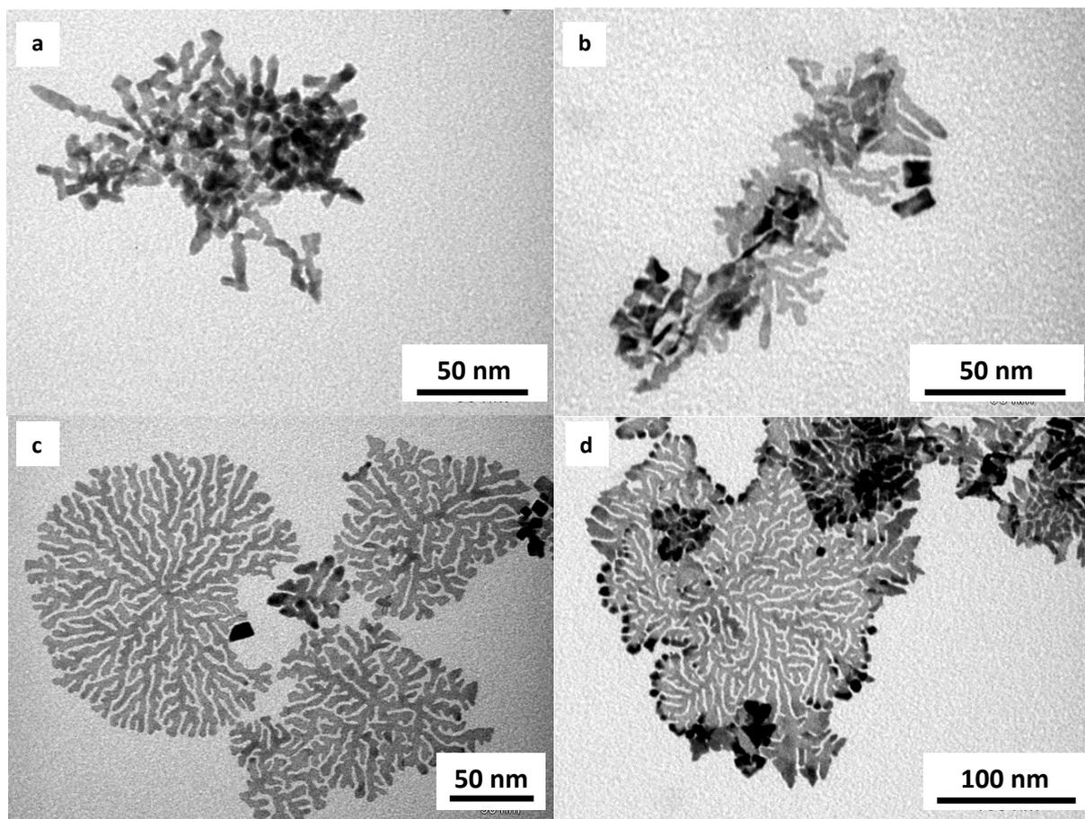
**Figure S7.** Time dependent evolution of the Pt UMNS. (a) 24 h reaction. (b) 48 h reaction; (c) 4 days reaction. (d) 7 days reaction.
