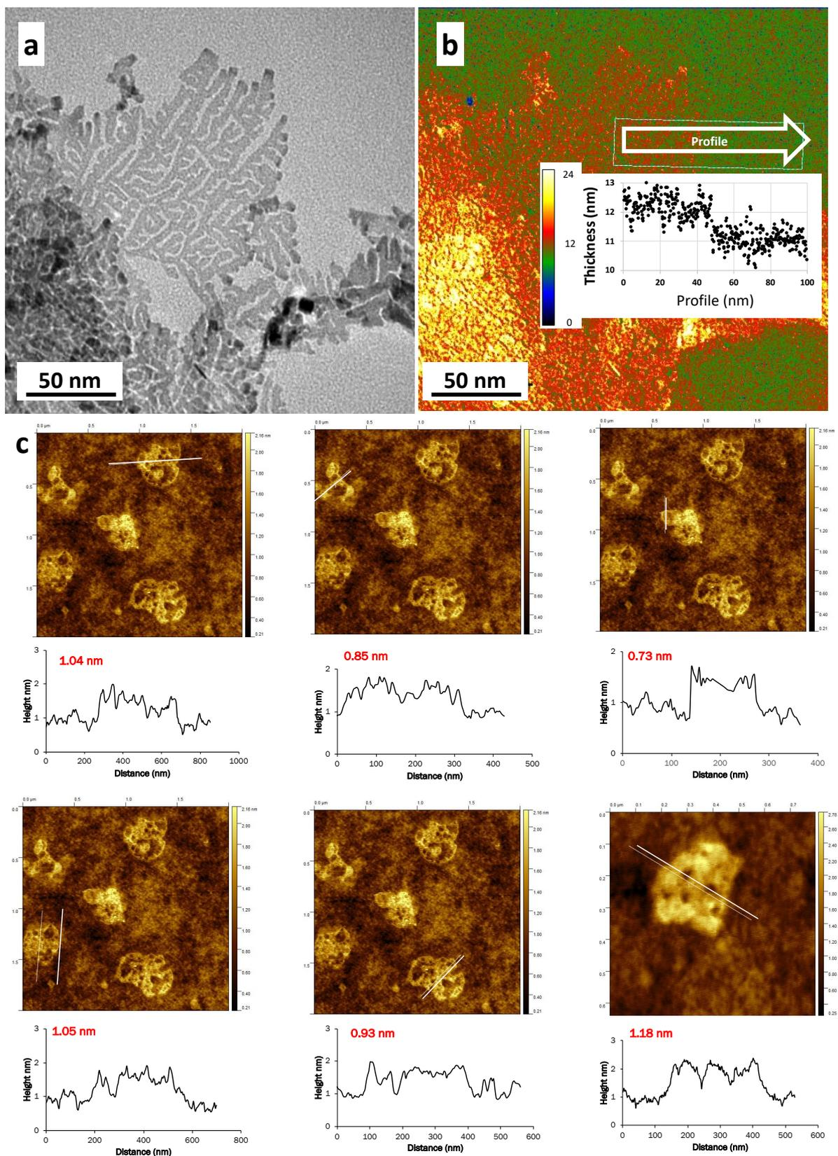
**Figure S8.** UMNS thickness. (a) TEM image of a Pt UMNS. (b) the corresponding thickness profile along line designated by the white arrow obtained through EFTEM. Point scattering is due to an average measurement of the thickness over all the pixels of the width of the
