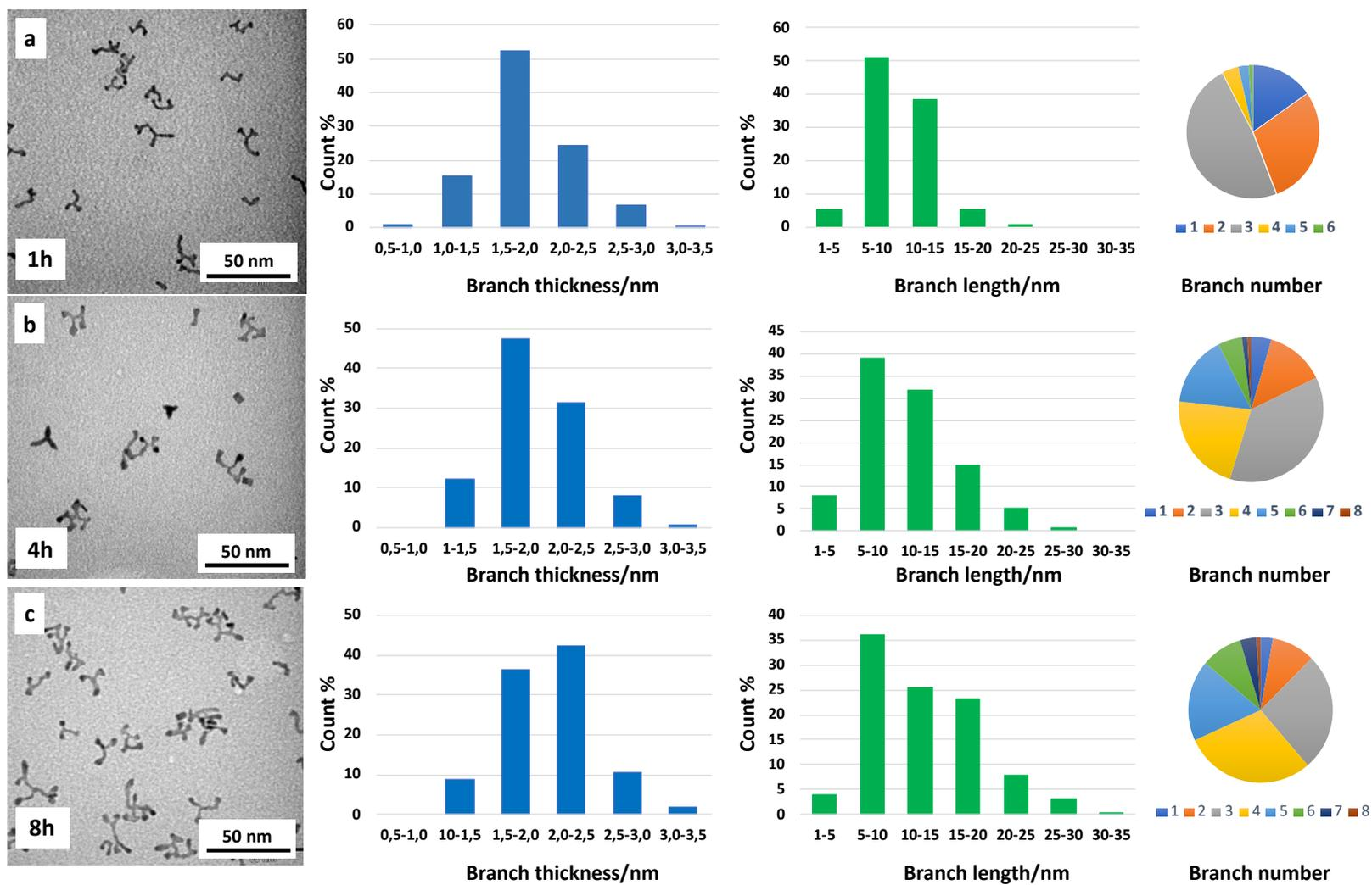
**Figure S2.** Time dependent evolution of the Pt multipods. (a) 1 h reaction. (b) 4 h reaction. (c) 8 h reaction.
