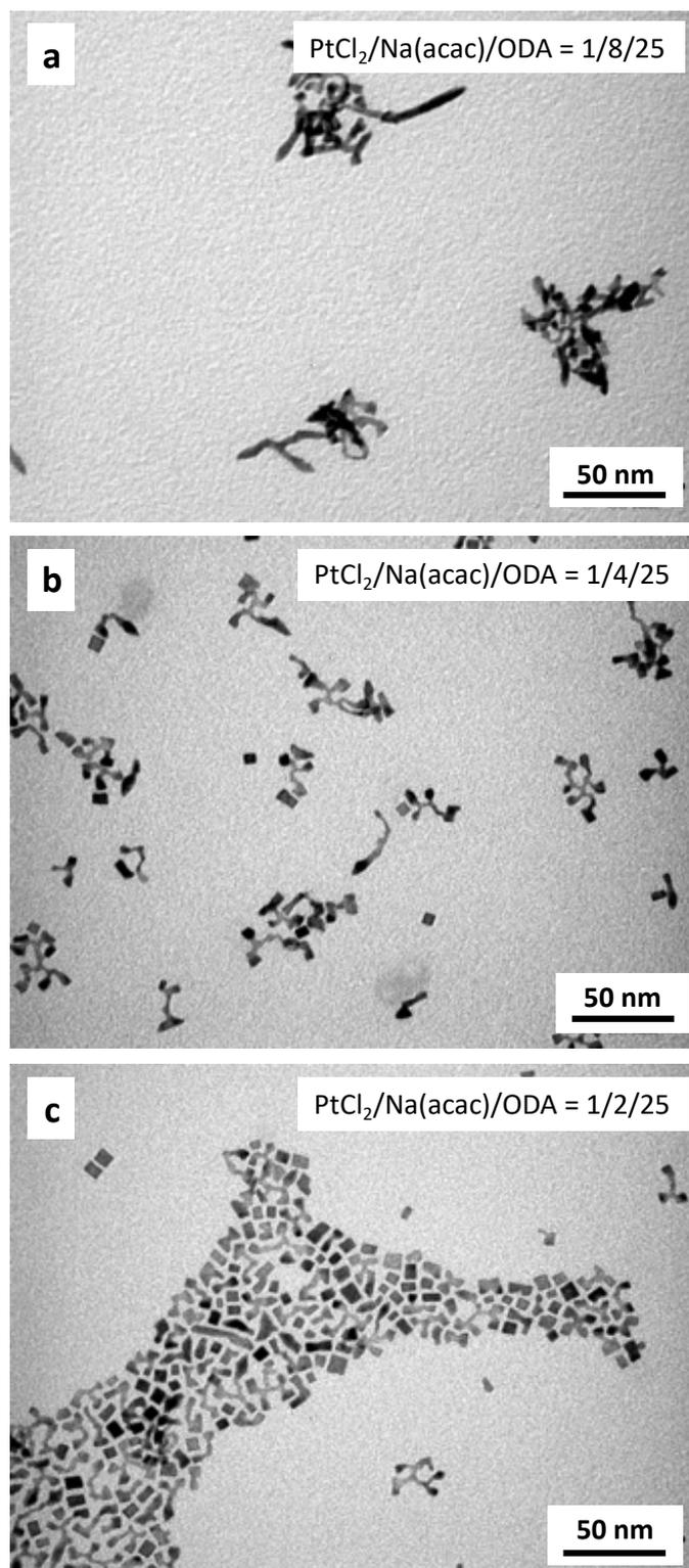
**Figure S13.** PtCl<sub>2</sub>/Na(acac)/ODA influence on the formation of dendritic multipods. All the results correspond to 24 h reaction at 20 °C. Pt Cl<sub>2</sub>/Na(acac)/ODA: (a) 1/8/25 (reference conditions); (b) 1/4/25; and (c) 1/2/25.
