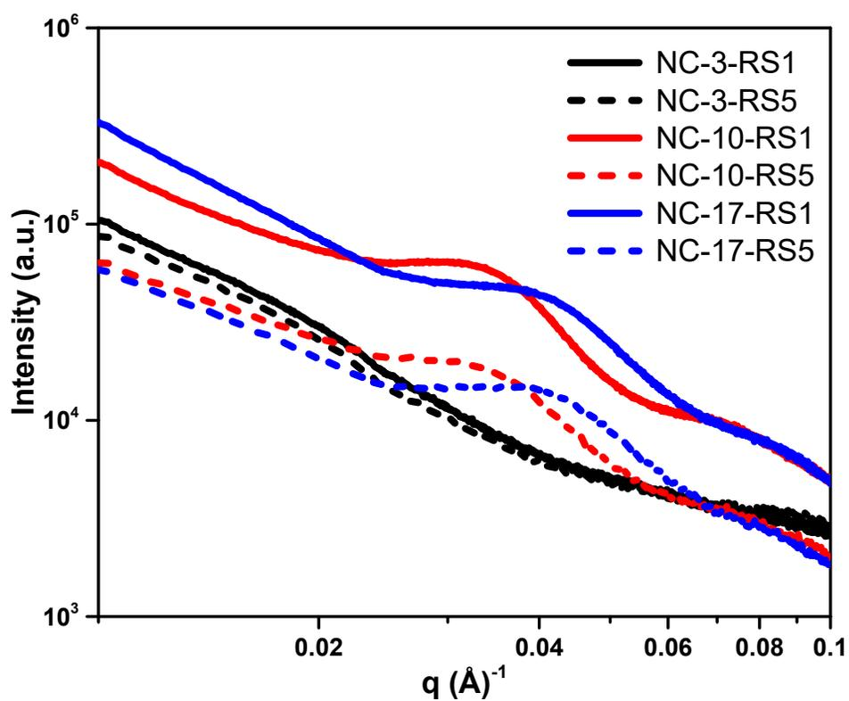
**Figure S4** Small angle X-ray scattering (SAXS) for NC-PNIPAM hydrogels after one and five reswelling, denoted as RS1 and RS5, respectively.
