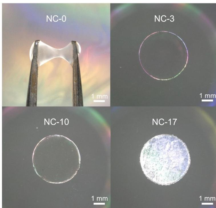
**Figure S1.** Microscopic images of as-prepared NC-*X* hydrogels. NC-0 was unable to be handled due to the minimal amount of chemical crosslinker present. The transparency of the cured NC-PNIPAM decreases with increasing NC concentration.
