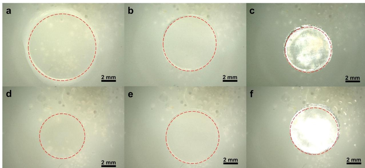
**Figure S3.** Comparison of the transparency of (a) NC-3-S, (b) NC-10-S and (c) NC-17-S samples with (d) NC-3-RS1, (e) NC-10-RS1, and (f) NC-17-RS1, respectively.
