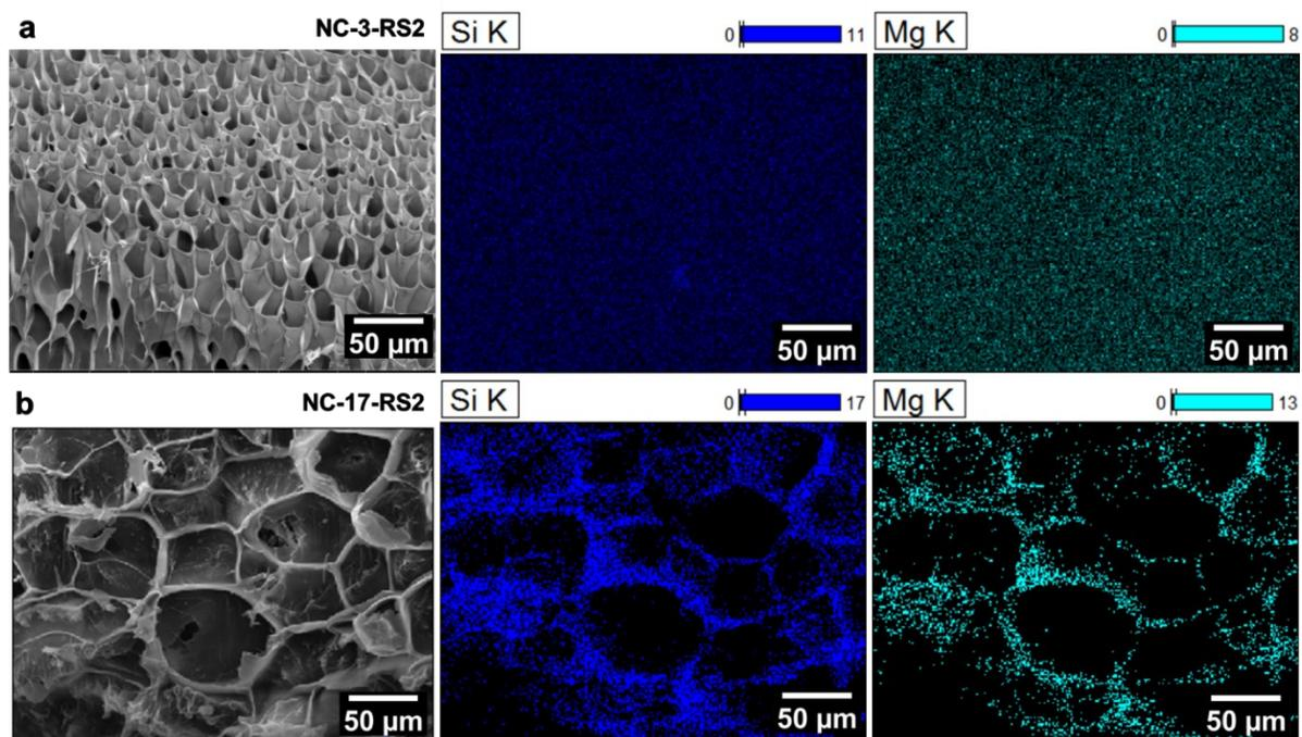
**Figure S6.** SEM images and corresponding EDX images of (a) NC-3-RS2 and (b) NC-17-RS2. The detected elements are Si and Mg.
