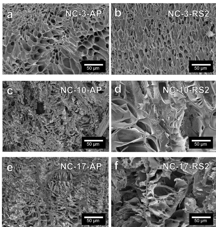
**Figure S5.** SEM images of the as-prepared (AP) states and second reswelled states (RS2) for hydrogels (a, b) NC-3, (c, d) NC-10, and (e, f) NC-17, respectively.
