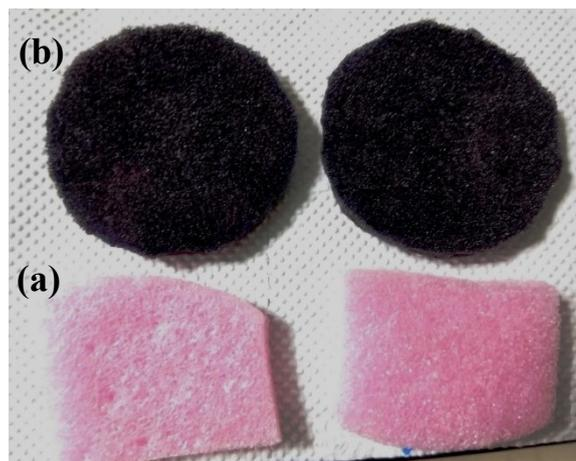
**Figure. S6.** Digital images of (a) commercial PU foams (b) CNT infiltrated PU foams.
