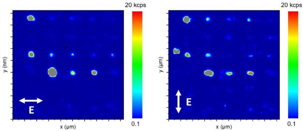
**Figure S4:**  $18 \mu\text{m} \times 18 \mu\text{m}$  PL color maps of 30 assemblies of NDs in the 100 nm gap of Si dimers for an incident laser illumination linearly polarized either parallel (left) or perpendicular (right) to the main axis of the dimers.
