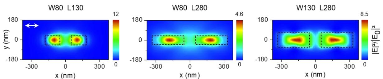
**Figure S3:** Simulated electric field intensity distribution in the xy plane, 15 nm above 3 silicon dimers of different widths  $W$  and lengths  $L$  (both in nanometers) and with a gap  $G = 100$  nm, when illuminated by a plane wave at 520 nm polarized along the dimer long axis. Black, dashed dots indicate the dimer edges.
