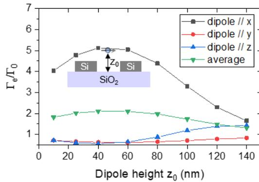
**Figure S5:** Simulated evolution of the normalized decay rate in the gap of a dimer W80 L130 G100 as a function of the height  $z_0$  of an electric dipole emitting at 700 nm, for different dipole orientations. The inset shows a sketch of an electric dipole oriented along  $x$  and located at a height  $z_0$  from the surface, in the gap of a silicon dimer.
