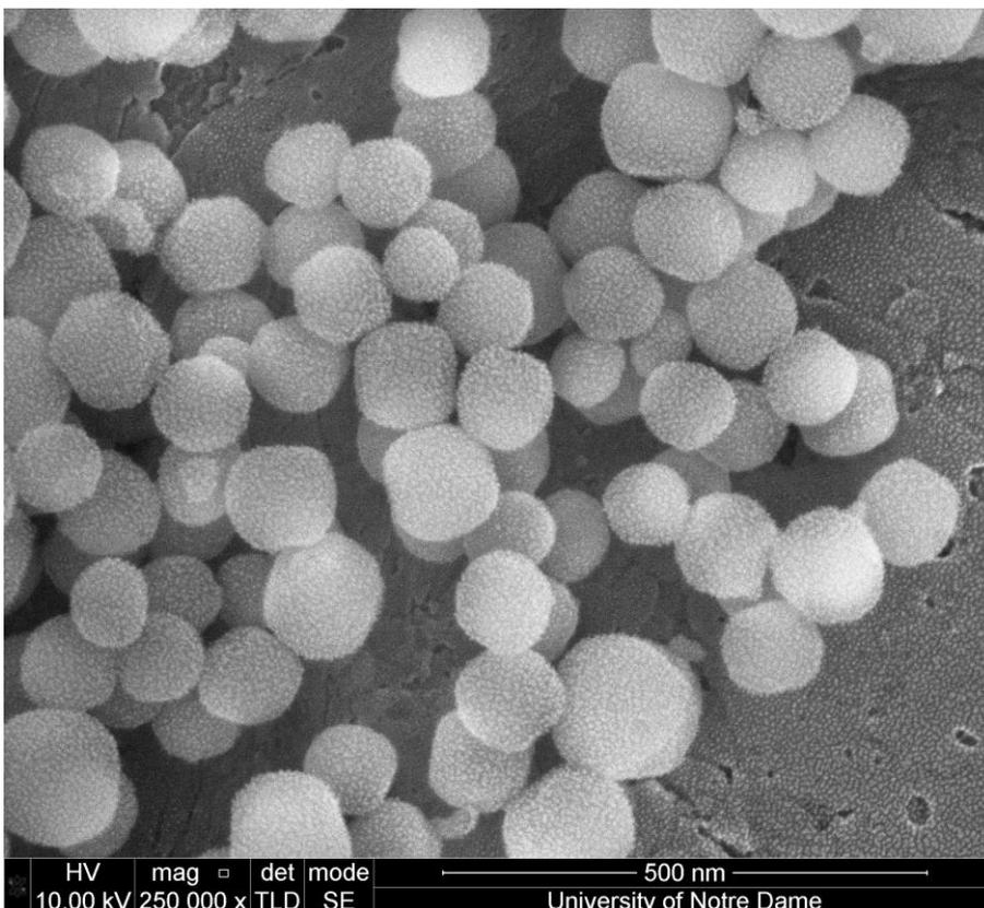
Fig. S2. SEM images of sputtered mesoporous silica nanoparticles (mesoporous SNPs) purchased from Nanocomposix. ~100 nm diameter, pore diameter 3.74 nm (nitrogen adsorption (BET)).
