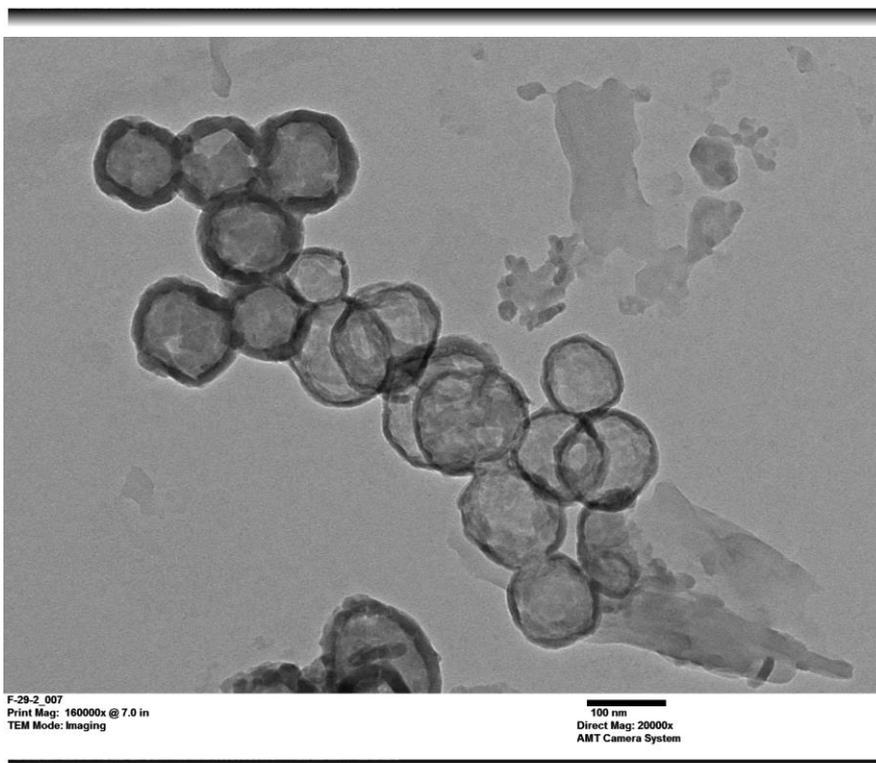
Fig. S11. TEM images. Mesoporous silica nanoparticles (mesoporous SNPs) (200  $\mu$ L, 5 mg/mL in EtOH) were washed with PBS then suspended in PBS (2 mL). Dye S2 (0.4 mg in 50  $\mu$ L DMSO) was added; another 1 mL PBS was used to rinse the tube containing S2 and combined with the reaction mixture. The reaction was stirred at 75 - 80  $^{\circ}$ C in an oil bath for 18 h and at r.t. for another 24 h, then washed with water and stored as a suspension in water ( $\sim$ 1 mg/mL).
