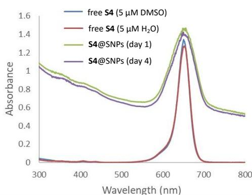
Figure S20. Absorbance spectra for solutions of free S4 (5  $\mu\text{M}$ , DMSO or H<sub>2</sub>O), or hollow SNPs (S4@SNP, 1 mg/mL, H<sub>2</sub>O) that had been created by heating mesoporous SNPs with S4. Spectra of S4@SNP acquired after storage for 1 or 4 days.
