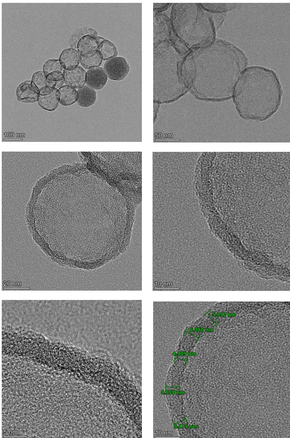
Fig. S13. TEM images. Mesoporous silica nanoparticles (mesoporous SNP) (200  $\mu$ L, 5 mg/mL in EtOH) were washed with PBS then suspended in PBS (2 mL). Mitoxantrone (0.4 mg in 50  $\mu$ L DMSO) was added; another 1 mL PBS was used to rinse the tube containing mitoxantrone and combined with the reaction mixture. The reaction was stirred at 75 - 80  $^{\circ}$ C in an oil bath for 18 h and at r.t. for another 24 h, then washed with water and stored as a suspension in water ( $\sim$ 1 mg/mL).
