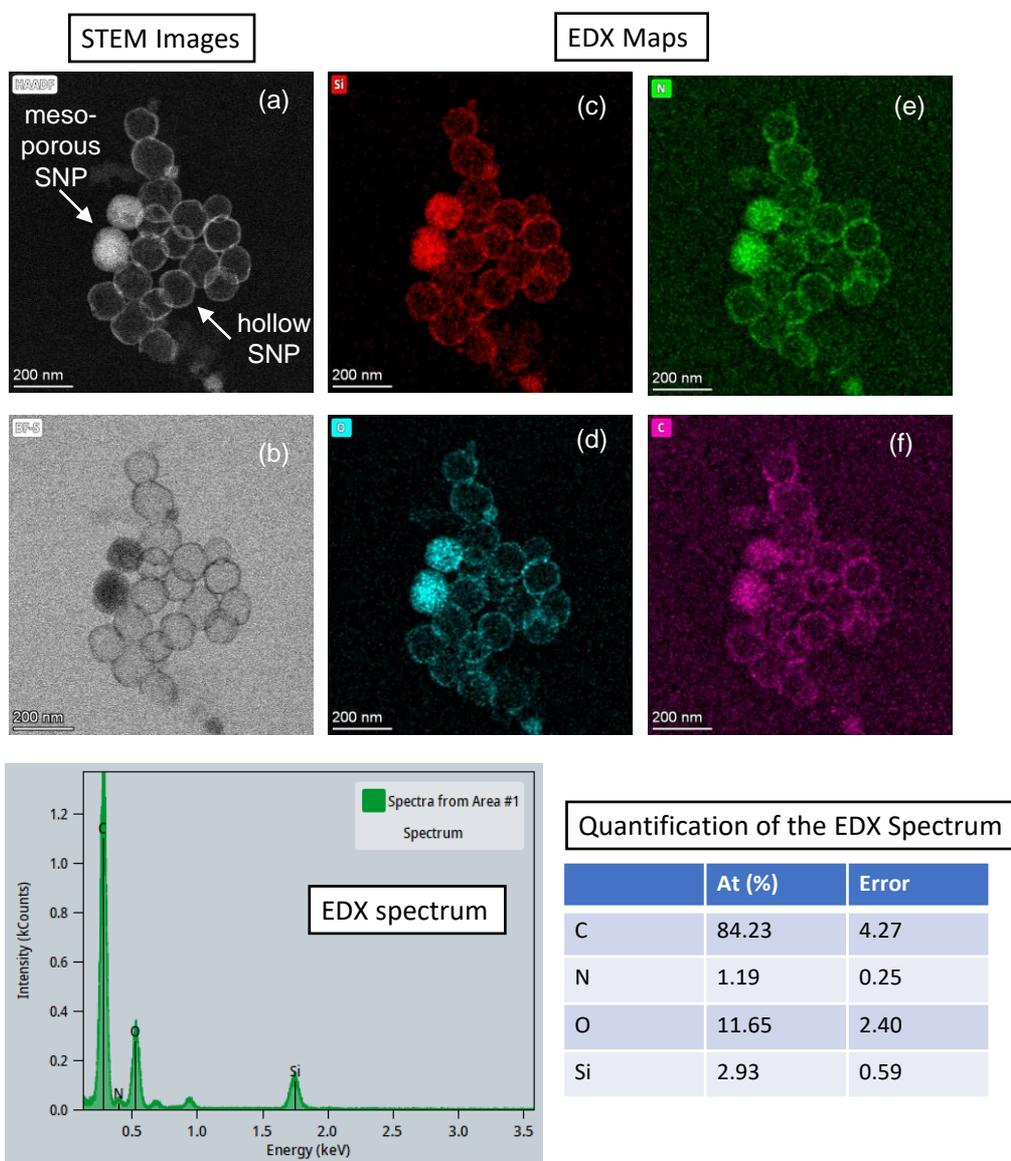
Panels (a-b): **STEM Images** (high angle annular dark field, HAADF and bright field scanning, BFS) of a nanoparticle population comprised of hollow SNPs and two unconverted mesoporous SNPs. Panels (c-f): **EDX Maps** of the image showing distribution of Silicon, Oxygen, Nitrogen, and Carbon. There is also an **EDX Spectrum** and associated table with **Quantification of the EDX Spectrum** for each element in the image.
