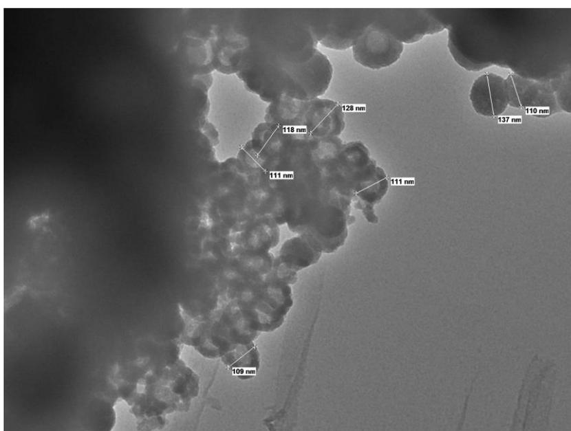
Fig. S19. TEM images. Mesoporous silica nanoparticles (200  $\mu$ L, 5 mg/mL in EtOH) were washed with PBS then suspended in PBS (2 mL). Mitoxantrone (0.4 mg in 50  $\mu$ L DMSO) was added; another 1 mL PBS was used to rinse the tube containing mitoxantrone and combined with the reaction mixture. The reaction was stirred at 75 - 80  $^{\circ}$ C in an oil bath for 48 h, then washed with water and stored as a suspension in water ( $\sim$ 1 mg/mL).
