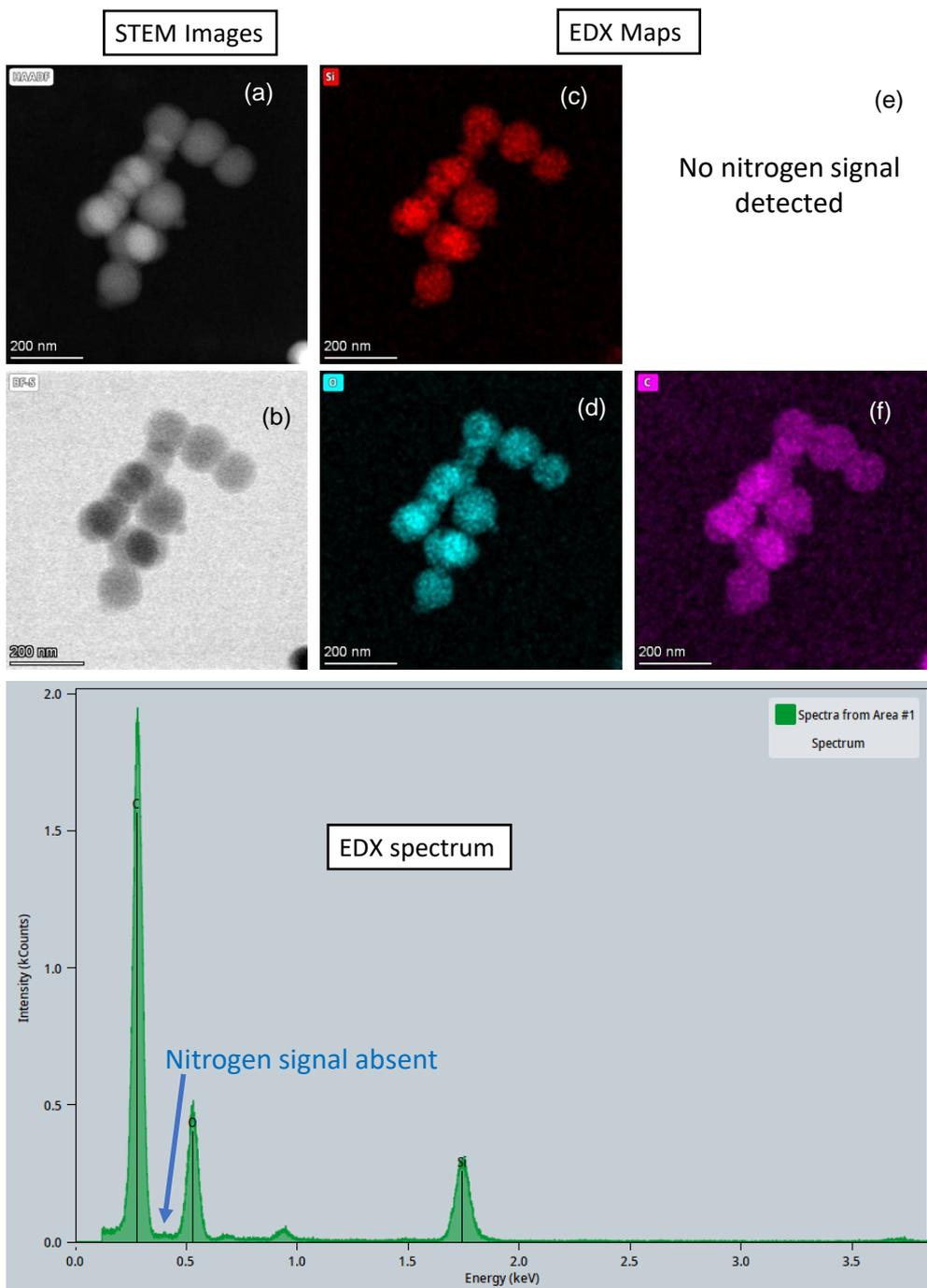
Panels (a-b): **STEM Images** (high angle annular dark field, HAADF and bright field scanning, BFS) of untreated mesoporous SNPs. Panels (c-f): **EDX Maps** of the image showing distribution of Silicon, Oxygen, Nitrogen, and Carbon. There is also an **EDX Spectrum** for each element in the image.
