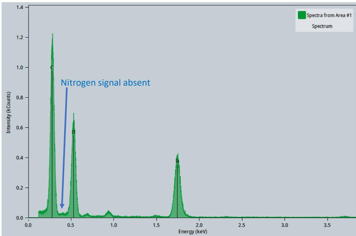
Fig. S18b. EDX spectrum of a separate sample of the mesoporous SNPs described in Figure S18a, all spectra show the same results.
