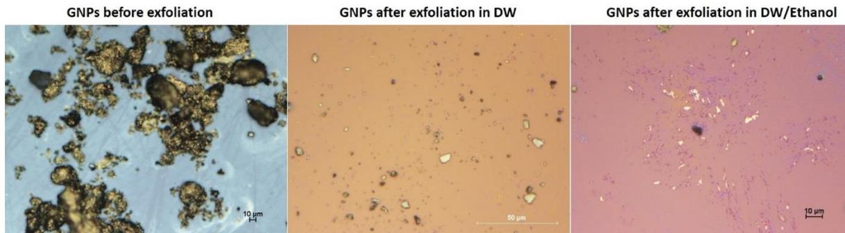
**Figure S2:** From left to right: GNPs before the liquid phase exfoliation, after the exfoliation with distilled water and after the exfoliation with the binary mixture of distilled water/ethanol.
