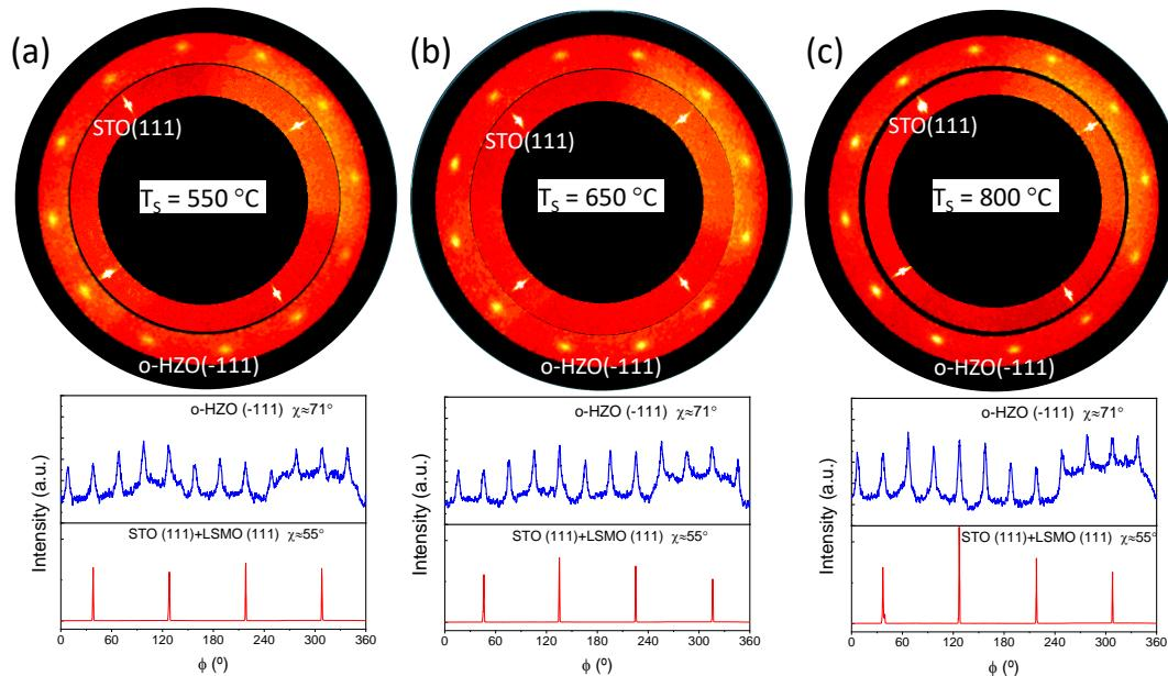
**Figure S2 XRD  $2\theta - \chi$  maps measured with 2D detector**
