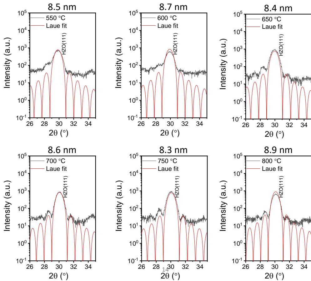
**Figure S4 XRD  $\theta$ - $2\theta$  scans of HZO films deposited on Si(001)**
