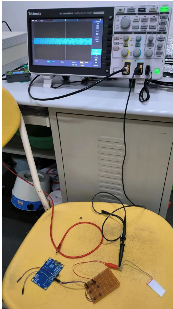
Fig. S 4 The photograph of the oscilloscope detects the power noise.
