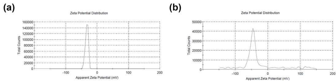
**Figure S5.** Zeta Potentials of (a) ICG and (b) ICGCDs
