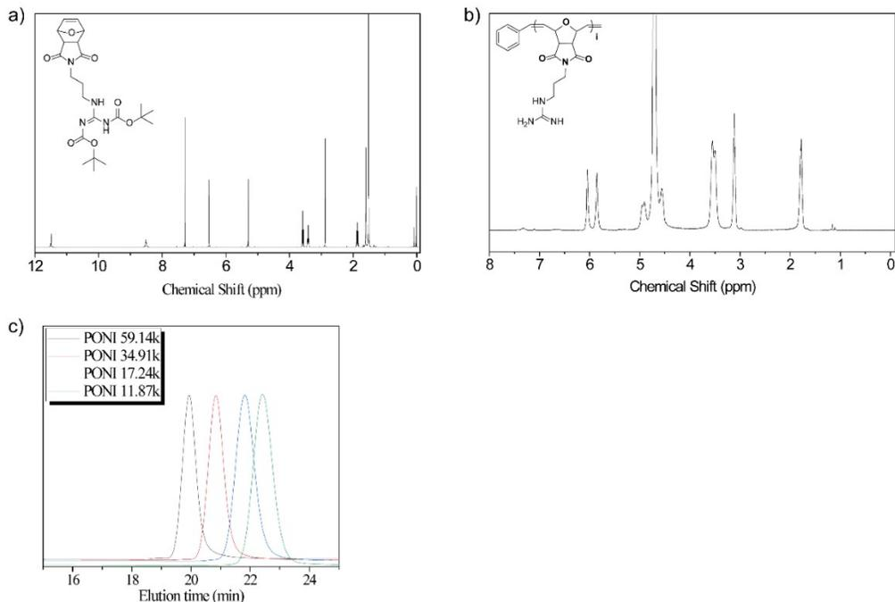
**Figure S2.** (a) Nuclear magnetic resonance (NMR) spectra of compound **5** in CDCl<sub>3</sub> and PONI-Guan polymer in D<sub>2</sub>O. (c) Gel permeation chromatography (GPC) traces of different MW PONI-Guan polymers against PMMA standards.
