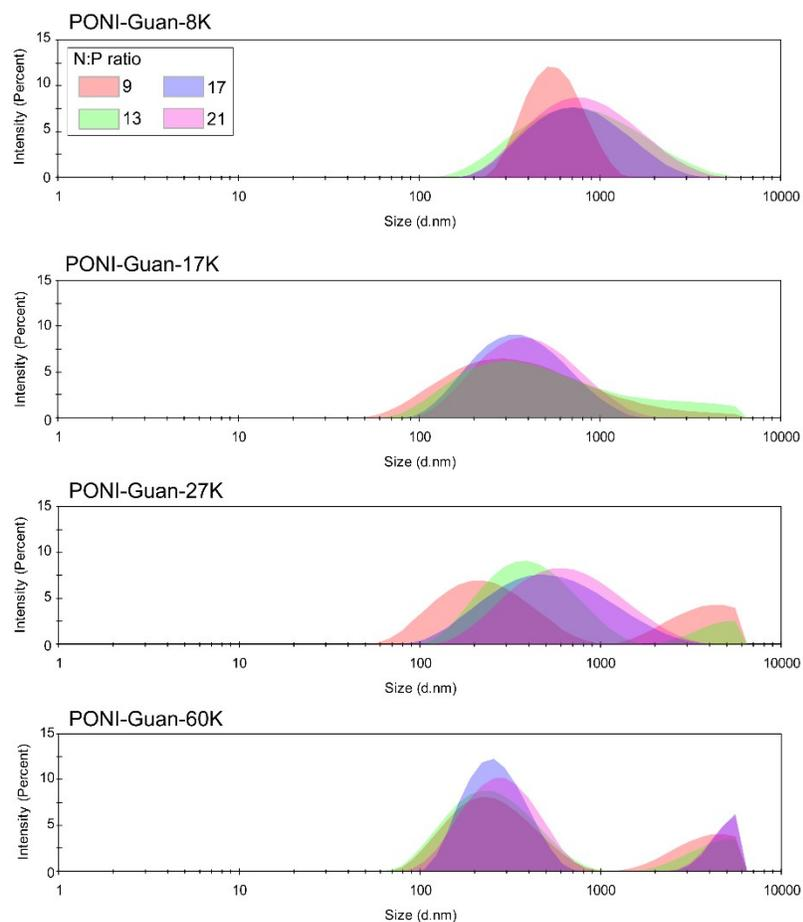
**Figure S4.** Hydrodynamic radius determined by DLS (Intensity). Representative histograms shown for 4 N:P ratio formulations. Key applies to all four spectra.
