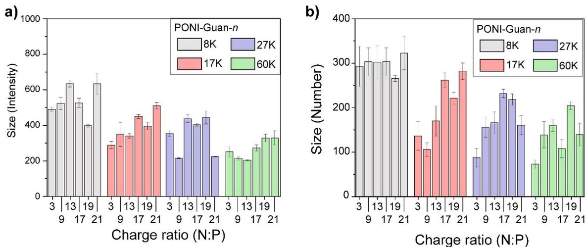
**Figure S3.** Average hydrodynamic radius (nm) of polyplexes measured by DLS, presented by (a) Intensity average and (b) Number average.
