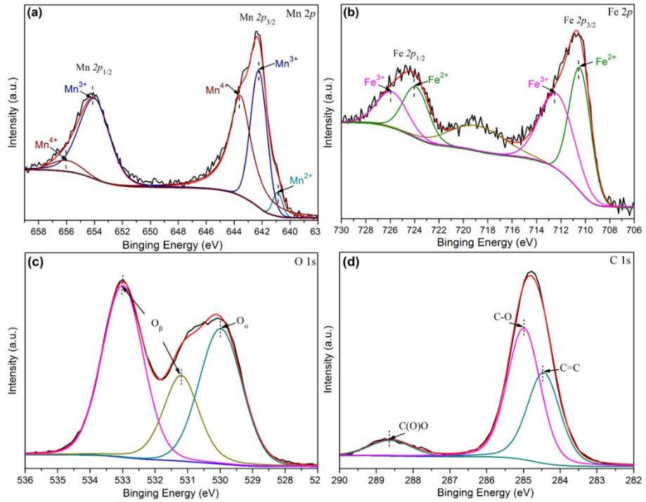
Fig. S5 (a) Mn 2p, (b) Fe 2p, (c) O 1s and (d) C 1s XPS spectra of the Mn<sub>1</sub>Fe<sub>2</sub>-450- used.
