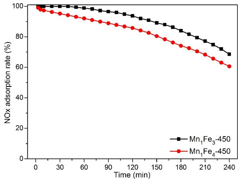
Fig. S1 NO<sub>x</sub> adsorption rate on Mn<sub>1</sub>Fe<sub>3</sub>-450 and Mn<sub>1</sub>Fe<sub>4</sub>-450 at 200 °C.
