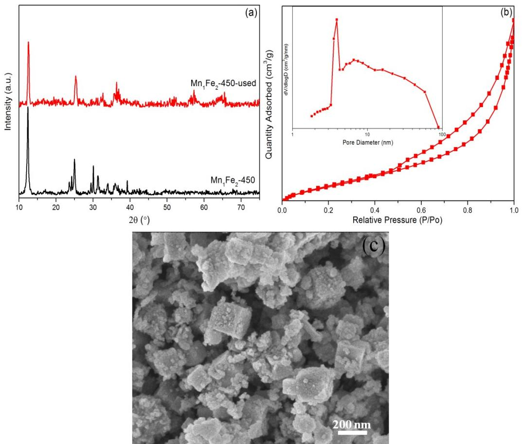
Fig. S4 (a) XRD curve and (b)  $\text{N}_2$  adsorption-desorption isotherms and pore size distribution (inset), and (c) SEM of the  $\text{Mn}_1\text{Fe}_2$ -450-used.
