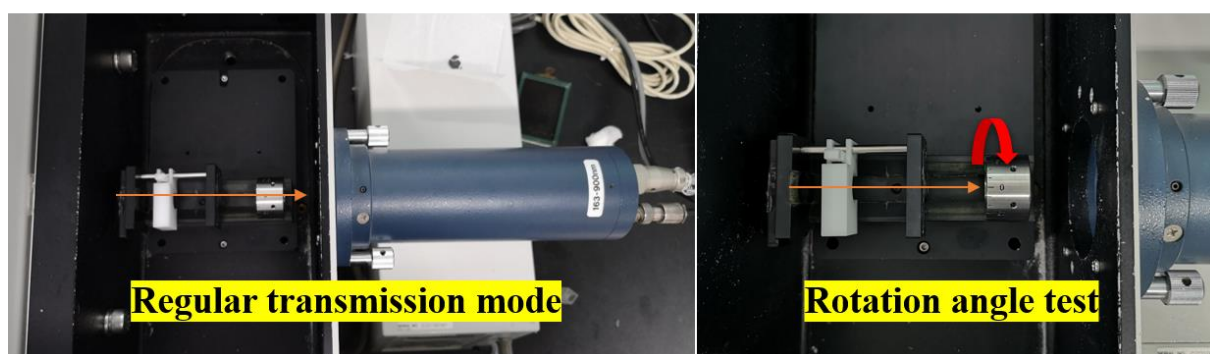
Figure S5. Brief description of infiltration CD method (ICD). In this case, n-decane (a poor solvent for TPU matrix) was added dropwise on the fibrous samples to make them transparent or translucent, and then the infiltrated fibrous samples were adhered closely onto a quartz plate for CD measurement. After the solvent evaporates, the nanofibers return to their original appearance.
