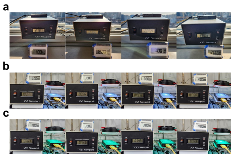
Fig. S10 Measured light intensity using calibrated reference cell depending on time (a) sunlight, (b) white LED and (c) green LED.
