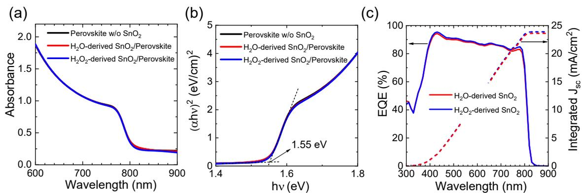
**Figure S2.** (a) Absorbance and (b) Tauc plot of the perovskite films without and with SnO<sub>2</sub> layer (H<sub>2</sub>O-derived and H<sub>2</sub>O<sub>2</sub>-derived SnO<sub>2</sub>). Films were deposited on a glass substrate. (c) External quantum efficiency (EQE) spectra and integrated J<sub>sc</sub> of PSCs based on the H<sub>2</sub>O-derived and H<sub>2</sub>O<sub>2</sub>-derived SnO<sub>2</sub>.
