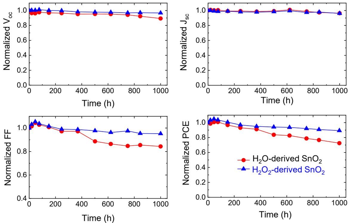
**Figure S6.** Storage stability showing normalized photovoltaic parameters of  $V_{oc}$ ,  $J_{sc}$ , FF and PCE of PSCs based on the H<sub>2</sub>O- and H<sub>2</sub>O<sub>2</sub>-derived SnO<sub>2</sub>, measured for 1000 h under relative humidity of 30±10% at room temperature.
