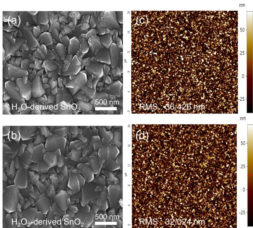
**Figure S1.** Top-view SEM images of (a) the H<sub>2</sub>O-derived SnO<sub>2</sub> and (b) the H<sub>2</sub>O<sub>2</sub>-derived SnO<sub>2</sub> on the FTO substrate. AFM images of (c) the H<sub>2</sub>O-derived SnO<sub>2</sub> and (d) the H<sub>2</sub>O<sub>2</sub>-derived SnO<sub>2</sub> on the FTO substrate. RMS is root mean square.
