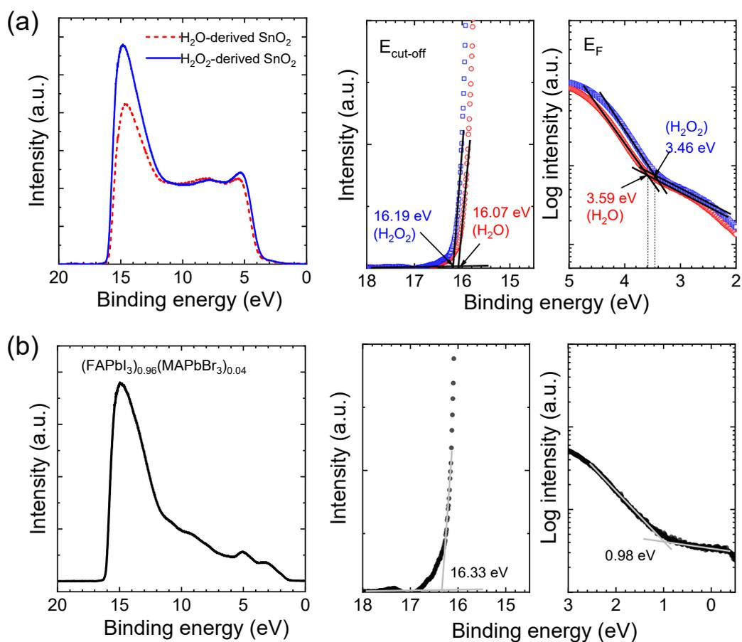
**Figure S3.** UPS spectra of (a) ALD-processed SnO<sub>2</sub> depending on oxygen source of H<sub>2</sub>O and H<sub>2</sub>O<sub>2</sub> and (b) (FAPbI<sub>3</sub>)<sub>0.96</sub>(MAPbBr<sub>3</sub>)<sub>0.04</sub> perovskite, showing the full range (left panel), the cut-off energy (middle panel) and Fermi edge (middle panel).
