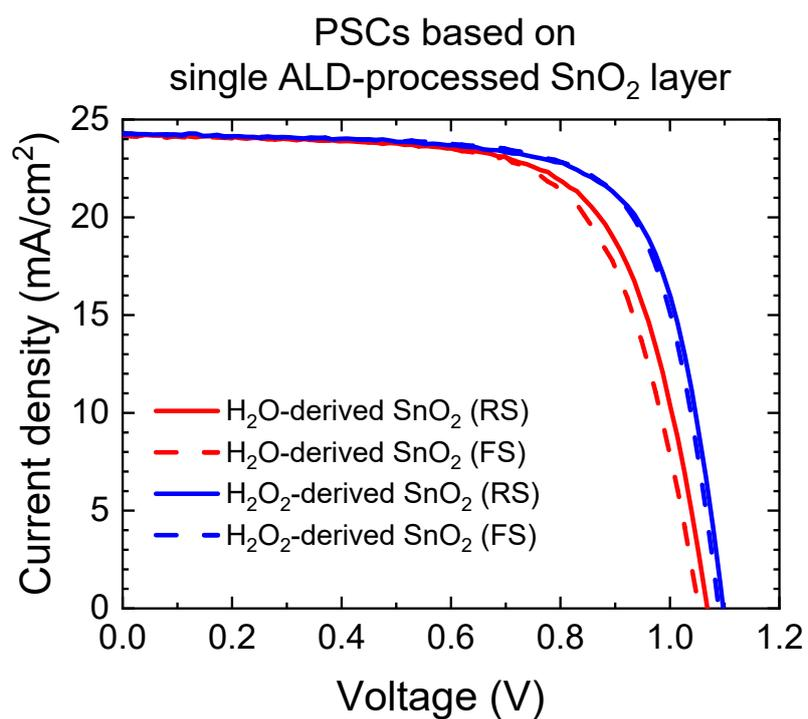
**Figure S5.** J-V curves of PSCs based on a single ALD-processed SnO<sub>2</sub> layer depending on oxygen source of H<sub>2</sub>O and H<sub>2</sub>O<sub>2</sub>. FS (dashed lines) and RS (solid lines) represent the forward and reverse scanned data, respectively.
