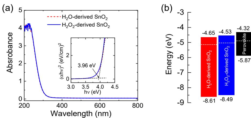
**Figure S4.** (a) UV-Vis spectra of the ALD-processed SnO<sub>2</sub> films deposited on a glass substrate. Inset shows Tauc plot. (b) Energy level diagram of the H<sub>2</sub>O-derived SnO<sub>2</sub>, H<sub>2</sub>O<sub>2</sub>-derived SnO<sub>2</sub>, and perovskite layer based on the data obtained from UPS and UV-Vis spectroscopy.
