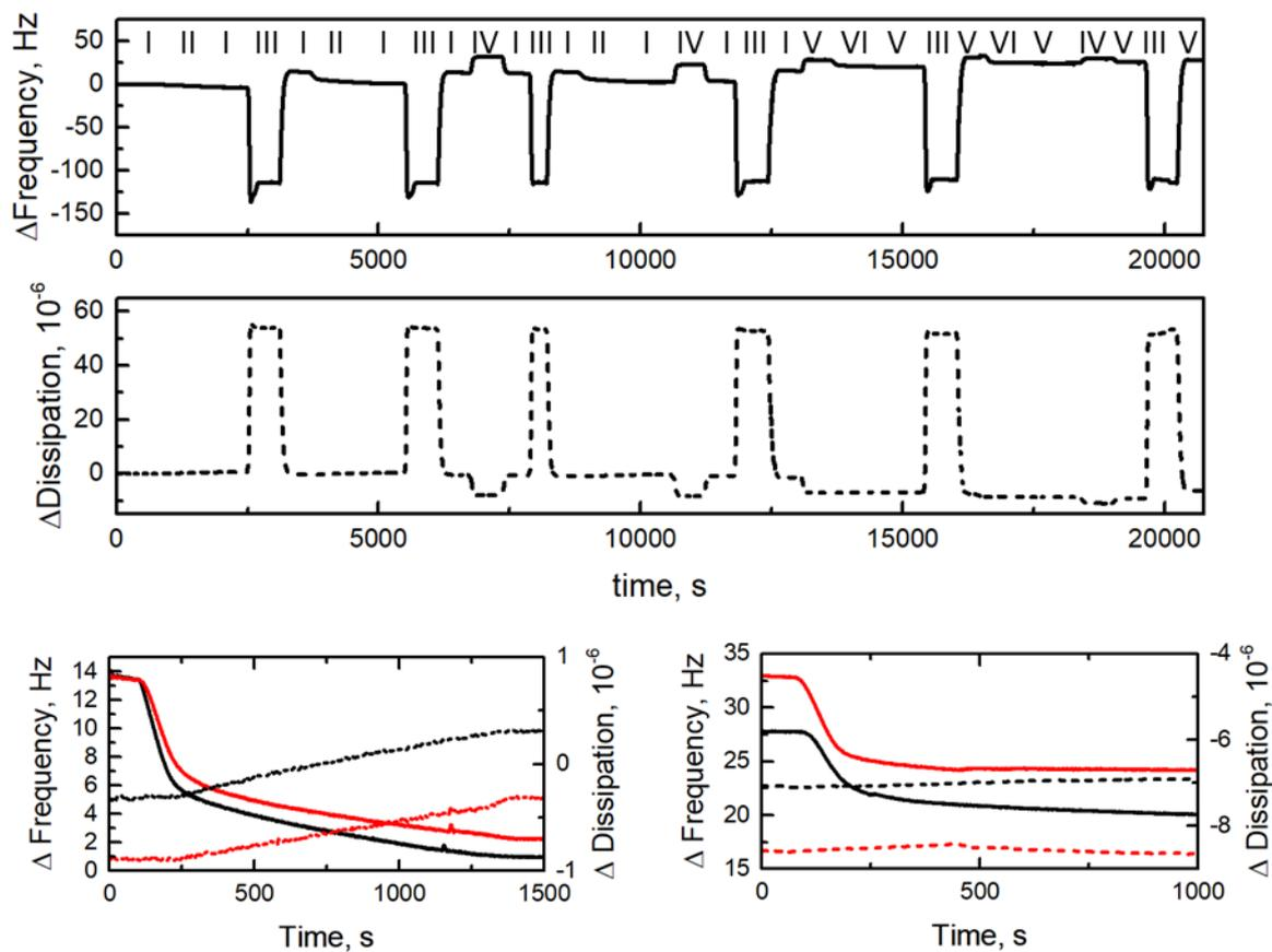
Figure S1.7. QCM-D sensorgrams of SUV solution injection on the **EG<sub>6</sub>AC<sub>8</sub>D** tethered substrate, i.e.  $\chi_{\text{EG}_6\text{AC}_8\text{D}}=100$  mol %. The injection sequence is marked in Roman numerals above the frequency sensorgram and described above. The overlays of vesicle injection at the positive (SUVs in hypertonic buffer) and neutral (isotonic solution) osmotic pressure are presented in the bottom left and bottom right panels, respectively.
