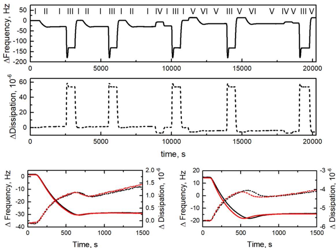
Figure S1.5. QCM-D sensorgrams of SUV solution injection on the **EG<sub>6</sub>AC<sub>8</sub>D** tethered substrate, i.e.  $\chi_{\text{EG}_6\text{AC}_8\text{D}} = (18.1 \pm 2.9) \text{ mol } \%$ . The injection sequence is marked in Roman numerals above the frequency sensorgram and described above. The overlays of vesicle injection at the positive (SUVs in hypertonic buffer) and neutral (isotonic solution) osmotic pressure are presented in the bottom left and bottom right panels, respectively.
