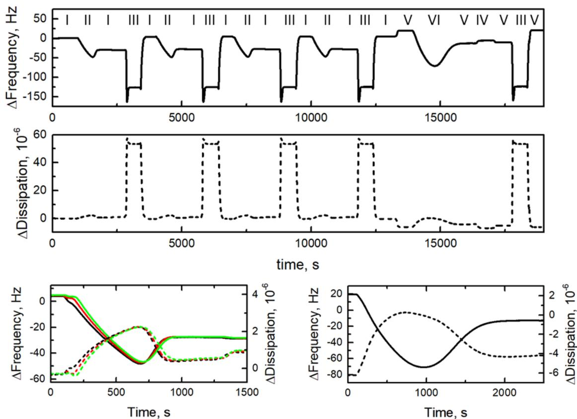
Figure S1.10. QCM-D sensorgrams of SUV solution injection on the  $\text{EG}_6\text{AC}_{16}\text{D}$  tethered substrate, i.e.  $\chi_{\text{EG}_6\text{AC}_{16}\text{D}} = 5.6 \pm 3.6$  mol %. The injection sequence is marked in Roman numerals above the frequency sensorgram and described above. The overlays of vesicle injection at the positive (SUVs in hypertonic buffer) and neutral (isotonic solution) osmotic pressure are presented in the bottom left and bottom right panels, respectively.
