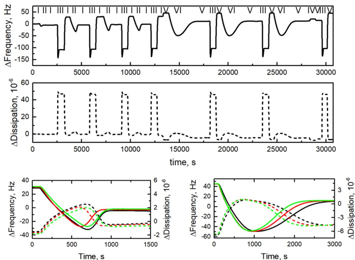
Figure S1.8. QCM-D sensorgrams of SUV solution injection on the  $\text{EG}_6\text{AC}_{16}\text{D}$  tethered substrate, i.e.  $\chi_{\text{EG}_6\text{AC}_{16}\text{D}} = 2.9 \pm 2.1$  mol %. The injection sequence is marked in Roman numerals above the frequency sensorgram and described above. The overlays of vesicle injection at the positive (SUVs in hypertonic buffer) and neutral (isotonic solution) osmotic pressure are presented in the bottom left and bottom right panels, respectively.
