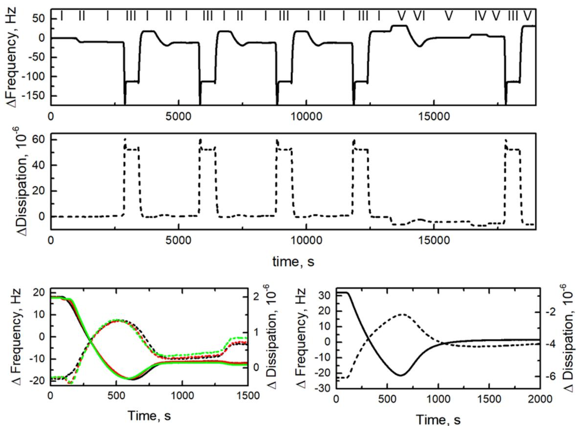
Figure S1.4. QCM-D sensorgrams of SUV solution injection on the **EG<sub>6</sub>AC<sub>8</sub>D** tethered substrate, i.e.  $\chi_{\text{EG}_6\text{AC}_8\text{D}} = (13.3 \pm 2.0) \text{ mol } \%$ . The injection sequence is marked in Roman numerals above the frequency sensorgram and described above. The overlays of vesicle injection at the positive (SUVs in hypertonic buffer) and neutral (isotonic solution) osmotic pressure are presented in the bottom left and bottom right panels, respectively.
