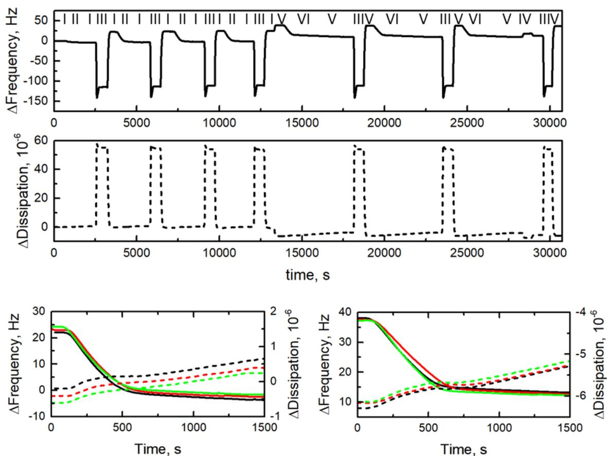
Figure S1.12. QCM-D sensorgrams of SUV solution injection on the **EG<sub>6</sub>AC<sub>16</sub>D** tethered substrate, i.e.  $\chi_{\text{EG}_6\text{AC}_{16}\text{D}} = 10.0 \pm 3.0$  mol %. The injection sequence is marked in Roman numerals above the frequency sensorgram and described above. The overlays of vesicle injection at the positive (SUVs in hypertonic buffer) and neutral (isotonic solution) osmotic pressure are presented in the bottom left and bottom right panels, respectively.
