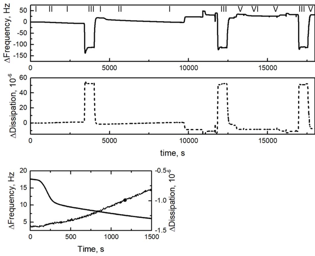
Figure S1.13. QCM-D sensorgrams of SUV solution injection on the **EG<sub>6</sub>AC<sub>16</sub>D** tethered substrate, i.e.  $\chi_{\text{EG}_6\text{AC}_{16}\text{D}}=100 \text{ mol } \%$ . The injection sequence is marked in Roman numerals above the frequency sensorgram and described above. The overlays of vesicle injection at the positive (SUVs in hypertonic buffer) in the bottom left panel, respectively.
