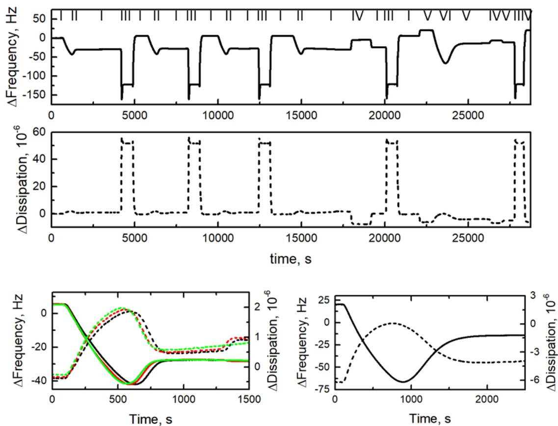
Figure S1.9. QCM-D sensorgrams of SUV solution injection on the **EG<sub>6</sub>AC<sub>16</sub>D** tethered substrate, i.e.  $\chi_{\text{EG}_6\text{AC}_{16}\text{D}} = 3.5 \pm 2.1$  mol %. The injection sequence is marked in Roman numerals above the frequency sensorgram and described above. The overlays of vesicle injection at the positive (SUVs in hypertonic buffer) and neutral (isotonic solution) osmotic pressure are presented in the bottom left and bottom right panels, respectively.
