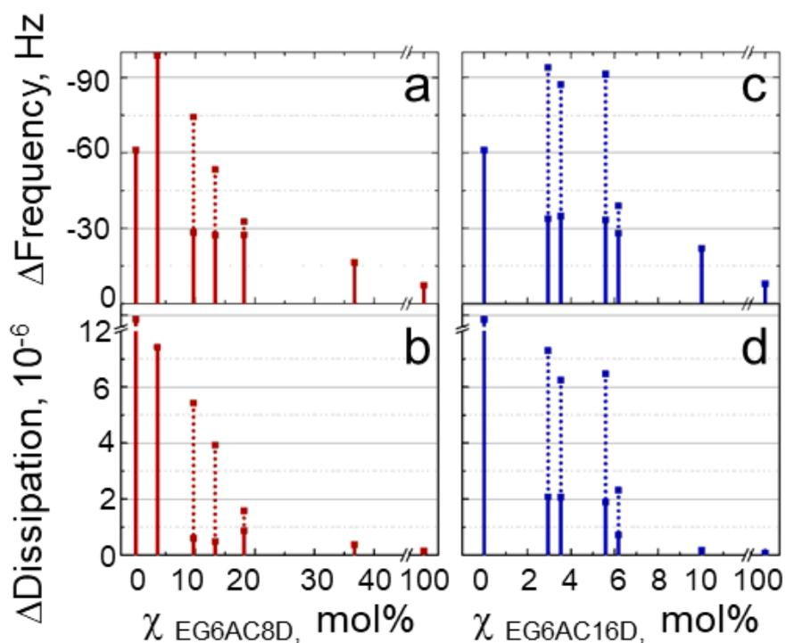
Figure S3. Analysis of lipid tBLM formation at neutral osmotic pressure (isotonic solution) conditions on the EG<sub>6</sub>AC<sub>8</sub>D (red) and EG<sub>6</sub>AC<sub>16</sub>D (blue) tethered surfaces, respectively. The frequency (a, c) and dissipation (b, d) signal amplitude (dotted line), and equilibrium (solid line) values are plotted as function of the tether surface molar density.
