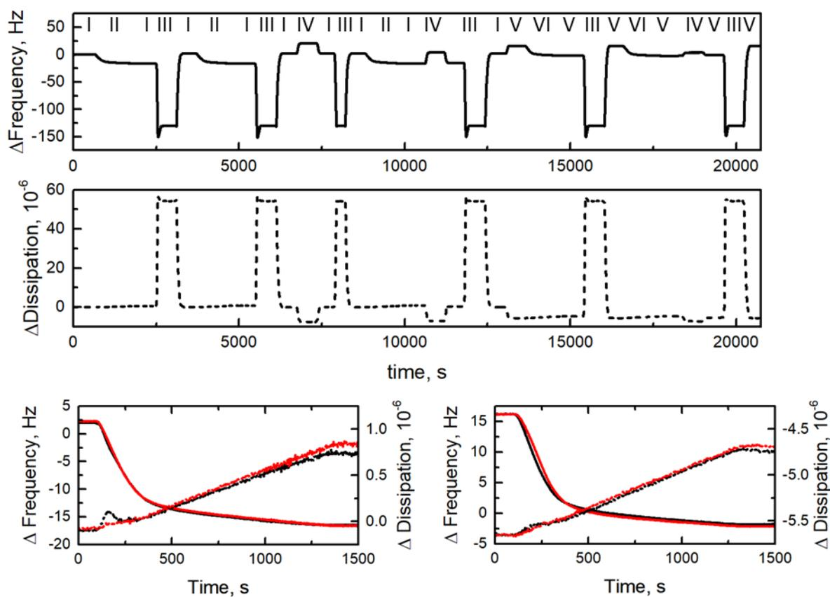
Figure S1.6. QCM-D sensorgrams of SUV solution injection on the **EG<sub>6</sub>AC<sub>8</sub>D** tethered substrate, i.e.  $\chi_{\text{EG}_6\text{AC}_8\text{D}} = (36.7 \pm 3.3) \text{ mol } \%$ . The injection sequence is marked in Roman numerals above the frequency sensorgram and described above. The overlays of vesicle injection at the positive (SUVs in hypertonic buffer) and neutral (isotonic solution) osmotic pressure are presented in the bottom left and bottom right panels, respectively.
