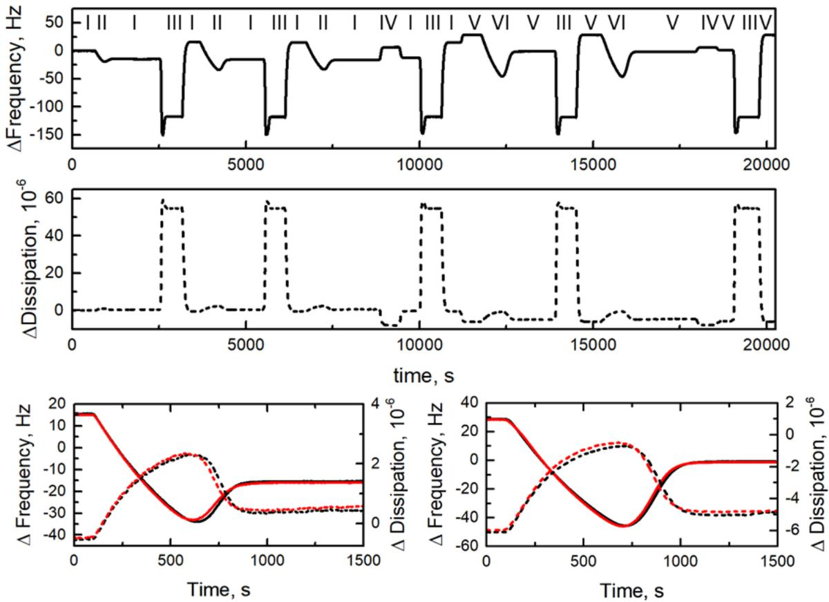
Figure S1.3. QCM-D sensorgrams of SUV solution injection on the **EG<sub>6</sub>AC<sub>8</sub>D** tethered substrate, i.e.  $\chi_{\text{EG}_6\text{AC}_8\text{D}} = (9.7 \pm 2.4)$  mol %. The injection sequence is marked in Roman numerals above the frequency sensorgram and described above. The overlays of vesicle injection at the positive (SUVs in hypertonic buffer) and neutral (isotonic solution) osmotic pressure are presented in the bottom left and bottom right panels, respectively.
