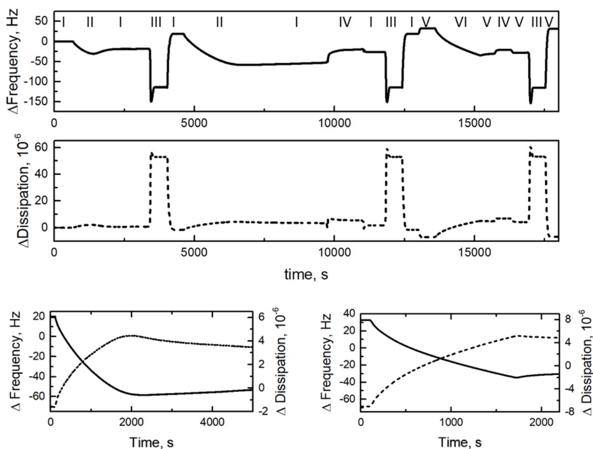
Figure S1.1. QCM-D sensorgrams of SUV solution injection on the tetherless **EG<sub>1</sub>H** substrate, i.e.. The injection sequence is marked in roman numerals above the frequency curve. The overlays of vesicle injection at the positive (SUVs in hypertonic buffer) and neutral (isotonic solution) osmotic pressure are presented in the bottom left and bottom right panels, respectively. Note the increase in dissipation upon injection of deionized water (injection IV).
