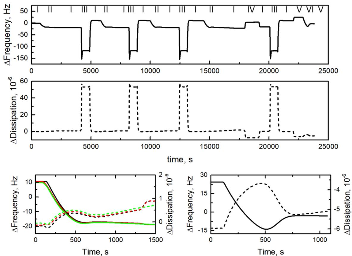
Figure S1.11. QCM-D sensorgrams of SUV solution injection on the **EG<sub>6</sub>AC<sub>16</sub>D** tethered substrate, i.e.  $\chi_{\text{EG}_6\text{AC}_{16}\text{D}} = 6.2 \pm 2.1$  mol %. The injection sequence is marked in Roman numerals above the frequency sensorgram and described above. The overlays of vesicle injection at the positive (SUVs in hypertonic buffer) and neutral (isotonic solution) osmotic pressure are presented in the bottom left and bottom right panels, respectively.
