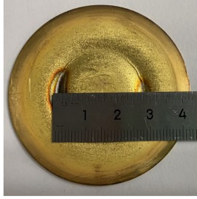
Fig. S2 A photograph of a gold target was used frequently on the magnetron sputter. It was found that the gold target exhibits an etching ring.
