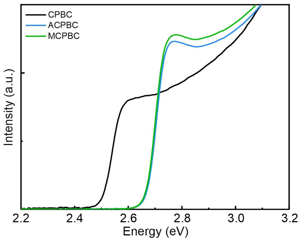
**Figure S7.** The bandgap curves of CPBC, ACPBC and MCPBC QDs, which are obtained from the absorption curves.
