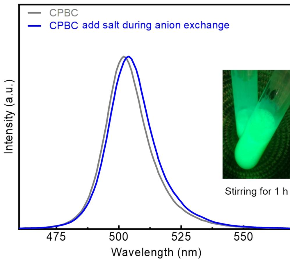
**Figure S2.** The PL spectra of CPB QDs without and with Al-salt added during anion exchange. The ratio of Al/Pb and the amount of DDAC is fixed as 1:1 and 0.1 mmol.
