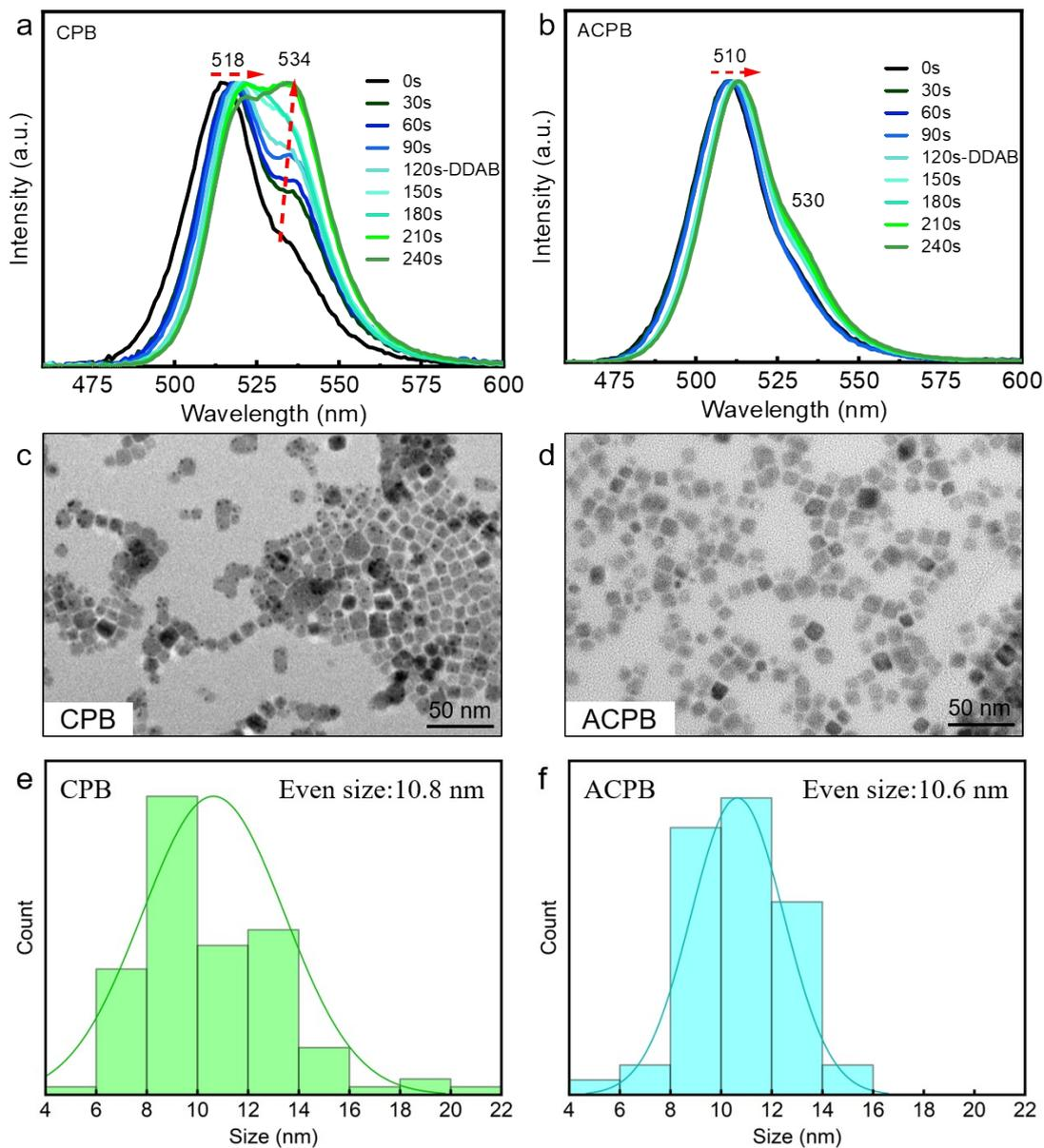
**Figure S4.** The in-situ PL spectra of CPB (a) and ACPB (b) QDs. the Cs-precursor is injected to Pb-precursor at 0 s, and DDAB solution is injected at 120 s. c. and d. The TEM graphs of CPB and ACPB QDs. e. and f. The size distribution of CPB and ACPB QDs, the later indicates a more uniform distribution, while there are individual large grains for the former.
