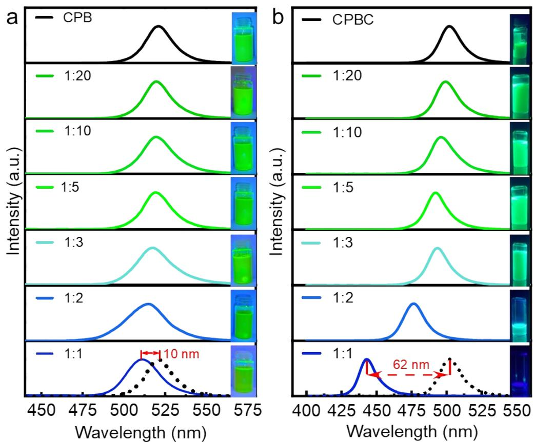
**Figure S1.** The spectra of CPB, CPBC, ACPB and ACPBC QDs. **a.** The PL spectra of crude solutions (CPB, the ratio of Al:Pb changes from 1:20 to 1:1). The illustrations demonstrate samples under ultraviolet (UV) light. **b.** The PL comparison of CPBC and ACPBC QDs (ratio of Al:Pb vary from 1:20 to 1:1). Inserts demonstrate the solutions after anion exchange.
