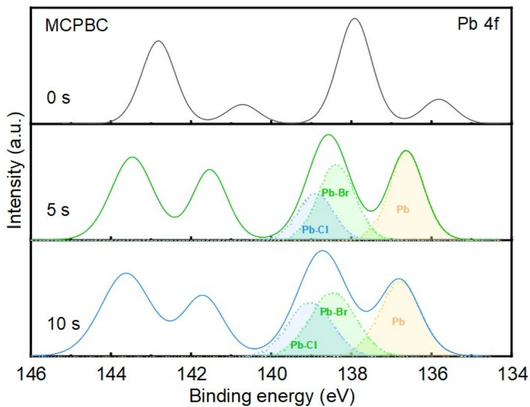
**Figure S5.** The XPS data of Pb in MCPBC QDs, the gray, green and blue respectively represent etching for 0, 5 and 10 s. There has a more obvious peak attribute to Pb<sup>0</sup> than that of CPBC and ACPBC (Figure S3c), demonstrating weaker stability of lattice structure.
