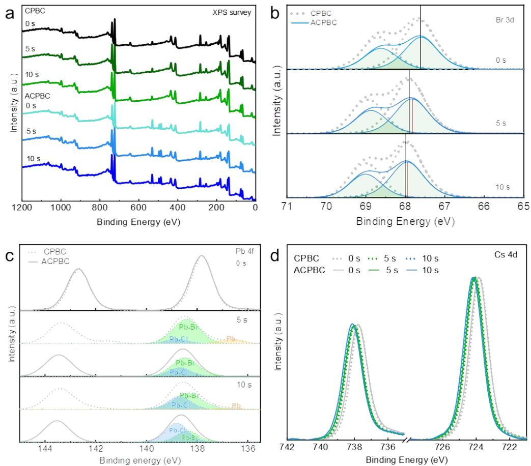
**Figure S3.** XPS spectra of CPBC and ACPBC QDs. **a.** The survey spectra of CPBC and ACPBC QDs under etching for 0s, 5s and 10s. **b.** The Br XPS spectra of CPBC and ACPBC QDs, the binding energy shift to higher level. **c.** The Pb XPS spectra of CPBC and ACPBC QDs. The peaks of Pb-Br and Pb-Cl can split two characteristic peaks (shaded area). **d.** The Cs XPS spectra of CPBC and ACPBC QDs under etching for 0s, 5s and 10s, the binding energies of two sample are approximate.
